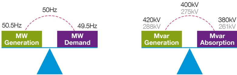
When active power (MW) generation is greater than active power demand, the frequency increases, and when active power generation is lower than active power demand the frequency decreases. Similarly, when Reactive Power (Mvar) generation is greater than Reactive Power absorption, the voltage increases, and when Reactive Power generation is lower than Reactive Power absorption the voltage decreases. However, unlike active power for
