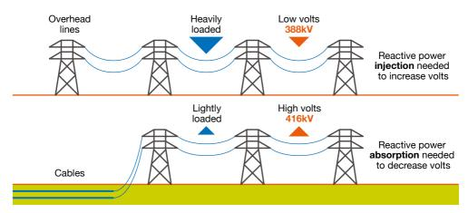
Reactive power differs from active power because it is a locational requirement. Reactive power is only effective for voltage control if it is provided close to the area where the voltage needs to change. It becomes less effective with distance.
