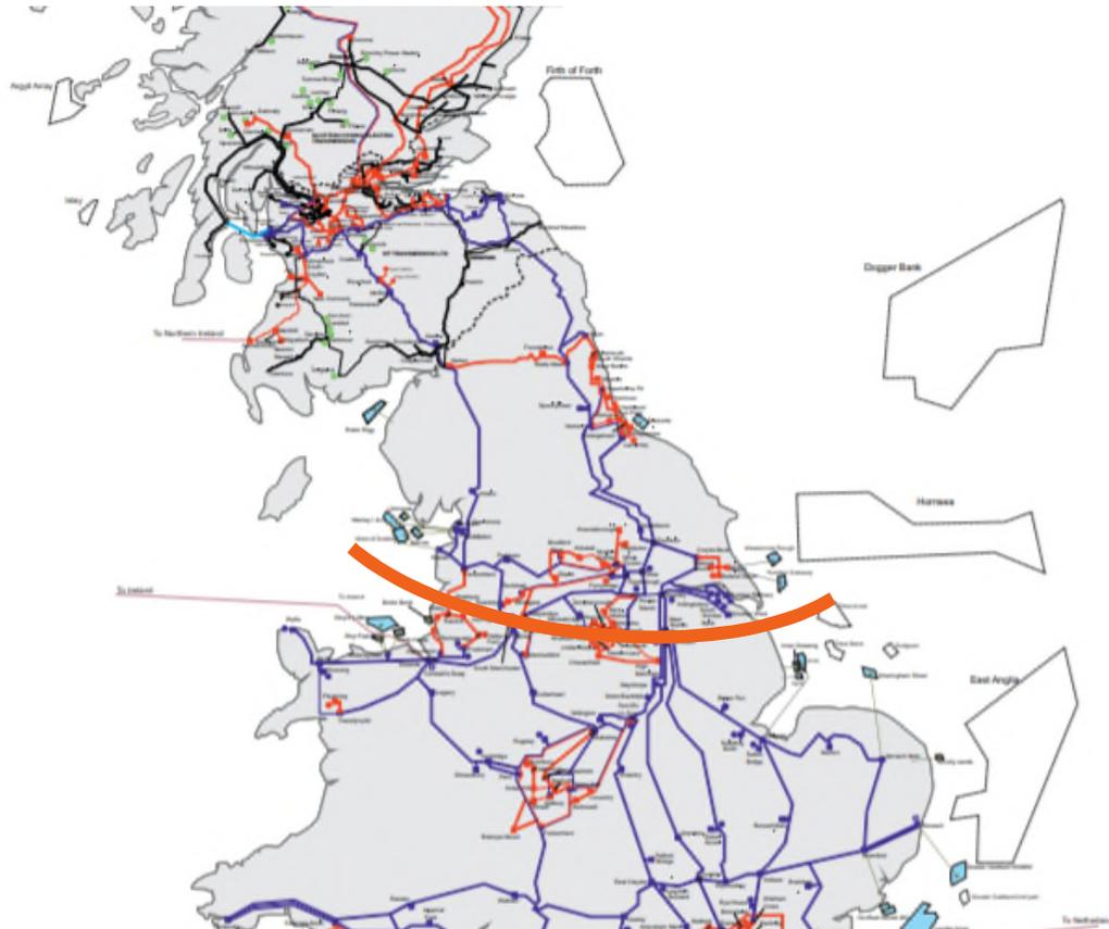
Constraint boundary driven by year ahead planned outage on West coast. This outage could not be recalled.
