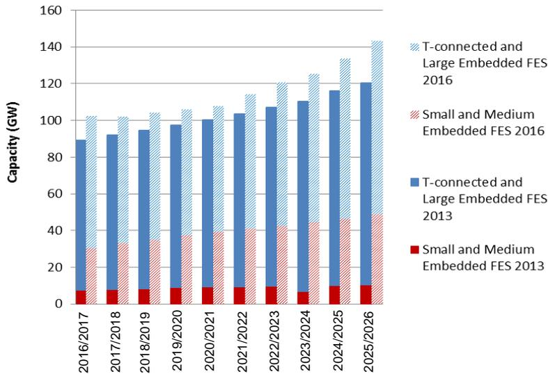
Figure 2: GB electricity supply capacity in different generation types forecasted under Gone Green Scenario according to FES 2013 and FES 2016.
