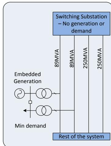
Figure 23. Local boundary issues that may be caused due to generation constrain
