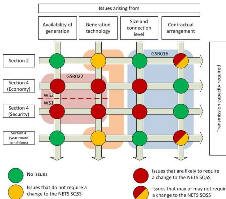
Figure 1: Issues and interactions when applying NETS SQSS due to increasing level of small and medium EG
