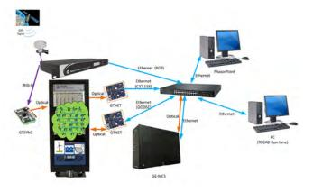
Figure 5: RTDS-HiL testbed and communication setup
