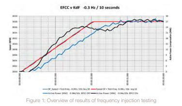
Although the test results were generally considered successful, the interaction between conventional frequency response (KdF) and RoCoF-based frequency response is very important to all concerned. Although the revised frequency control logic is not being used in a live environment, Centrica is able to analyse how it would respond to actual power system events using the CCGT module's DEPP system – a fast data recorder with a resolution down to 40ms.
