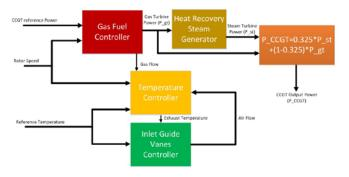
Figure 3: CCGT block diagram model
