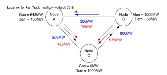
Therefore, circuits AB and BC are tagged as Peak Security and AC is tagged as Year Round.
