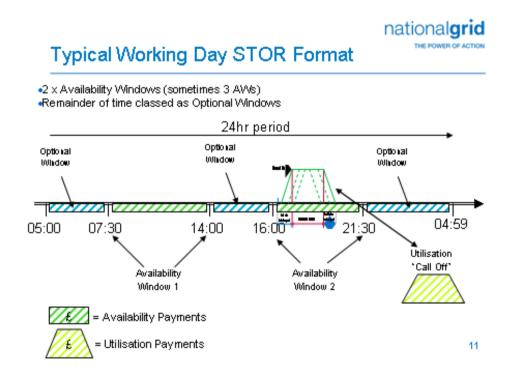
In addition, where delivery of Contracted MW is up to the end, or close to the end, of the Availability Window, there may be energy delivered outside the Window whilst the unit/site is returning to its default state. These are called preand post-window phases and are expressly defined under the service:
