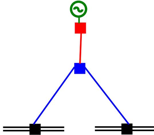
Example 3 shows a generation substation connecting to a second substation via a single circuit which is further connected to two different MITS substations. In this case, only the generation substation and the circuit connecting this to the second substation form a single radial spur used only for connecting generation to the MITS. The second substation and both the local circuits connecting this to the MITS substations do not form part of the spur as these parallel the MITS.
