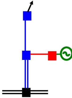
This example shows a radial circuit that facilitates both generation and demand. The separate demand and generation substations connect via to a substation via a single circuit which in turn connects to a single MITS substation via a double circuit. In this scenario the generation substation and the single circuit connecting to the intermediary substation form a radial spur used only for connecting generation to the MITS.
