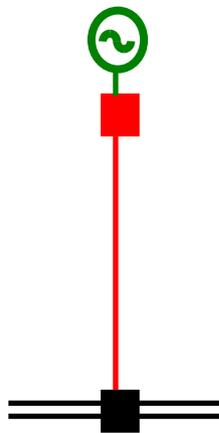
This example shows the simplest example of a single radial spur used only for connecting generation to the MITS, in the form of a single circuit. The circuit does not parallel the MITS, as it connects to a single MITS substation.
