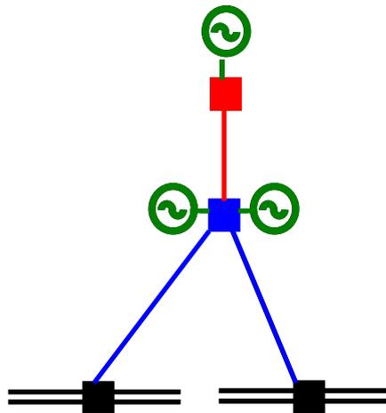
This example is identical to Example 3 with the exception that generation connects to the second substation. This makes no difference to the assets that form a radial spur used only for connecting generation to the MITS.
