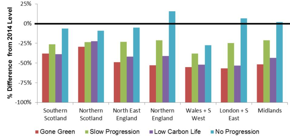
Figure 21 Minimum Short Circuit Level Relative to 2014/15 Level(2024/25)
