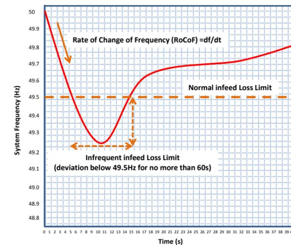
Figure 14 Impact of High RoCoF on Frequency Containment
