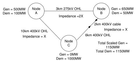
Step 2:Net export from Node B to Node C is 1000MW; route BC has impedance X and route
