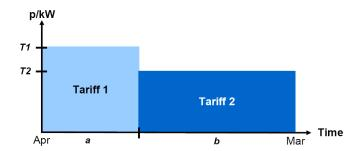
14.17.8 If multiple sets of energy tariffs are applicable within a single charging year, energy charges will be calculated by multiplying relevant Tariffs by the Chargeable Energy Capacity over the period that that the tariffs are applicable for and summing over the year.
