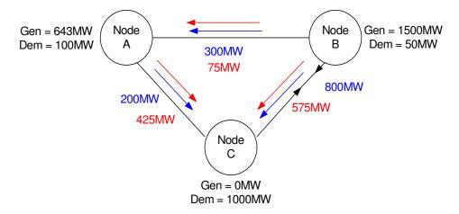
Therefore, circuits AB and BC are tagged as Peak Security and AC is tagged as Year Round.
