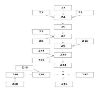
The arrows connecting generation charging zones and amalgamated generation charging zones represent the incremental km transmission boundary lengths towards the notional centre of the system. Generation located in zones behind arrows is considered to share based on the ratio of Low Carbon to Carbon cumulative generation TEC within those zones.
