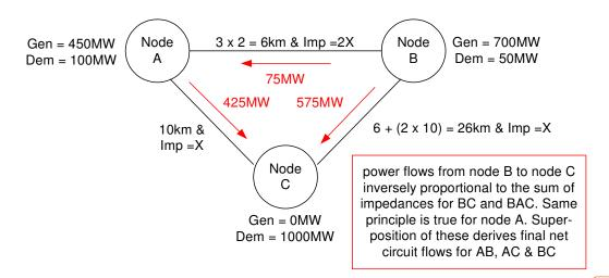
Nodes A and B export, whilst Node C imports. Hence the DCLF algorithm derives flows to deliver export power from Nodes A and B to meet import needs at Node C.
