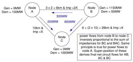
Node B exports, whilst Nodes A and C import. Hence the DCLF algorithm derives flows to deliver export power from Node B to meet import needs at Nodes A and C.
