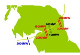
The adjacent diagram shows the circuits on the B6 constraint boundary and their capacities. The total capacity of the B6 is 10,000MW, 2,000MW of which relates to the HVDC link (shown in blue). As the HVDC link makes up 20% of the B6 boundary capacity, the desired B6 boundary flow on the HVDC link will be 1,200MW (20% of the B6 base boundary flow (6000MW)).
