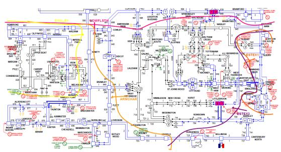
159. During periods of high output from Thames Estuary generation with exports or low imports on the IFA the loss of a double circuit route from the Thames Estuary will result in unacceptable loading of the remaining circuits. Imports from Netherlands on BritNed during such periods (loop flows) would exacerbate the existing issues.
