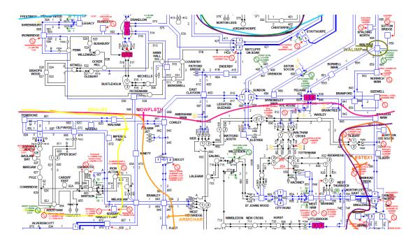
156. LOWFLSTH captures issues associated with insufficient generation across the South of England. This limit can be active under both pre and post fault conditions. This limit is typically managed by increasing generation in the South or trading to increase imports on the IFA.
