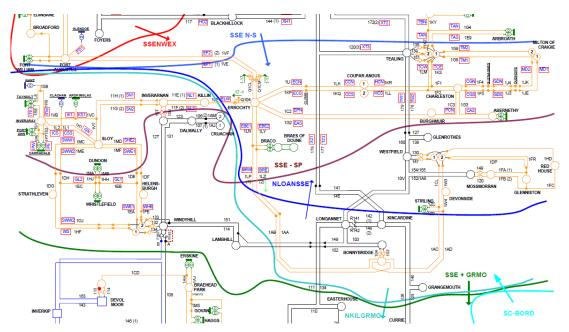
146. System instability constrains the transfer that can be secured across this boundary. The transfer that can be secured across this boundary is heavily dependent on the number of Longannet generators synchronised and the output of each generator. This is modelled by considering only the output of generation at Longannet and using the corresponding limit.
