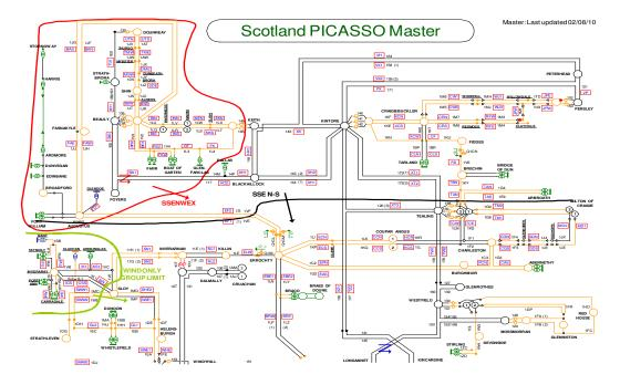
143. All generation behind this boundary is wind generation. As such, costs to manage any constraints can be significant. Under the Connect and Manage Regime, this boundary is likely to become active under pre and post fault conditions.
