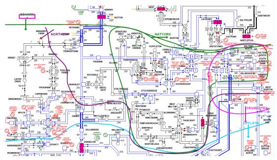
151. This boundary captures the thermal issues resulting from high output from Aire Valley generation, flowing South West. This issue is exacerbated overnight when Dinorwig generation switches into pump mode.
