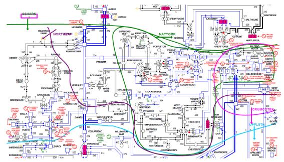
152. This boundary is active during outages of circuits along the boundary and is driven by thermal issues resulting from high transfers from Scotland combined with high output from generation
