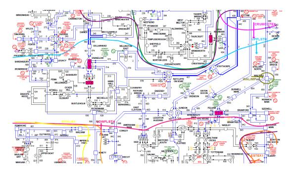
155. WALIMP is a thermal import constraint enclosing the demand at Walpole. Walpole has 4 off 240MVA Supergrid transformers and when one of these is on a planned outage, for the loss of a remaining transformer, the firm capacity is down to 480MVA. The demand at Walpole can exceed this level at peak periods making the WALIMP constraint active. Embedded generation at Kings Lynne/Peterborough will be constrained on to secure the local demand.
