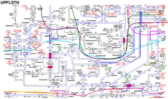
154. The boundary serves to capture thermal issues resulting from the loss of a double circuit along the boundary. Within the model it will also serve to secure any voltage limitation on the FLOWSTH boundary.
