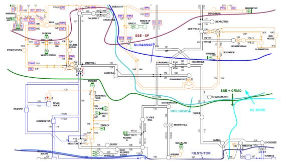
147. This boundary describes a thermal limit on the transfers which can be secured. A programme of works at several substations on the boundary has increased the boundary capability. It is not likely to be a limiting boundary on the system prior to completion of the Beauly-Denny circuit.
