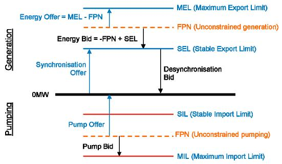
Figure 6 showing the balancing mechanism price-quantity relationships
