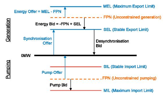
Figure 5 showing the balancing mechanism price-quantity relationships
