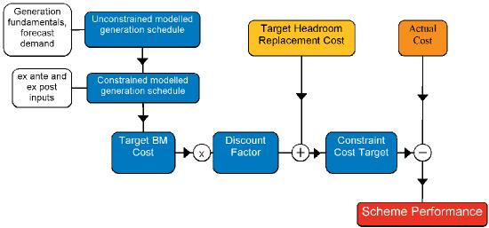
Figure 1: Overview of constraint modelling process
