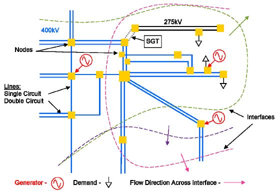
Figure 2 showing extract of E+W electricity network
