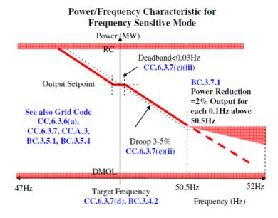
Figure C2: Frequency Sensitive Operation Inverter Mode
