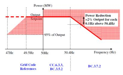
Figure C1: Limited Frequency Sensitive Mode Inverter Operation
