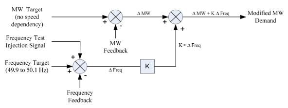
Figure C3: Typical Frequency Test Injection Scheme
