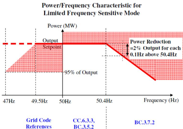
Figure C1: Limited Frequency Sensitive Mode Inverter Operation
