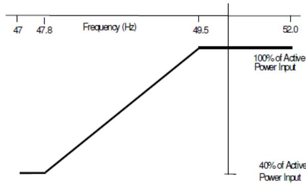
Figure C1b – Limited Frequency Sensitive Mode Rectifier Operation
