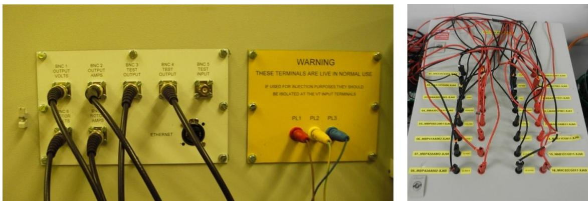
Figure 1 – Example of Compliance Test Signal Connections
