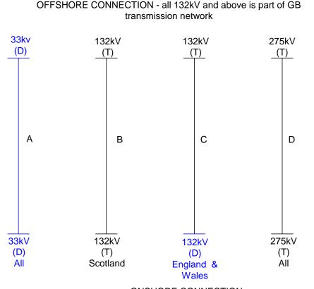
ONSHORE CONNECTION 132/275/400kV circuits are part of GB Transmission network in Scotland Only 275/400 circuits are part of GB Transmission network in England & Wales
