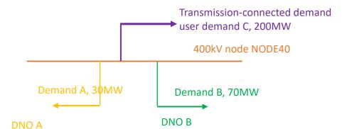
As demand C connects at a Connection Site consisting of connections to more than one demand zone, for the purpose of DCLF Transport modelling and calculation of demand zonal tariffs, demand C is spread evenly across the multiple GSP Groups (A and B). Therefore demand C at NODE40 is split into two parts: 100MW at GSP Group A, and 100MW at GSP Group B. The zonal demand at A and B is calculated as below (copying 14.15.41):
