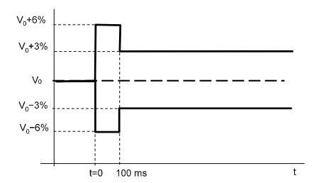
Figure ECC.6.1.7 (1) — Voltage characteristic for frequent events
