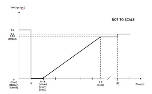
Figure ECC.6.3.15.7 - Voltage against time curve applicable to HVDC Systems and Remote End HVDC Converter Stations
