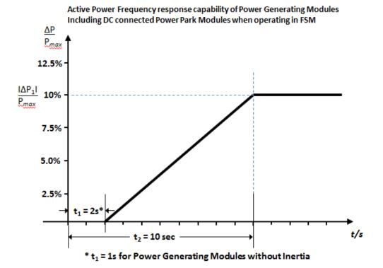
Figure 6.3.7.3.3(b) Active Power Frequency Response capability.
