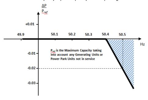
Figure ECC.6.3.7.1 –  $P_{ref}$  is the reference **Active Power** to which  $\Delta P$  is related and  $\Delta P$  is the change in **Active Power** output from the **Power Generating Module** (including **DC Connected Power Park Modules**) or **HVDC System**. The **Power Generating Module** (including **DC Connected Power Park Modules** or **HVDC Systems**) has to provide a negative **Active Power** output change with a droop of 10% or less based on Pref.
