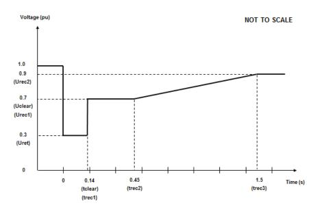
Figure ECC.6.3.15.2 - Voltage against time curve applicable to **Type B Synchronous Power Generating Modules**
