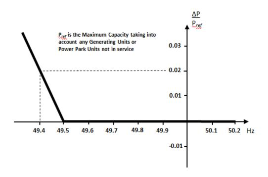
Figure ECC.6.3.7.2.2 –  $P_{ref}$  is the reference **Active Power** to which  $\Delta P$  is related and  $\Delta P$  is the change in **Active Power** output from the **Power Generating Module** (including **DC Connected Power Park Modules**) or **HVDC System**. The **Power Generating Module** (including **DC Connected Power Park Modules** or **HVDC Systems**) has to provide a positive **Active Power** output change with a droop of 10% or less based on Pref.
