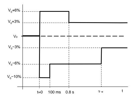
Figure ECC.6.1.7 (2) — Voltage characteristic for infrequent events
