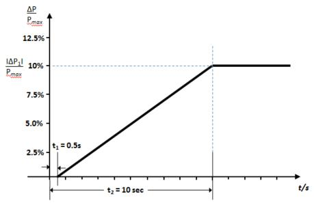
Figure 6.3.7.3.4(b) **Active Power Frequency Response** capability of a **HVDC System**. ΔP is the change in **Active Power** triggered by the step change in frequency
