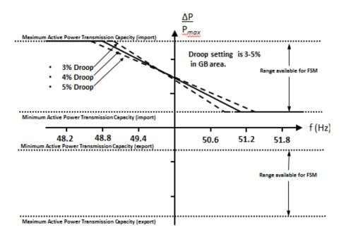
Figure 6.3.7.3.4(a) – **Active Power** frequency response capability of a **HVDC System** operating in **Frequency Sensitive Mode** (FSM).  $\Delta P$  is the change in active power output from the **HVDC System**..
