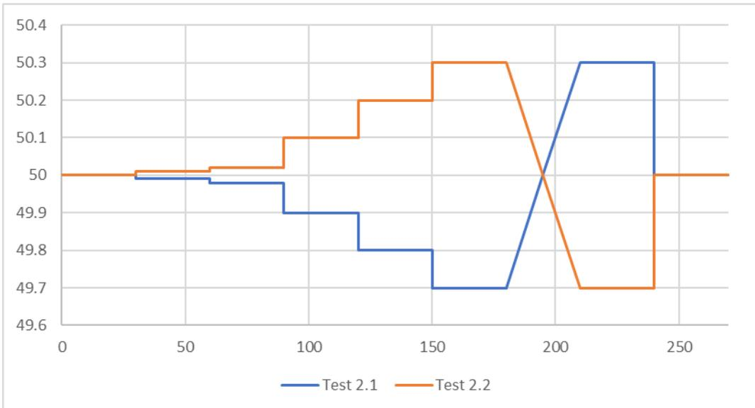
Pass Criteria for Tests 2.1 and 2.2
