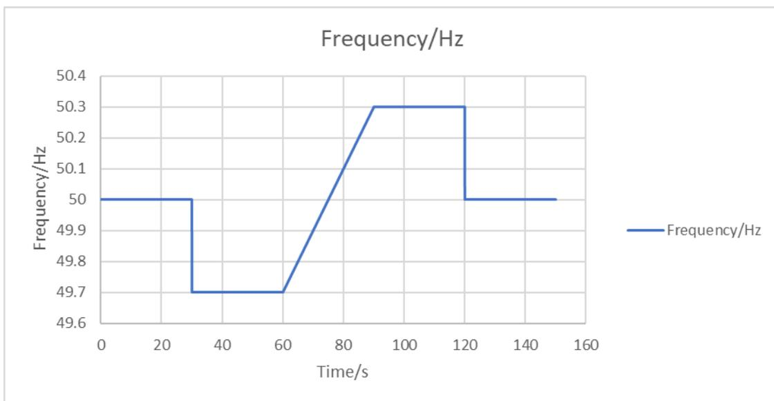
Table 11 - Test 2 Frequency Injection Profiles
