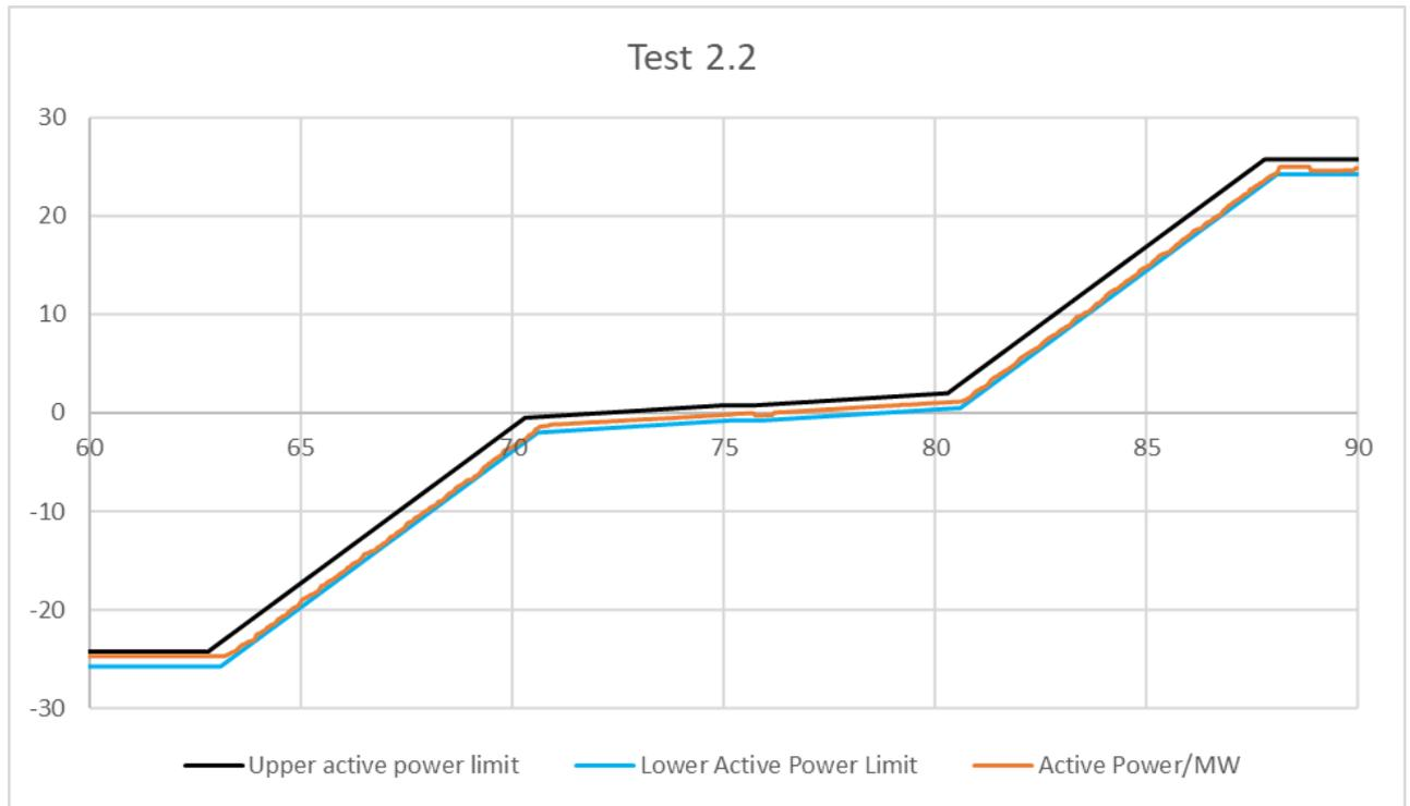
Table 5 - Test 2.1 and 2.2 Sweep Test tolerances (Without time delay to reach required delivery included)
