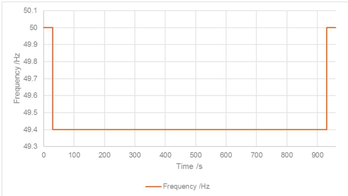
Table 6: Test 3.1 Frequency Injection Table Corresponding with times
