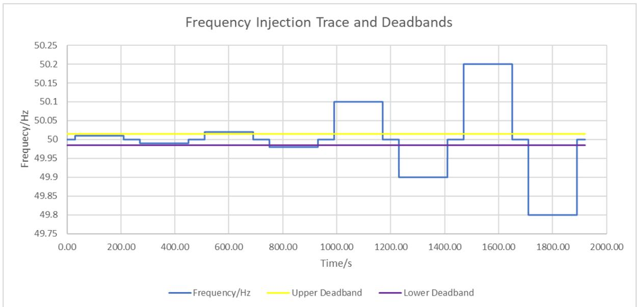
Table 9 - Test 1 Frequency Injection Profile corresponding with times
