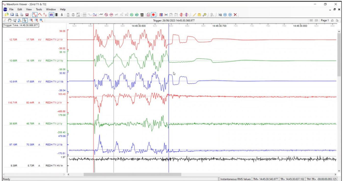
Figure 105: Transmission fault recorder capture during protection trip
