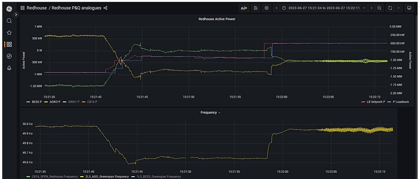
Figure 118: Diesel generator step from 2 MW to 0.05 MW
