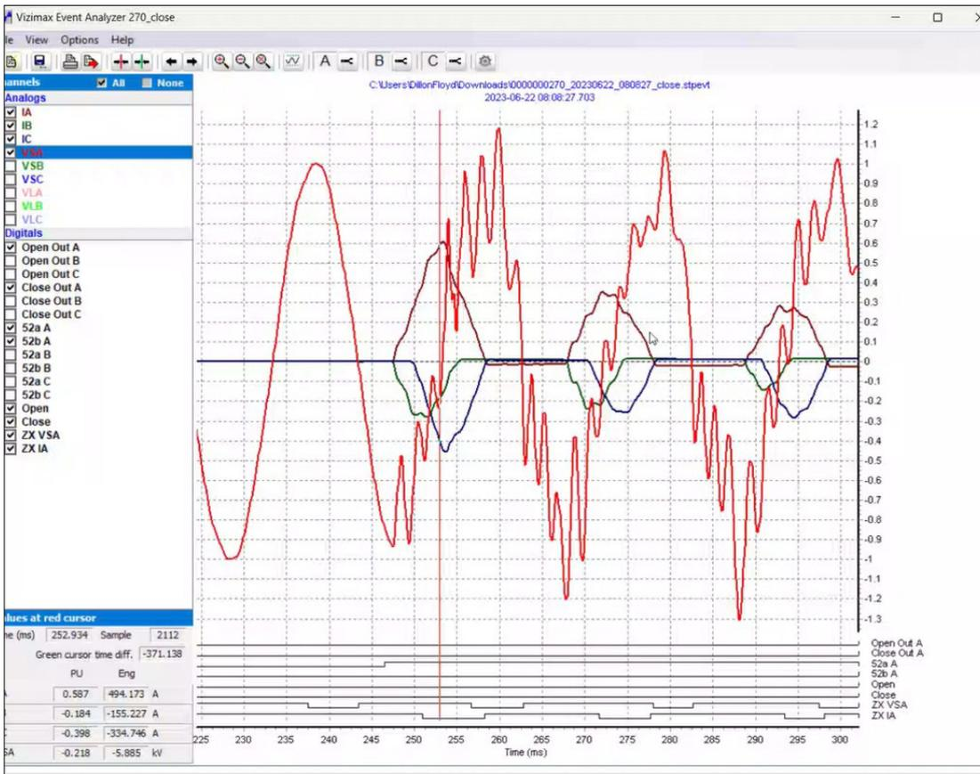
Figure 51: Voltage and current signals from PoW relay, failed Redhouse energisation
