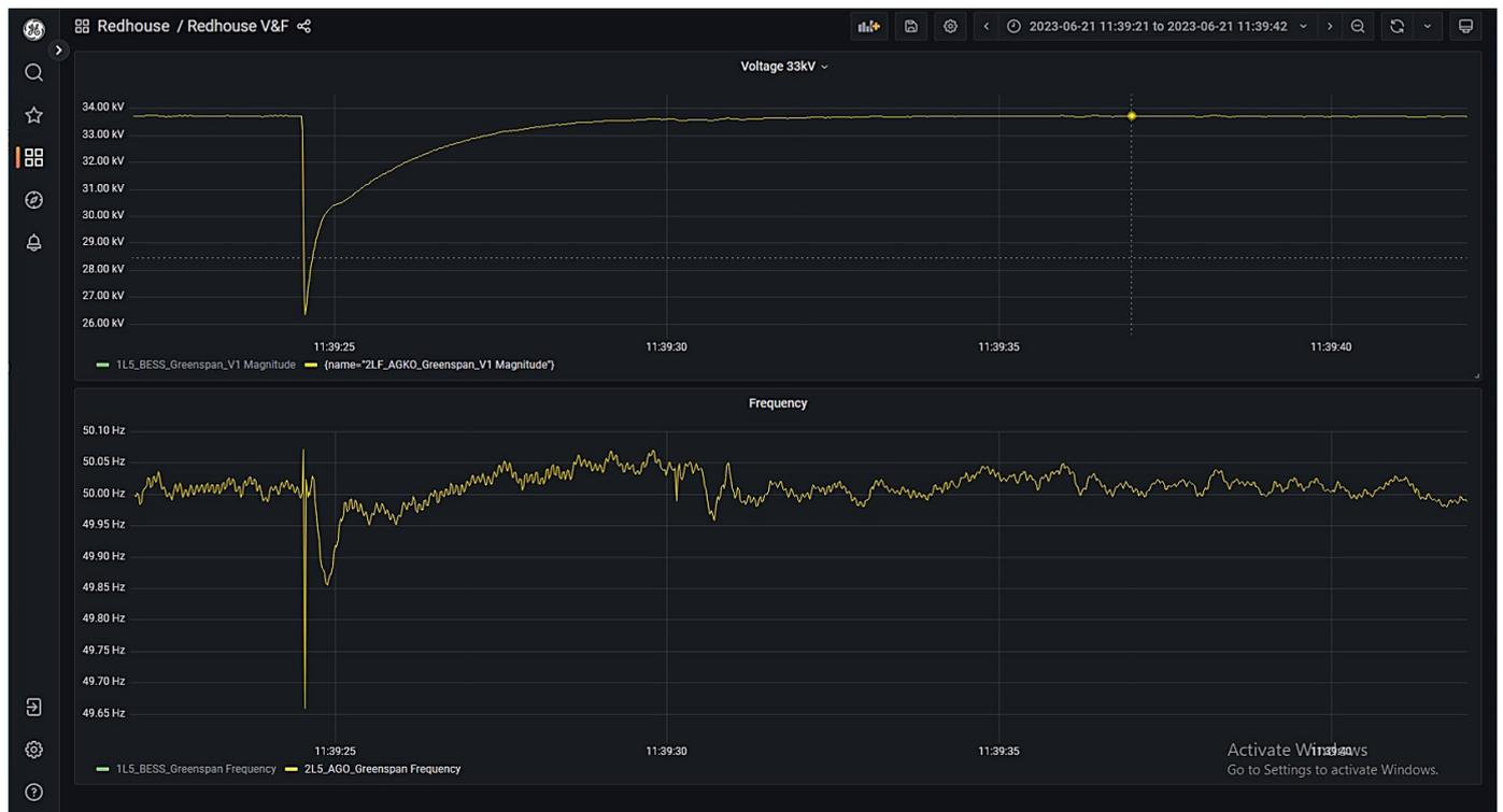
Figure 22: Redhouse primary T1 energised via the diesel generator without PoW
