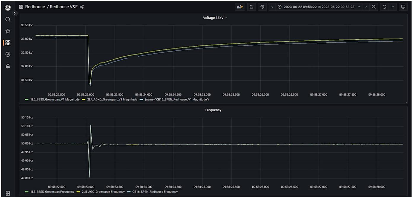
Figure 53: Redhouse primary T1 energised via BESS without PoW
