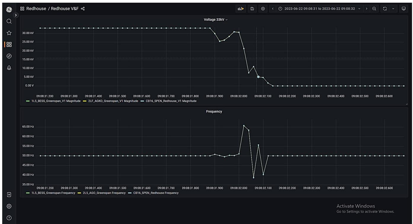
Figure 49: Redhouse primary T1 energisation attempt via BESS with PoW (BESS internal protection tripped)
