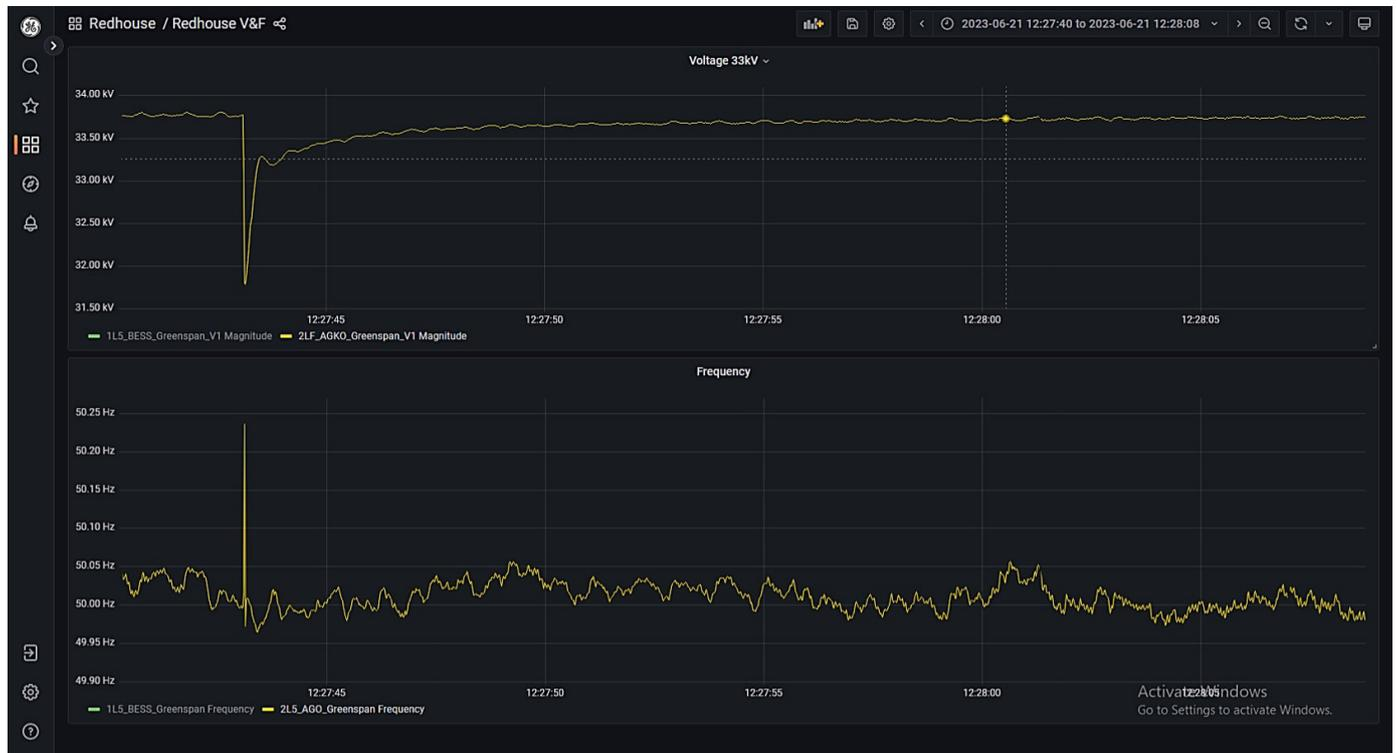
Figure 23: Redhouse primary T1 energised via the diesel generator with PoW
