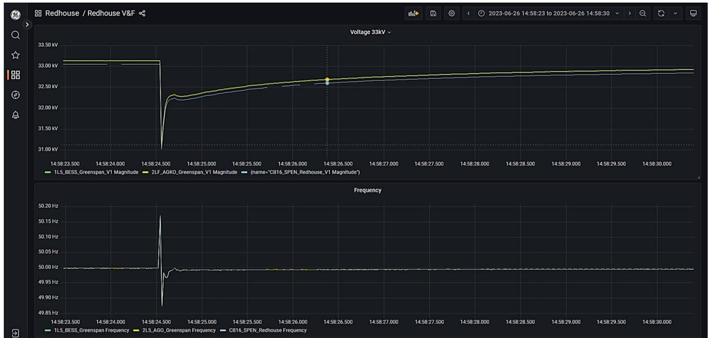
Figure 99: Redhouse GT1 and 132 kV OHL energised via the BESS without PoW
