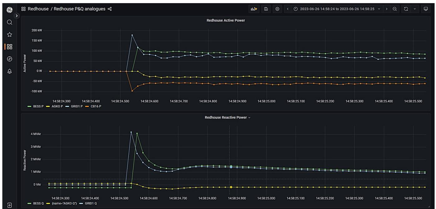
Figure 100: Redhouse GT1 and 132 kV OHL energised via the BESS without PoW
