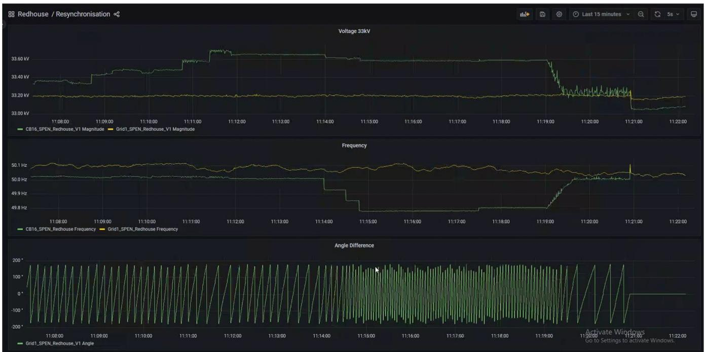
Figure 120: Voltage and frequency offset and resynchronisation via load bank control
