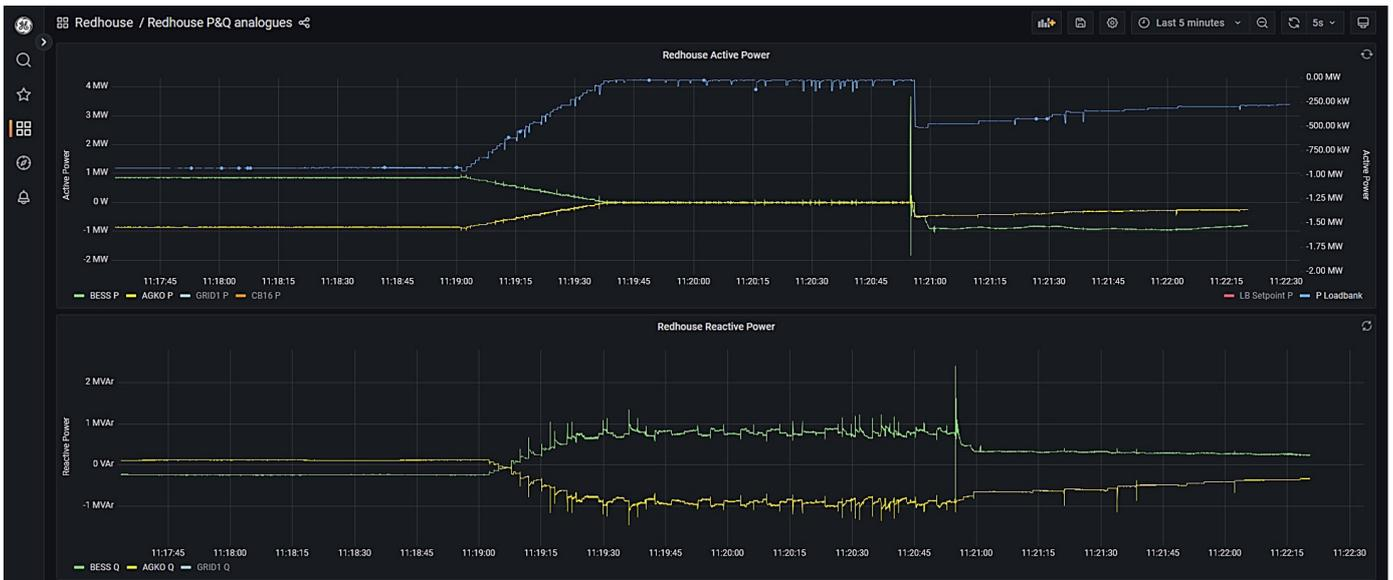
Figure 121: Active and reactive power before and after the closure of grid 1
