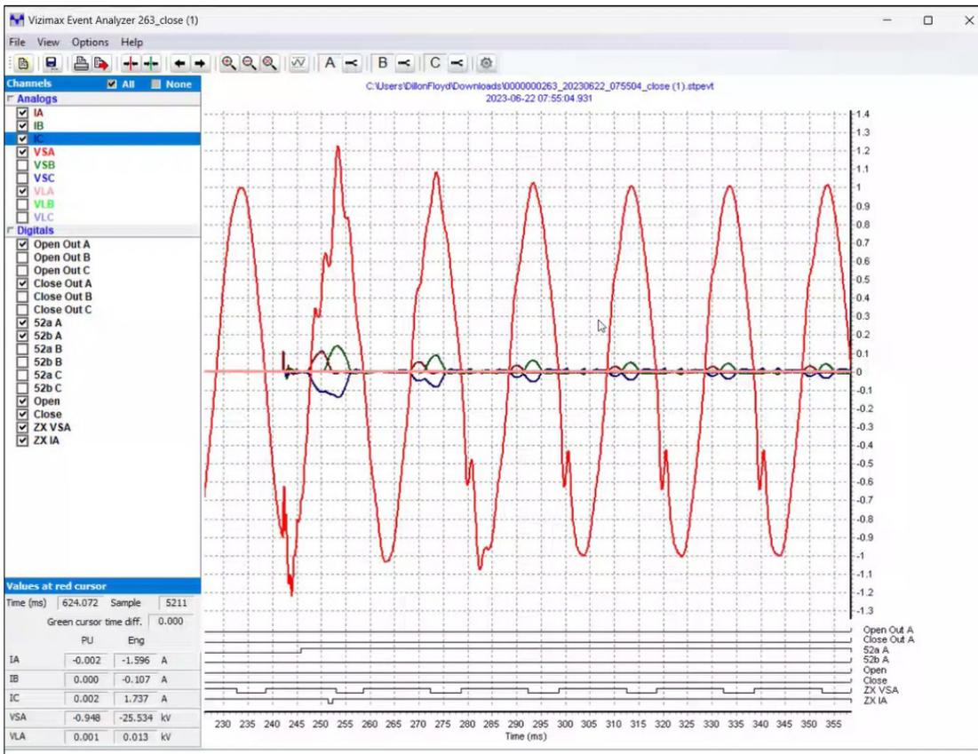
Figure 52: Voltage and current signals from PoW relay, successful Chapel energisation
