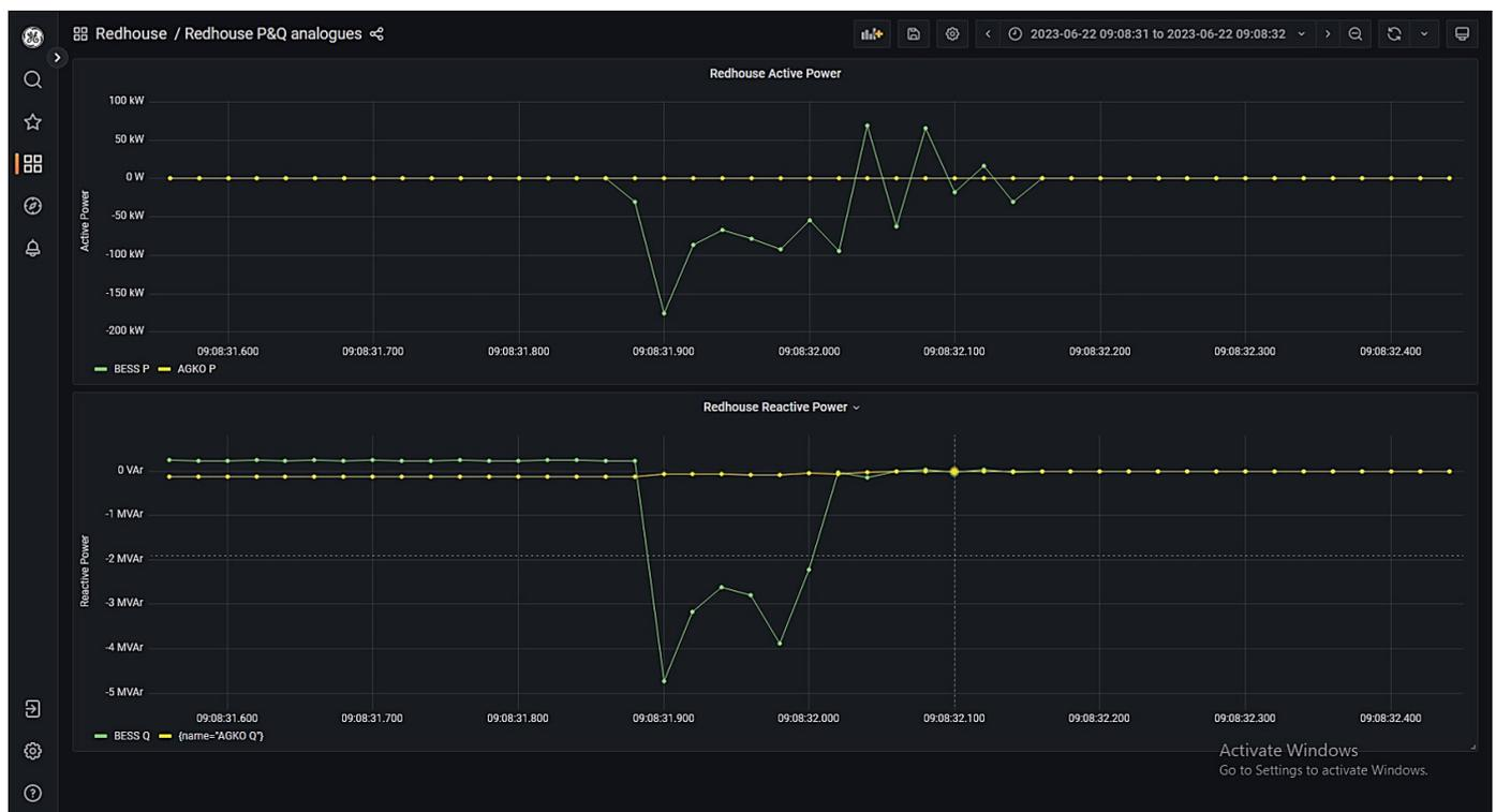
Figure 50: Redhouse primary T1 energisation attempt via BESS with PoW (BESS internal protection tripped)
