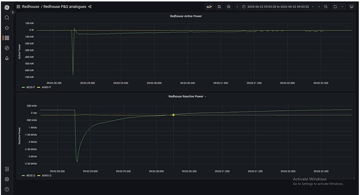
Figure 48: Chapel primary T1 energised via BESS with PoW
