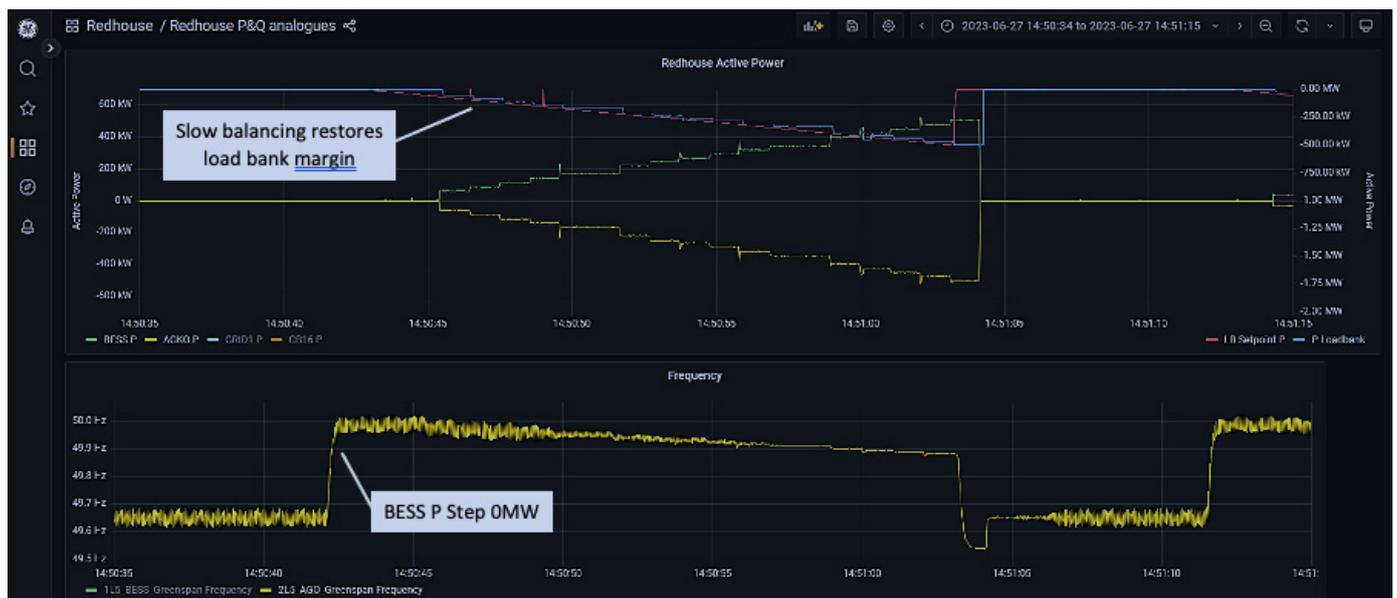
Figure 116: Slow balancing action to restore load bank margin
