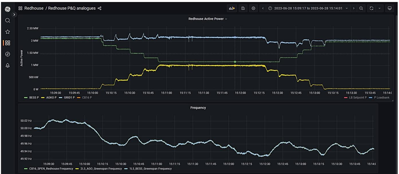
Figure 127: Diesel generator power steps while D-VPP mode is active with setpoint of 2 MW
