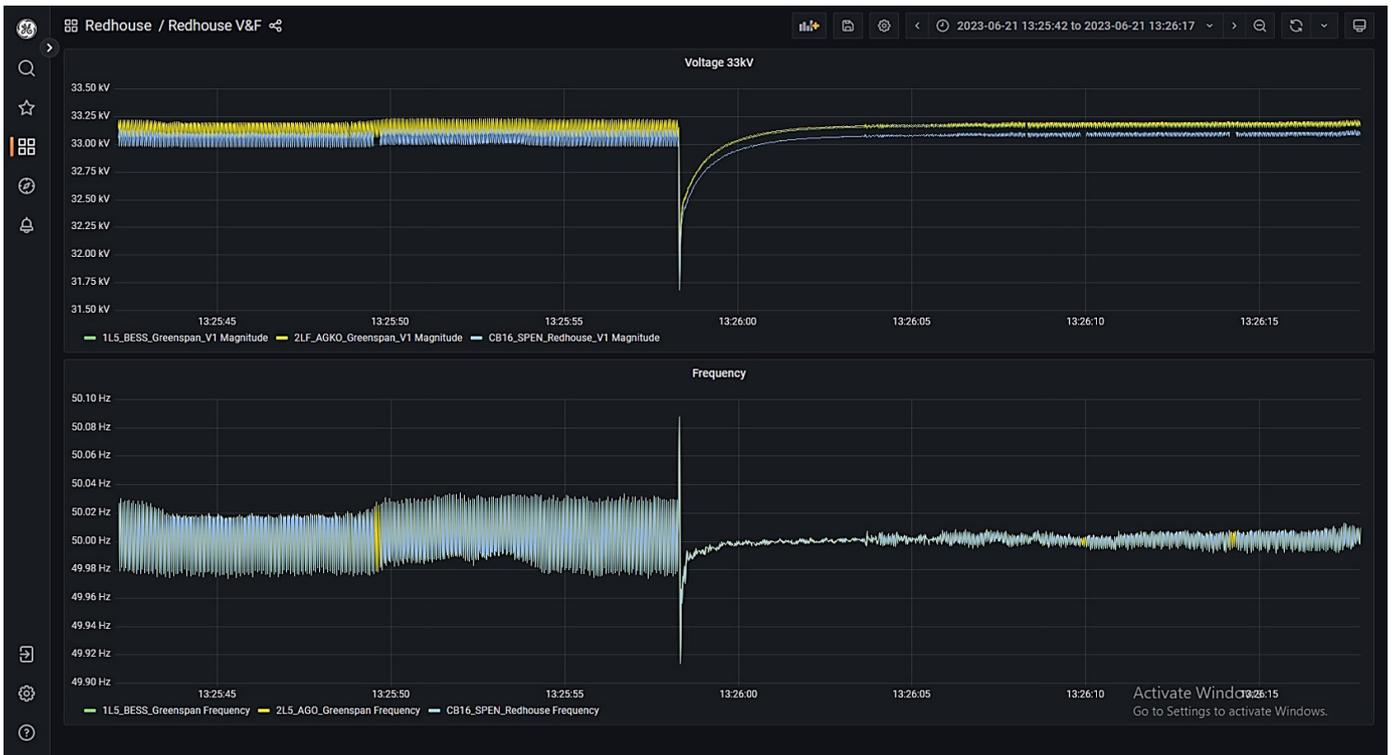
Figure 24: Chapel primary T1 energised via the diesel generator and grid-forming BESS without PoW
