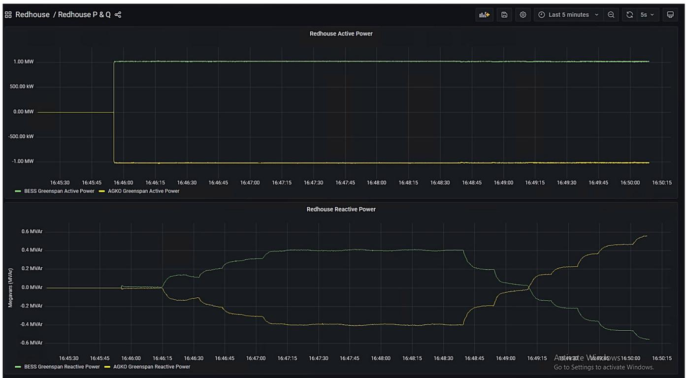
Figure 8: Active and reactive power of grid-following BESS under setpoint control
