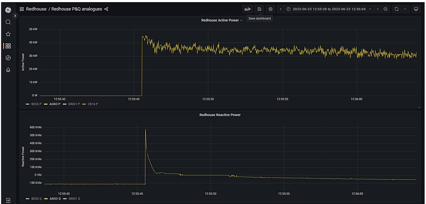
Figure 75: Redhouse GT1 energised via the diesel generator with PoW
