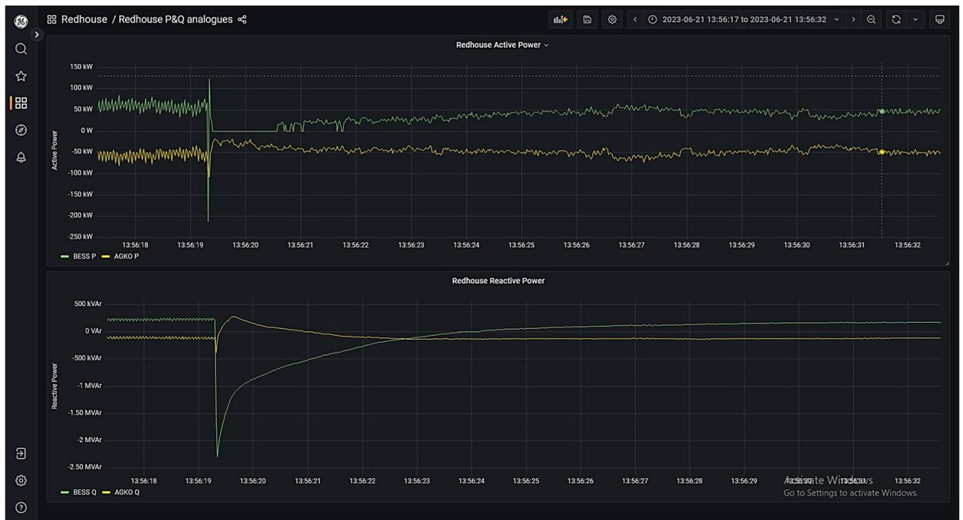
Figure 30: Redhouse primary T1 energised via the diesel generator and grid-forming BESS with PoW
