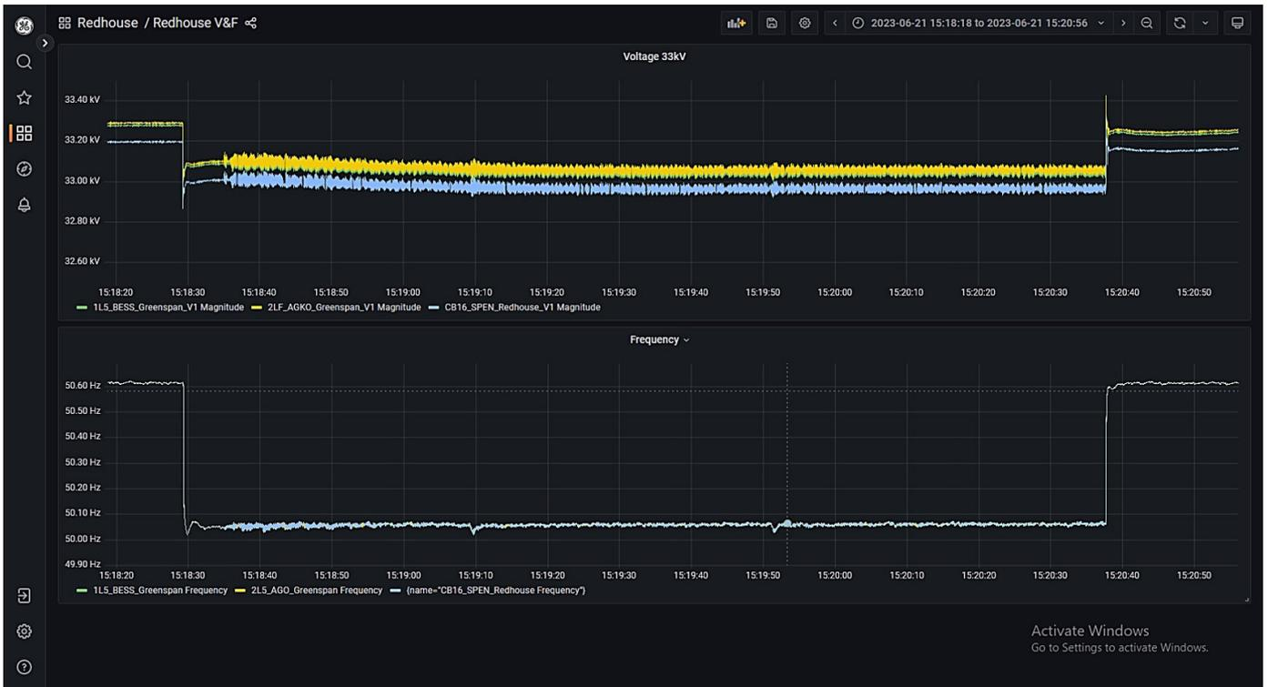
Figure 41: 2.5 MW load step applied to trial network with diesel generator, BESS and MBS connected
