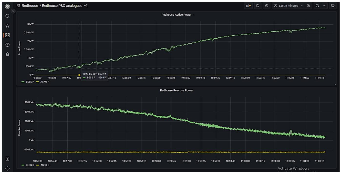
Figure 66: MBS output ramping up to ~3 MW
