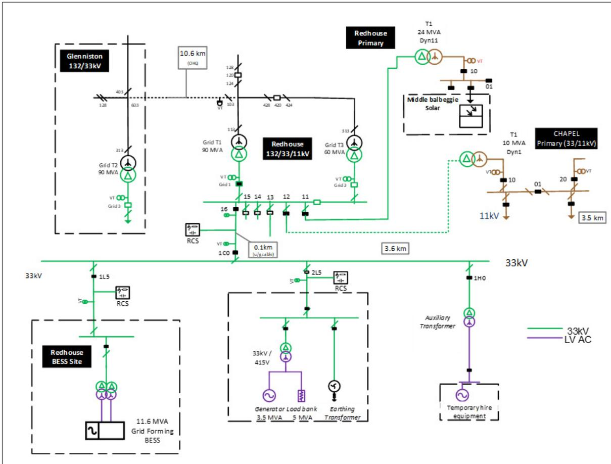
Figure 19: Phase 2 trial network diagram snapshot – SPEN network tests (CB positions may vary test by test)
