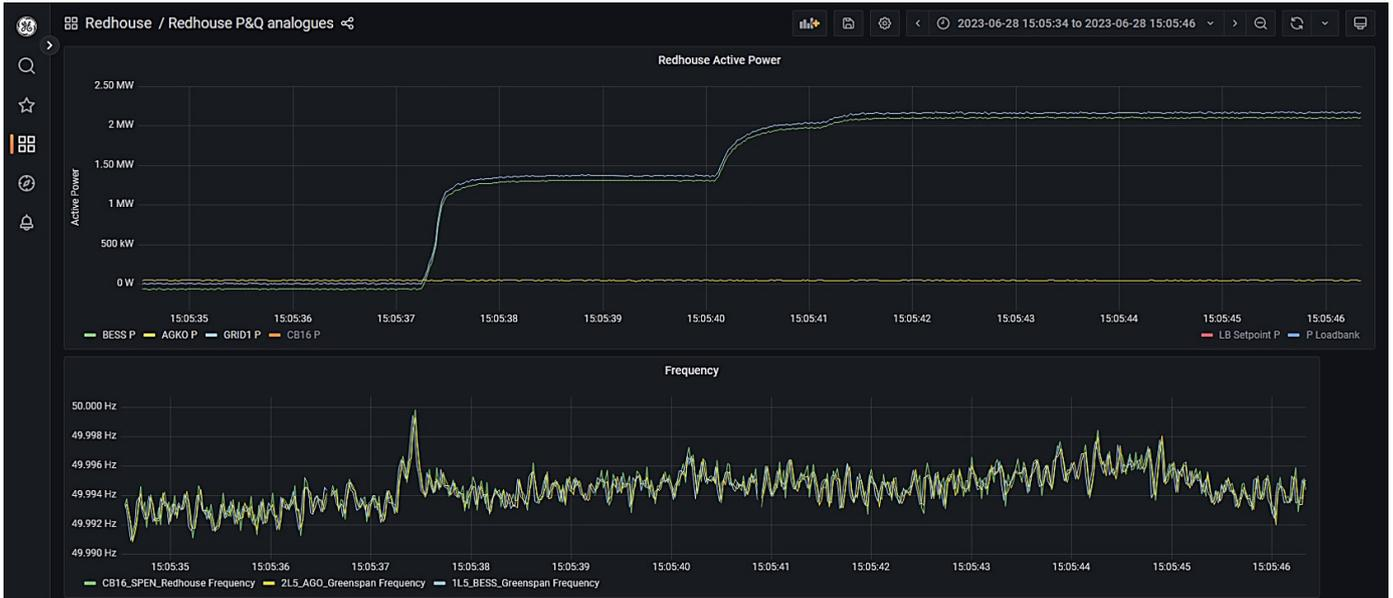
Figure 126: D-VPP setpoint change to 2 MW
