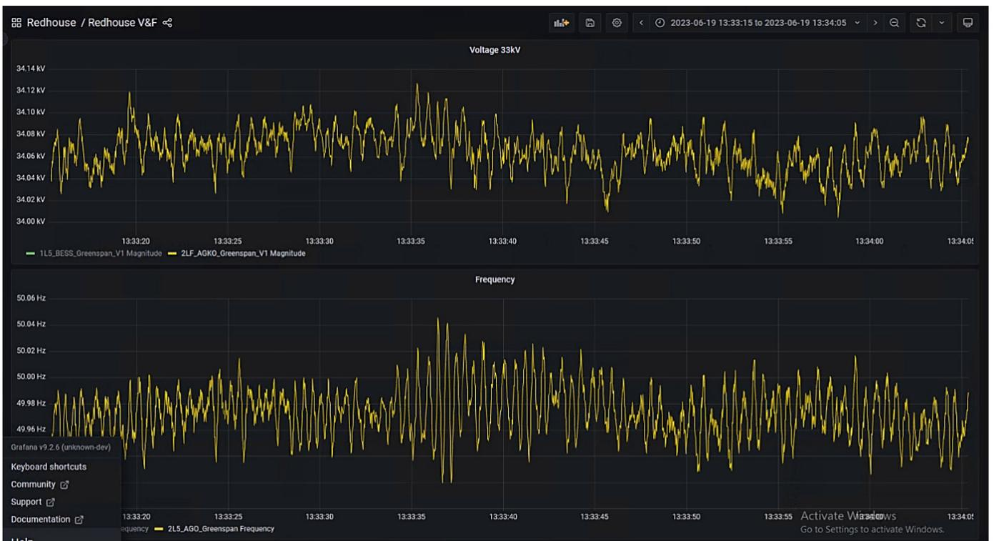
*Figure 6: Grid-following BESS synchronised with diesel generator, new settings applied*
