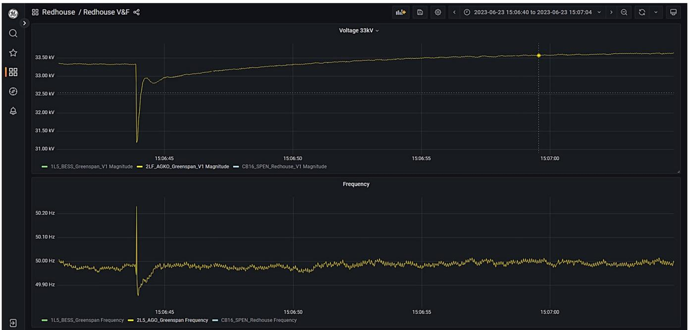
Figure 79: Redhouse GT1 and 132 kV OHL energised via the diesel generator with PoW
