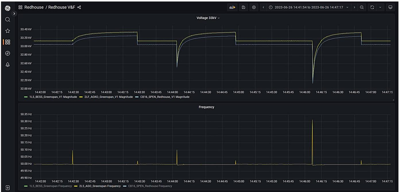
Figure 97: Redhouse GT1 and 132 kV OHL energised via the BESS with PoW
