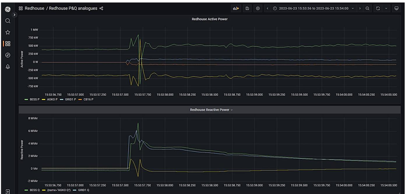
Figure 82: Redhouse GT1 energised via the BESS and diesel generator without PoW
