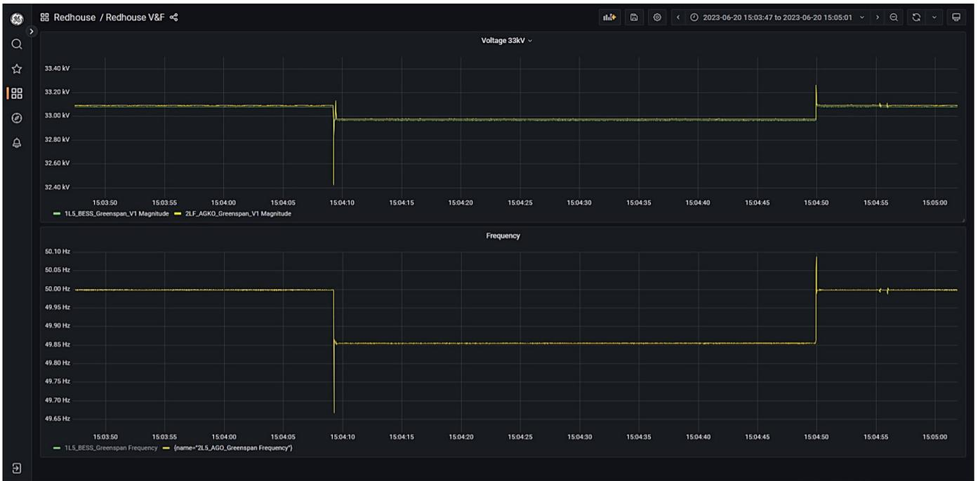
Figure 15: Grid-forming BESS voltage and frequency – 2.5 MW load step (1% droop)
