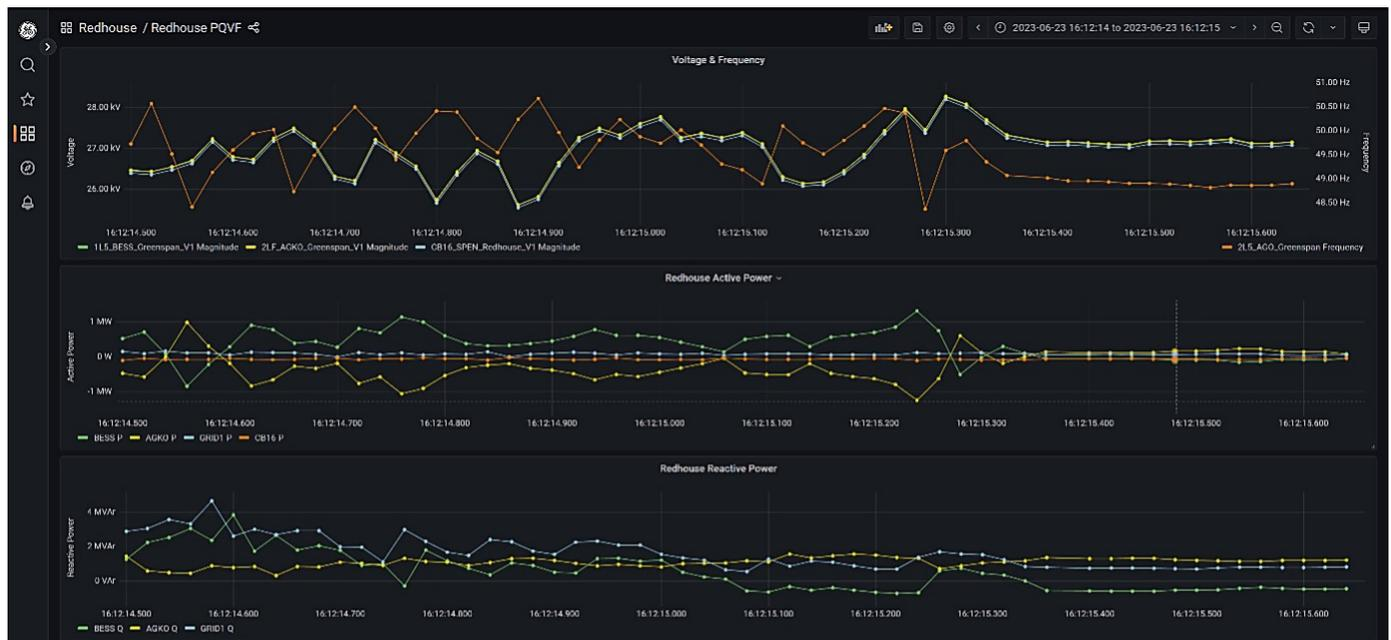
Figure 89: Stage 2 Highly variable V and f until stabilisation at low voltage
