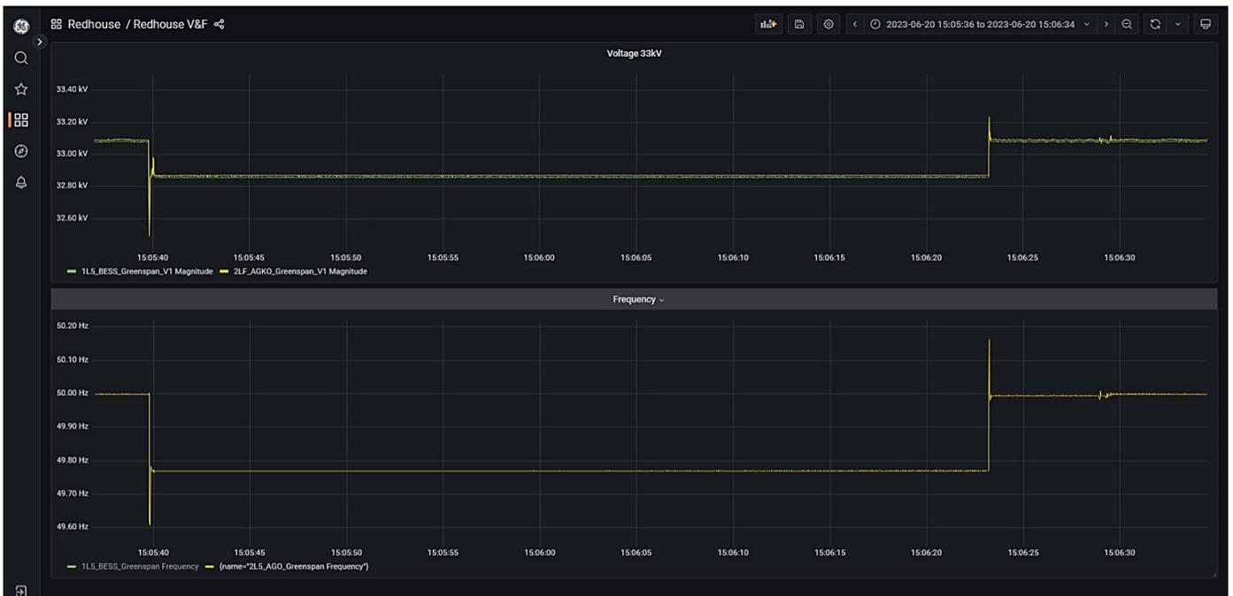
Figure 16: Grid-forming BESS voltage and frequency – 4 MW load step (1% droop)
