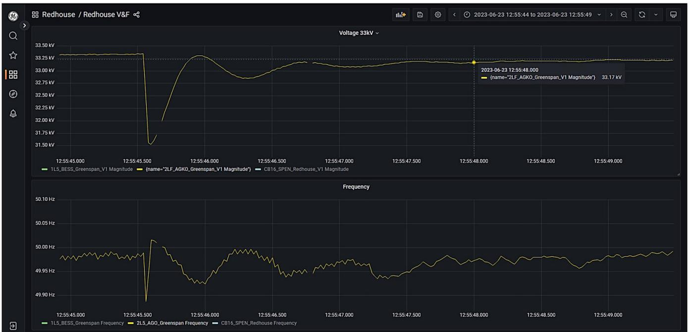
Figure 74: Redhouse GT1 energised via the diesel generator with PoW
