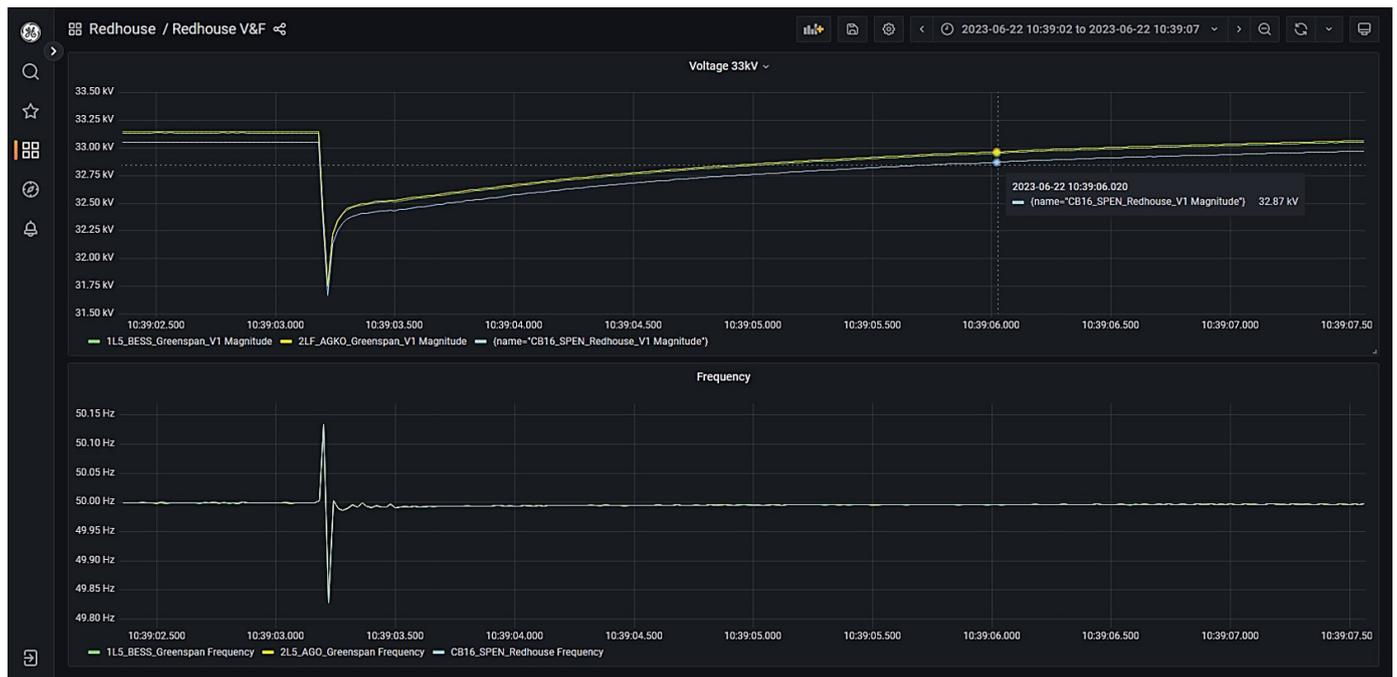
Figure 61: Chapel primary T1 and Redhouse primary T1 energised via BESS with PoW
