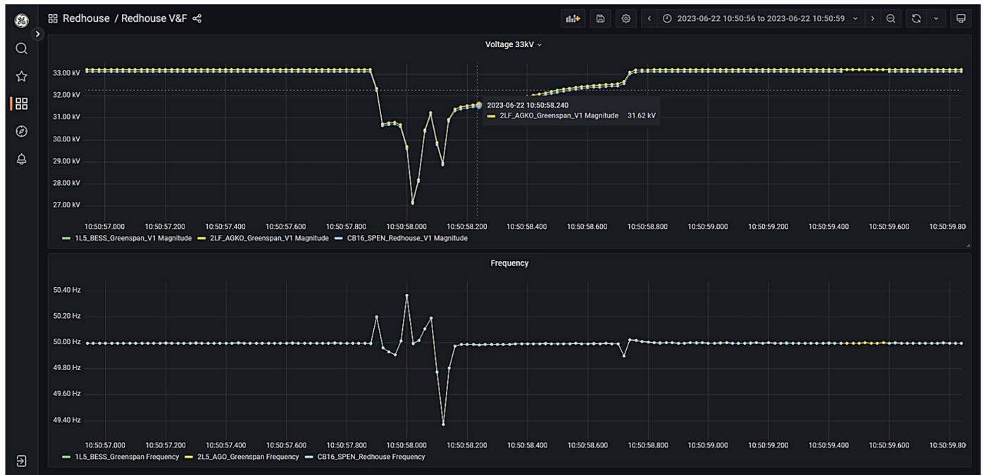
Figure 63: Energisation of Middle Balbeggie Solar transformers via BESS
