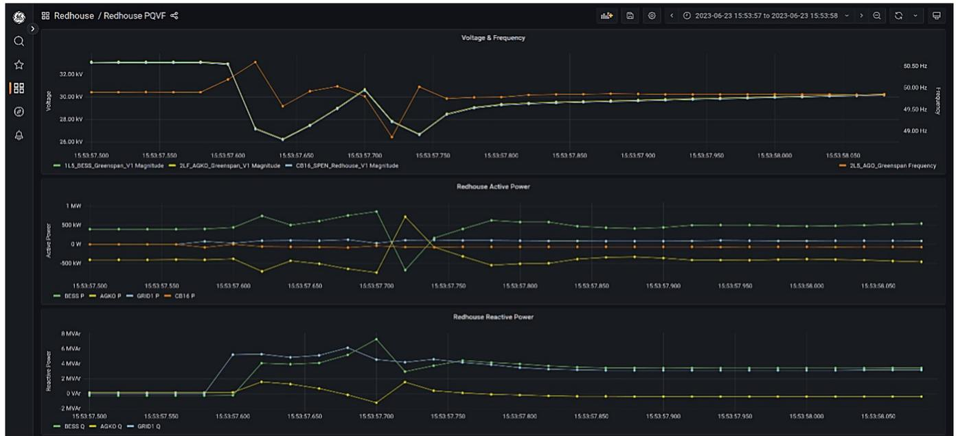
Figure 87: Comparison with grid 1 and 132 kV line energisation deep voltage depression 23-06-2023 1553 without PoW – successful but close to limit
