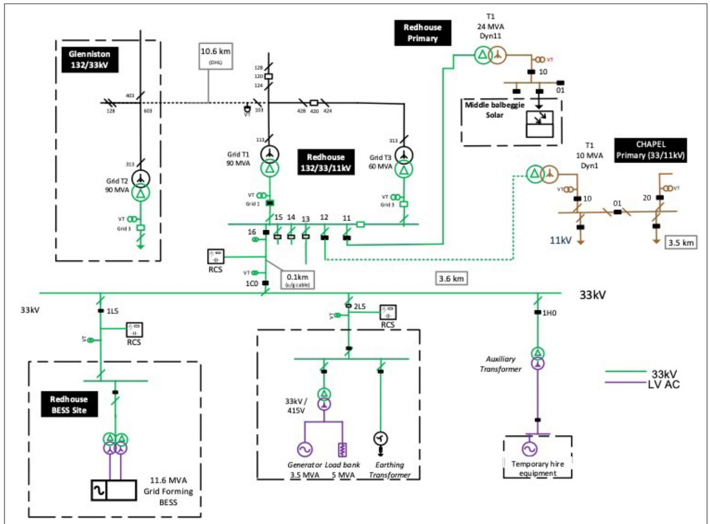
Figure 71: Phase 2 trial network diagram – Scottish Power transmission (SPT) network tests
