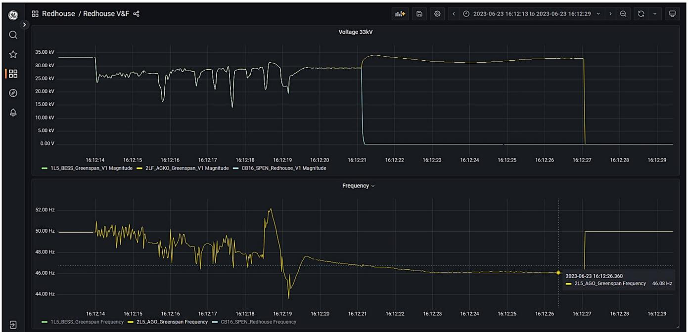
Figure 84: Redhouse GT1 and 132 kV OHL energisation attempt via the BESS and the diesel generator, instability led to trip
