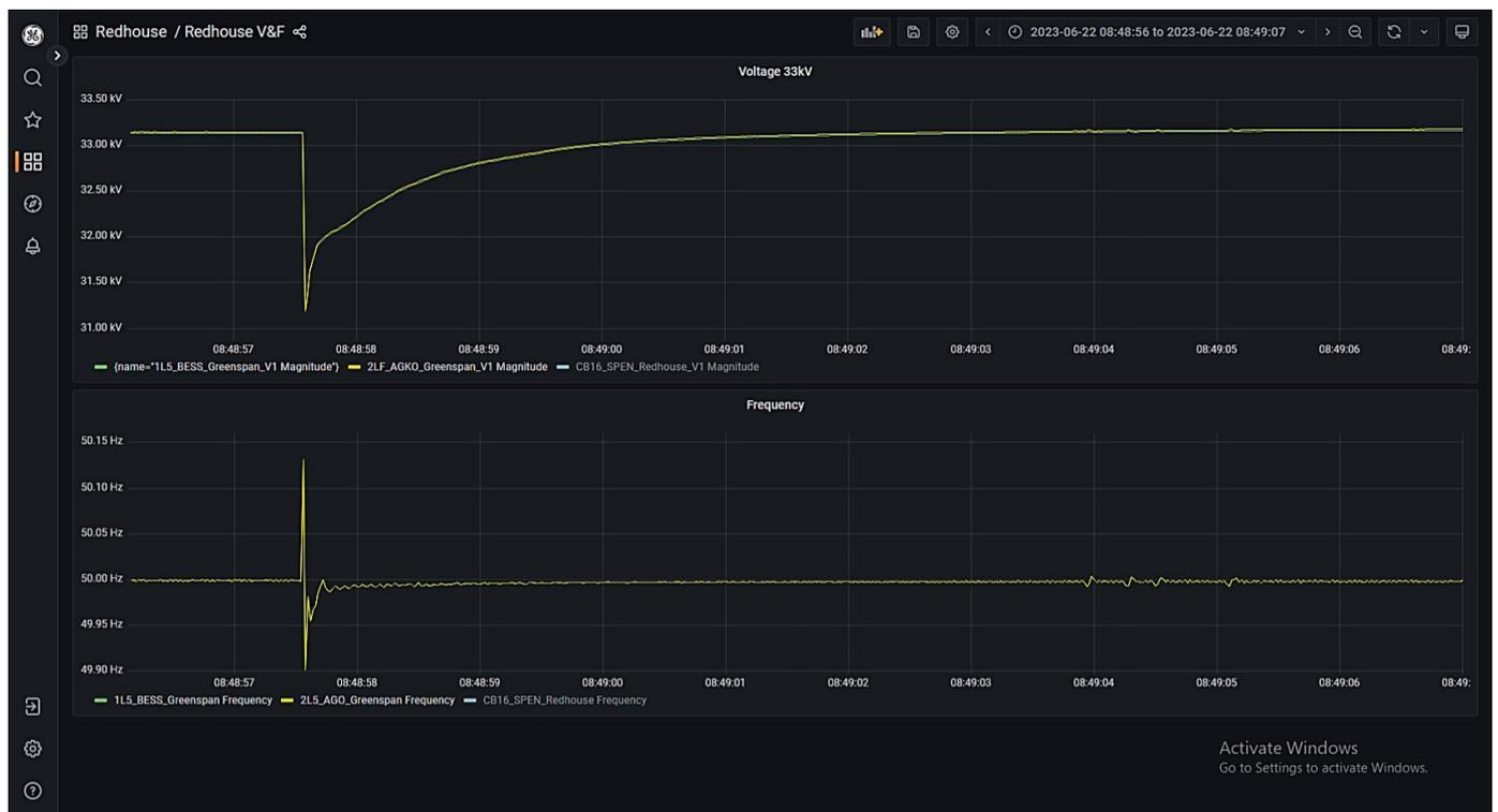
Figure 45: Chapel primary T1 energised via BESS without PoW
