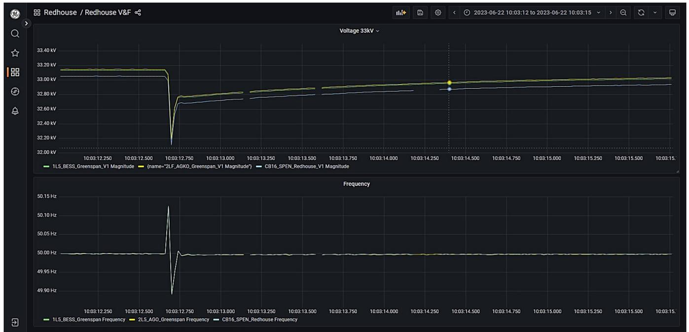
Figure 55: Redhouse primary T1 energised via BESS with PoW
