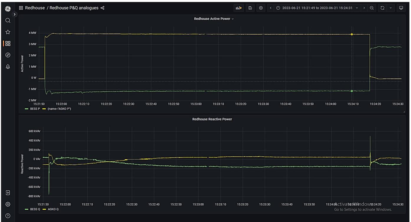
Figure 44: 4 MW load step applied to trial network with diesel generator, BESS and MBS connected
