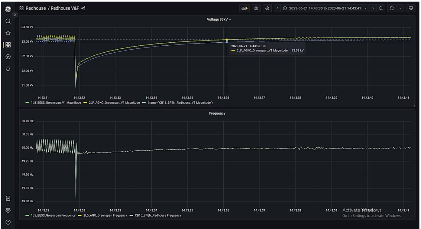
Figure 35: Chapel primary T1 and Redhouse primary T1 energised via the diesel generator and grid-forming BESS with PoW (updated operation time setting applied)
