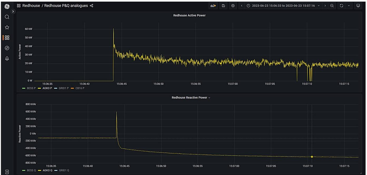
Figure 80: Redhouse GT1 and 132 kV OHL energised via the diesel generator with PoW
