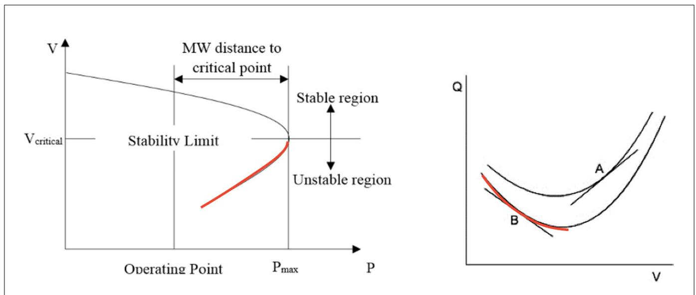
Figure 88: PV and QV stability curves
