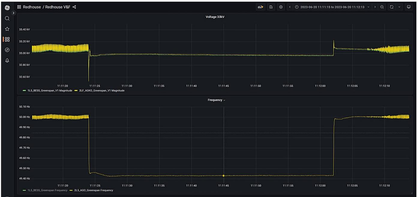
Figure 9: Grid-forming BESS and diesel generator voltage and frequency – 2.5 MW load step – on and off
