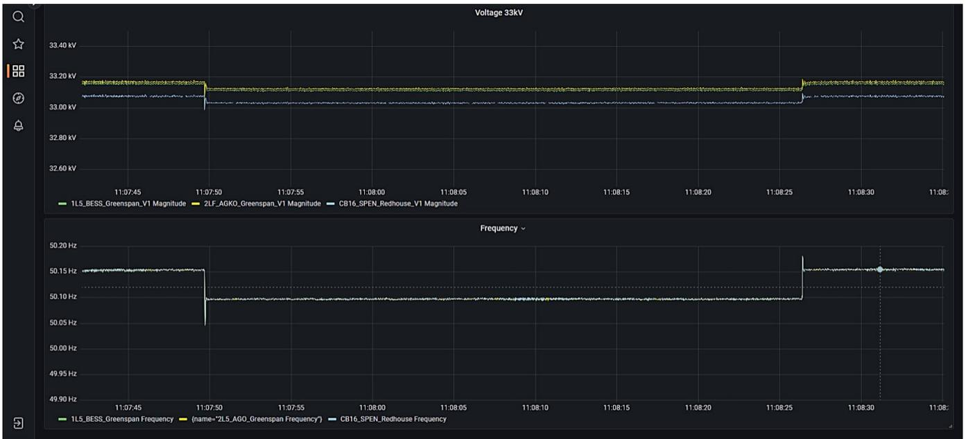
Figure 67: 1 MW load step applied to trial network with BESS and MBS connected
