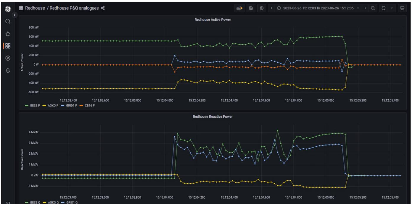
Figure 102: Redhouse GT1 and 132 kV OHL energisation attempt via the BESS without PoW – protection tripped
