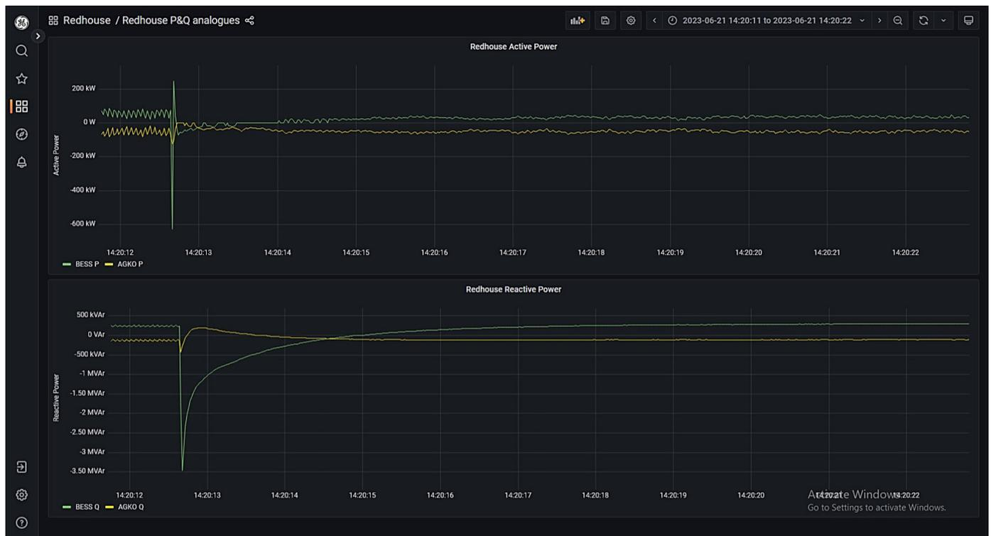
Figure 32: Chapel primary T1 and Redhouse primary T1 energised via the diesel generator and grid-forming BESS without PoW
