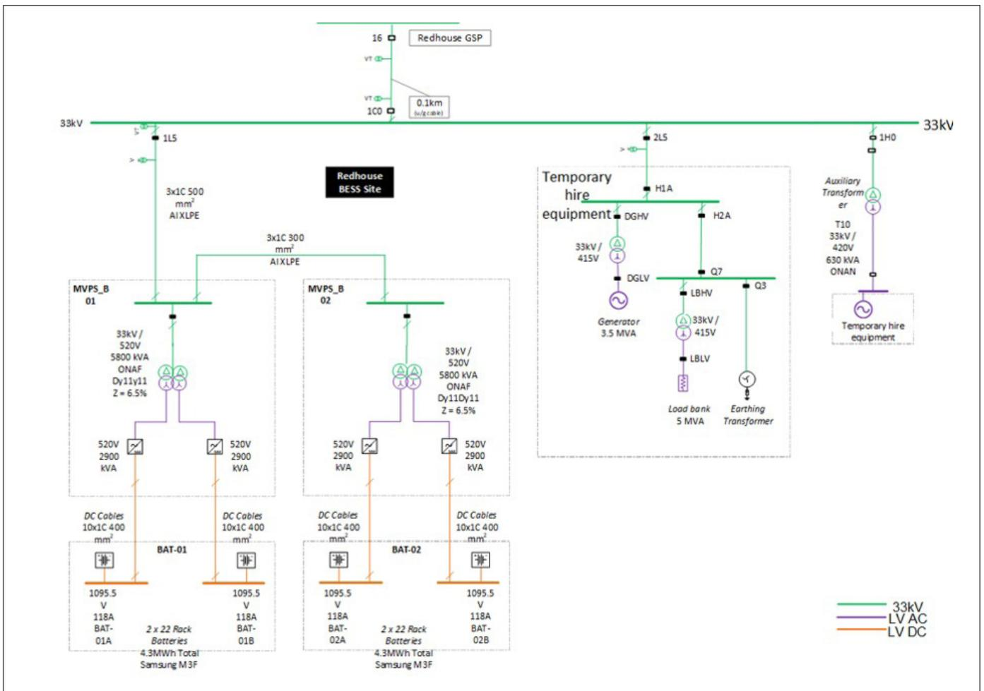
Figure 4: Phase 1 trial network diagram
