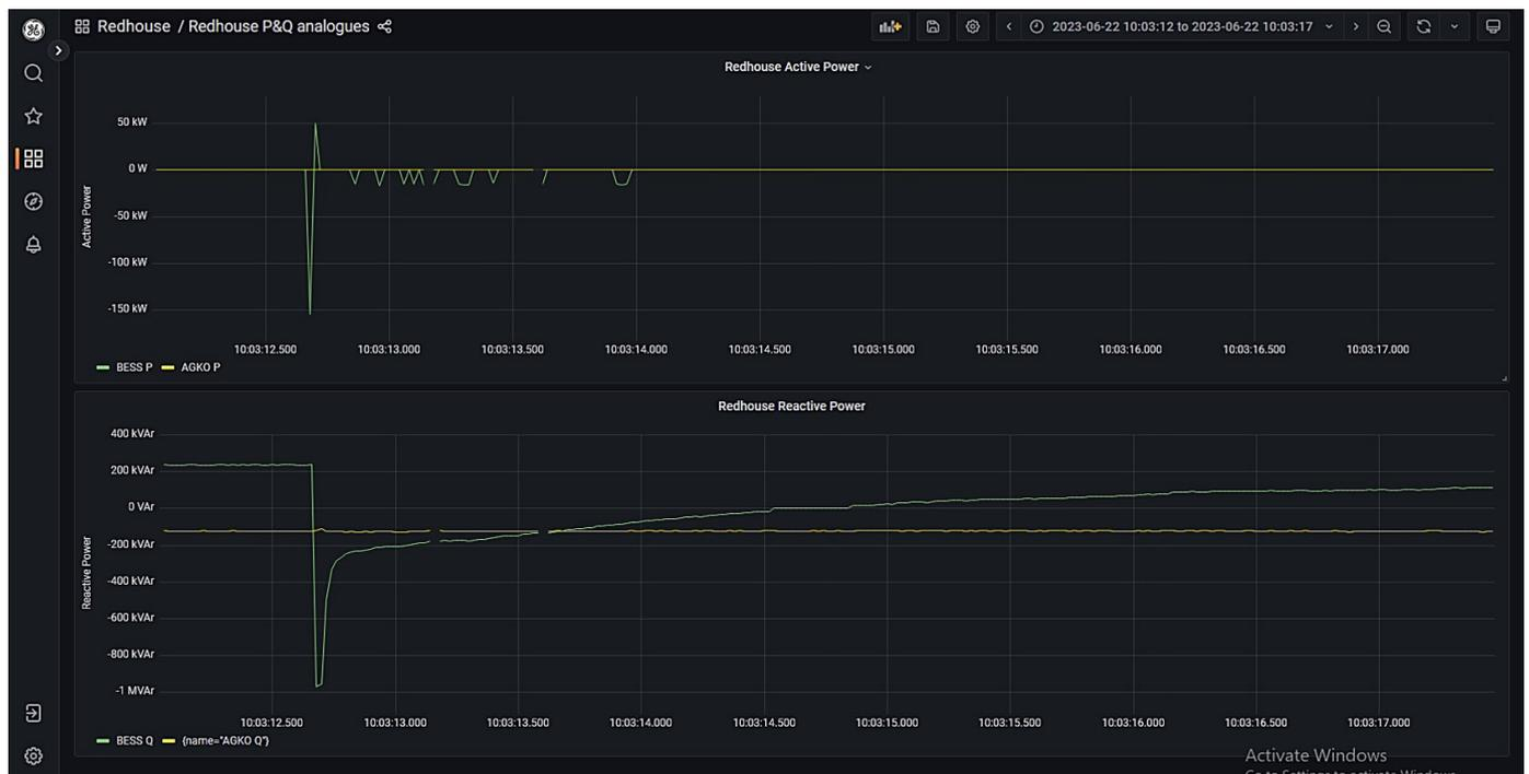
Figure 56: Redhouse primary T1 energised via BESS with PoW
