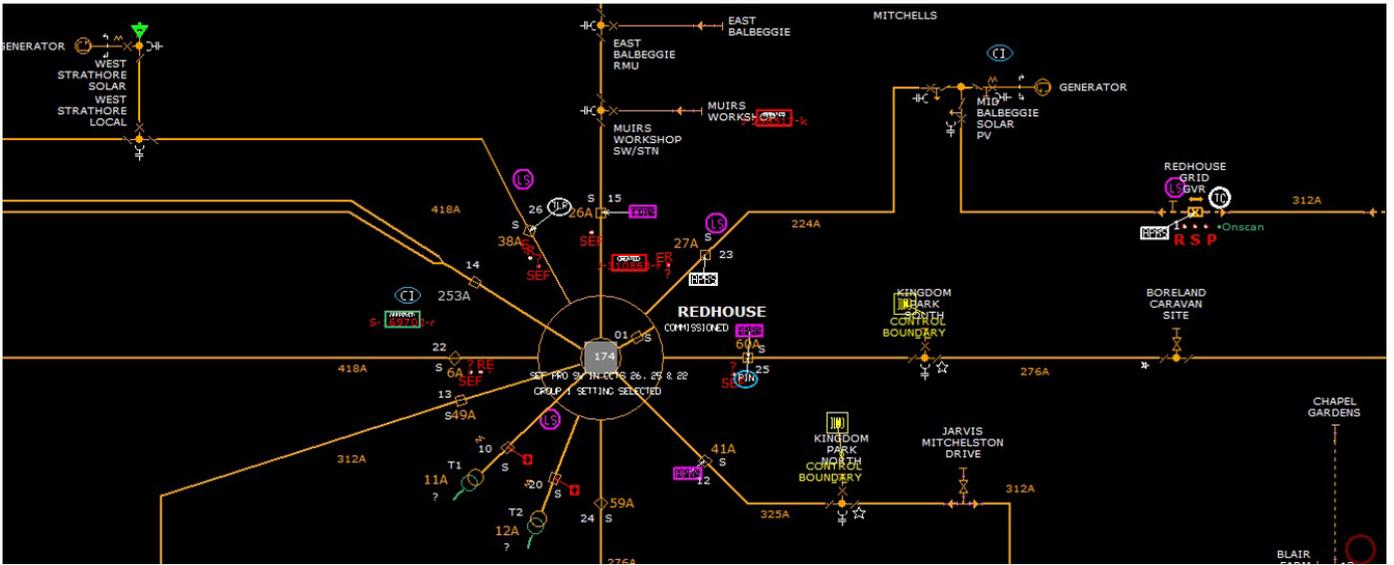
Figure 2: Redhouse primary network diagram (11 kV)
