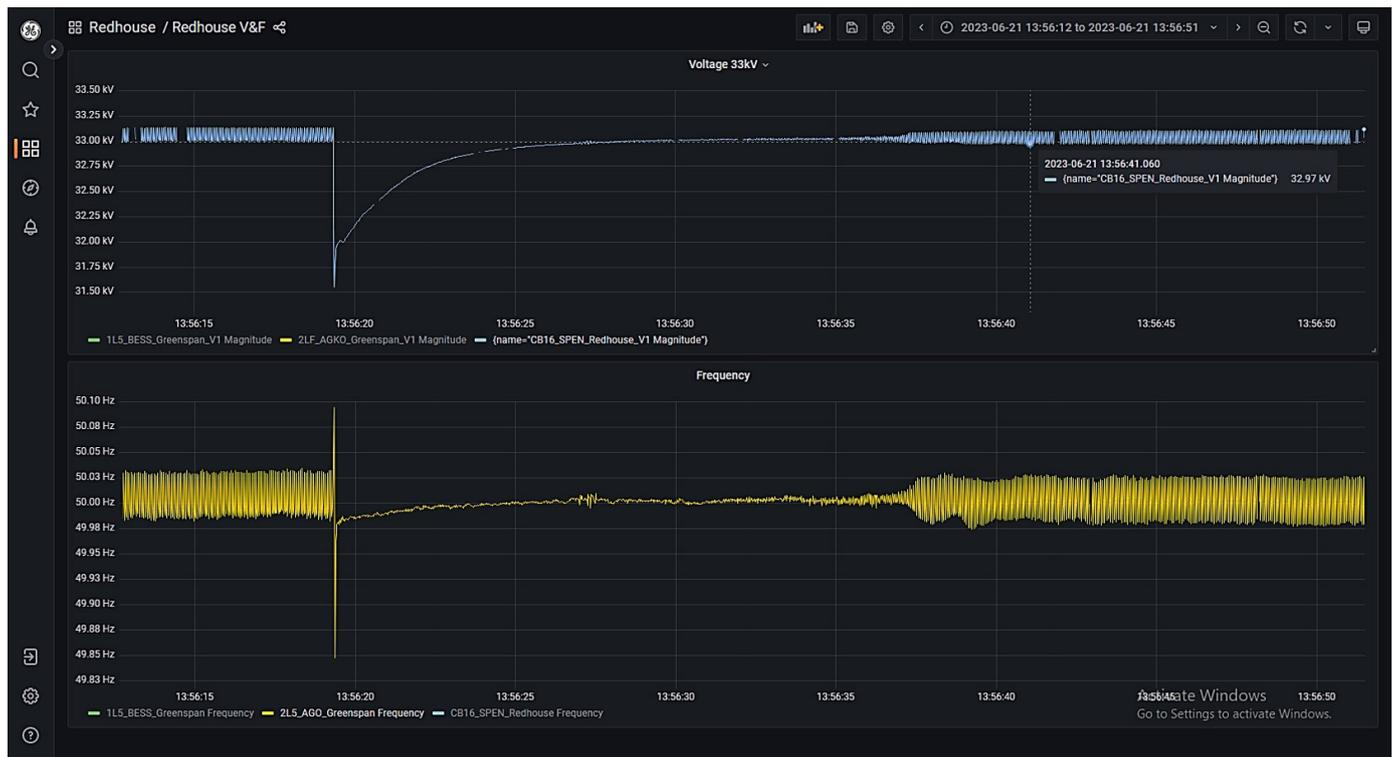
Figure 29: Redhouse primary T1 energised via the diesel generator and grid-forming BESS with PoW
