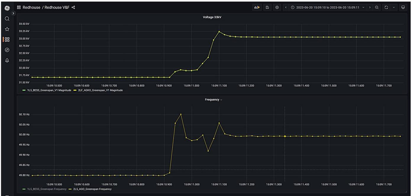
Figure 18: Grid-forming BESS voltage and frequency – 3.3 MW and 2.7 MVar load step (2/2)
