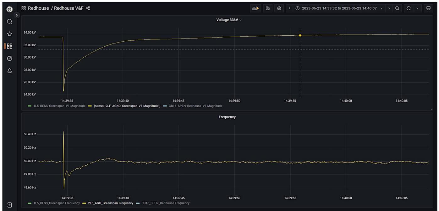
Figure 77: Redhouse GT1 and 132 kV OHL energised via the diesel generator without PoW
