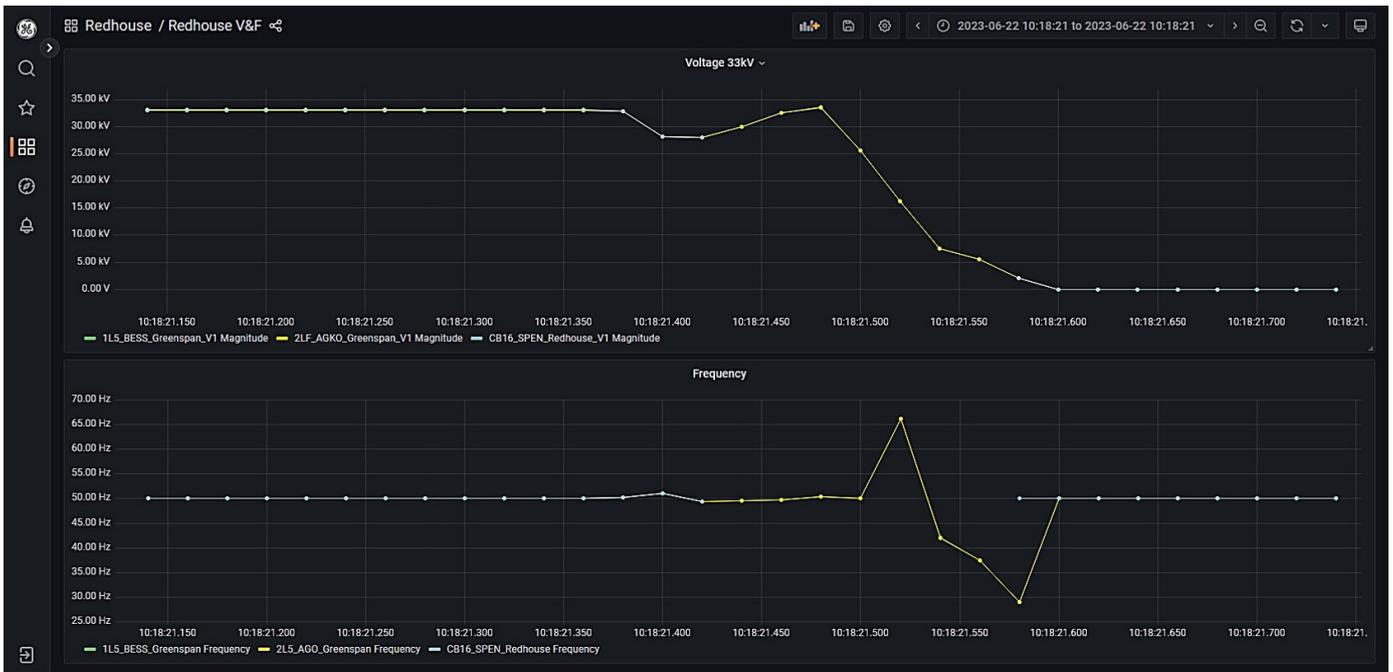
Figure 59: Chapel primary T1 and Redhouse primary T1 energised via BESS without PoW (BESS tripped)
