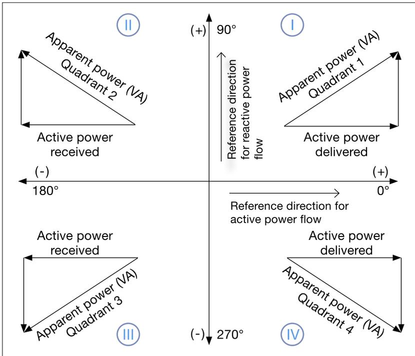
Figure 7: Four quadrants of active and reactive power
