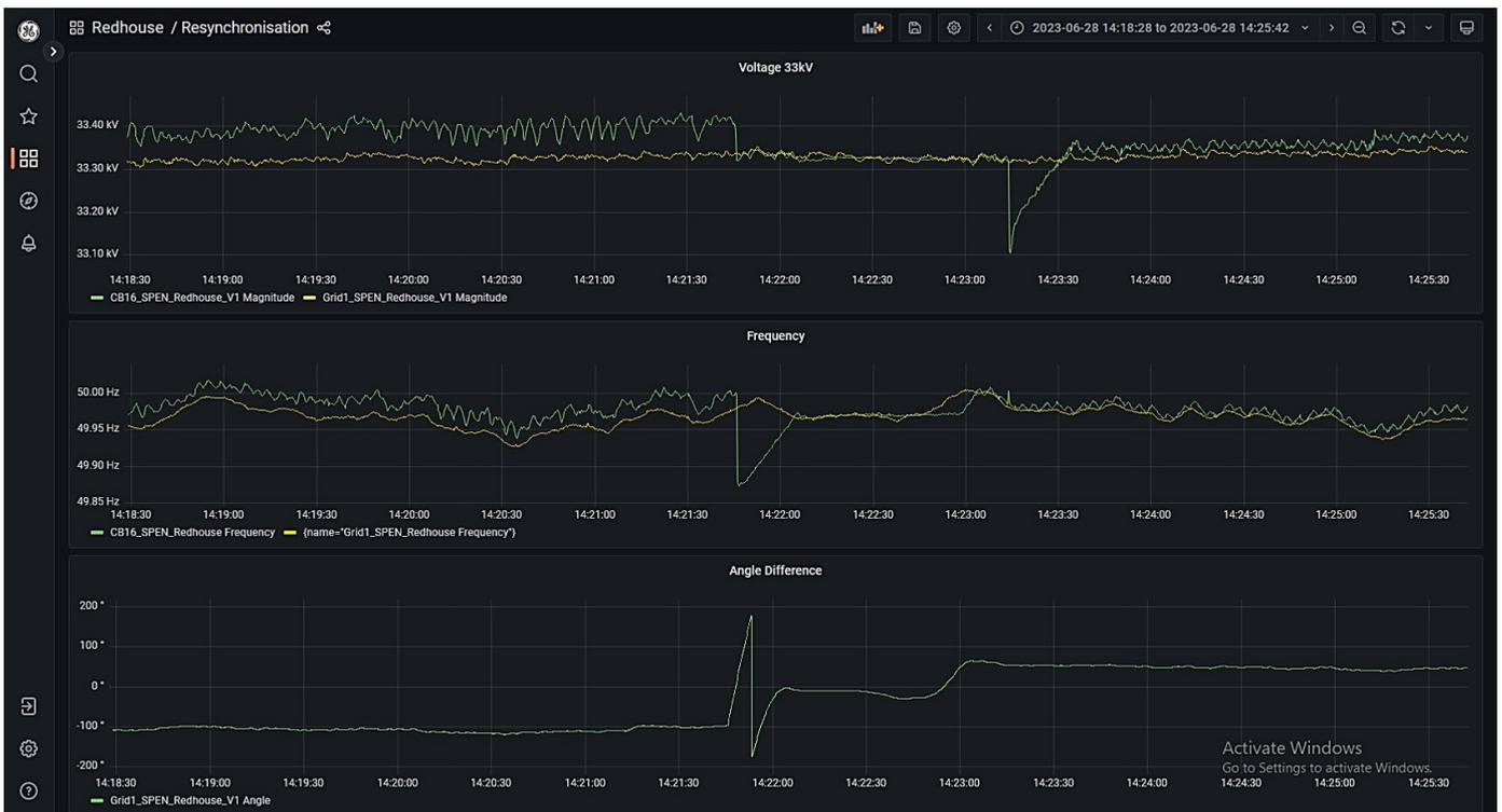
Figure 122: Voltage and frequency regulation via control of BESS prior to resynchronisation
