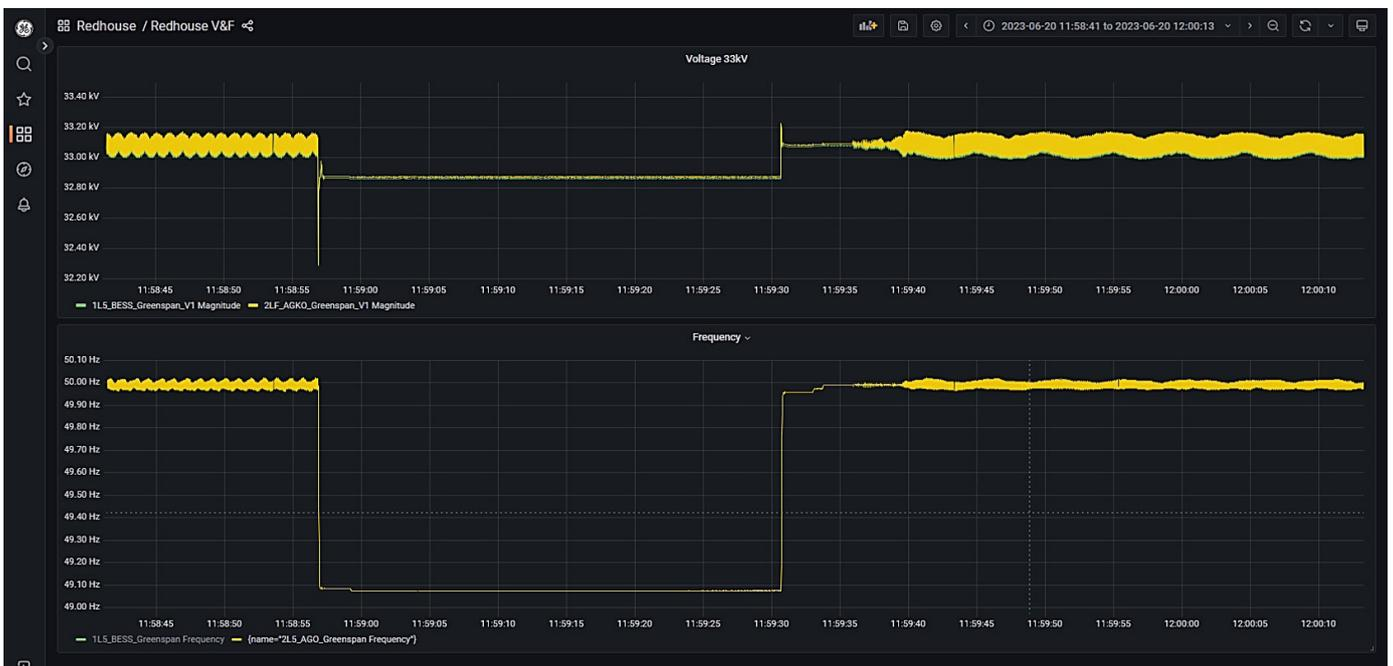
Figure 14: Grid-forming BESS voltage and frequency – 4 MW load step (4% droop)
