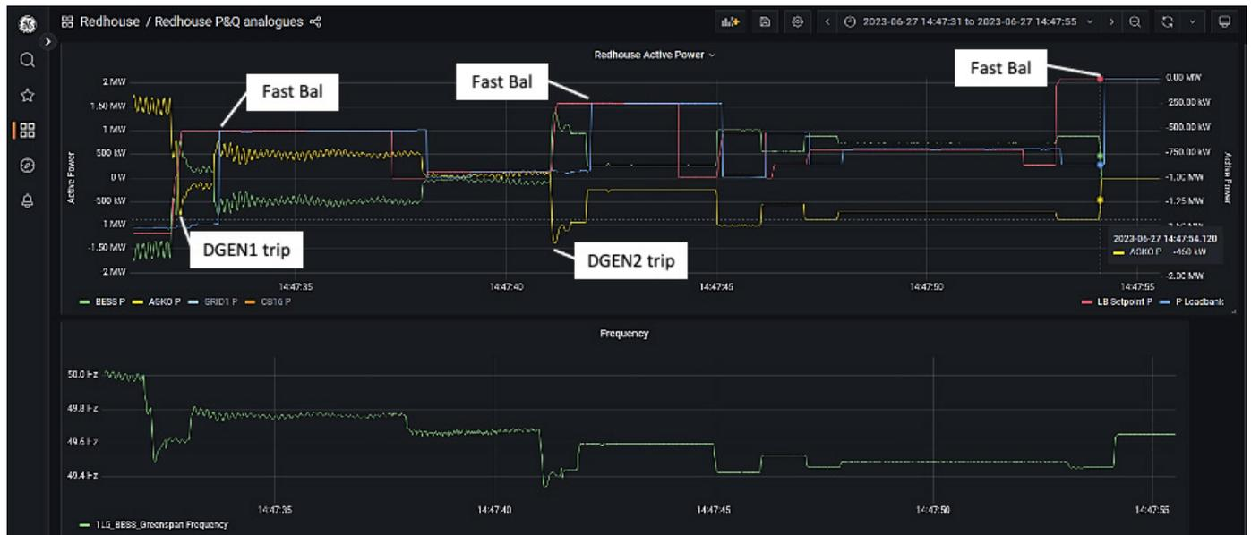
Figure 115: Diesel generator trip in two stages of 1.5 MW
