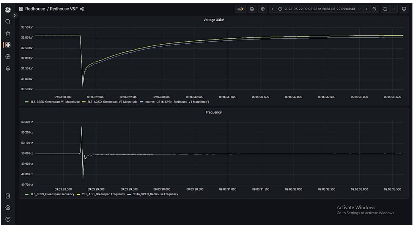
Figure 47: Chapel primary T1 energised via BESS with PoW
