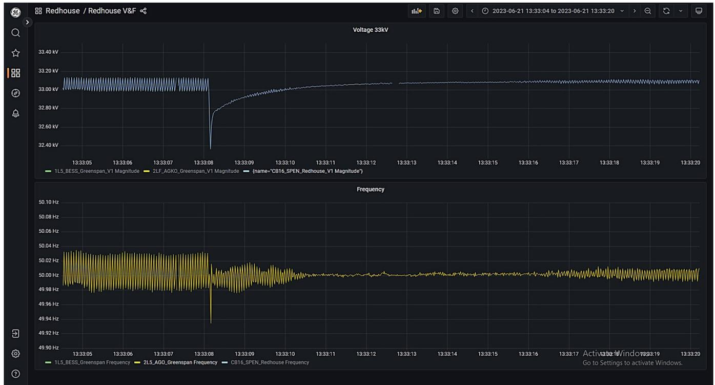
Figure 26: Chapel primary T1 energised via the diesel generator and grid-forming BESS with PoW
