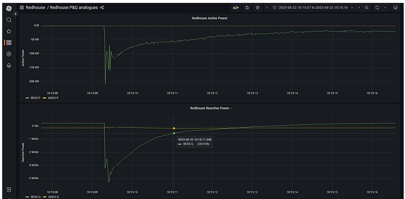
Figure 58: Chapel primary T1 and Redhouse primary T1 energised via BESS without PoW
