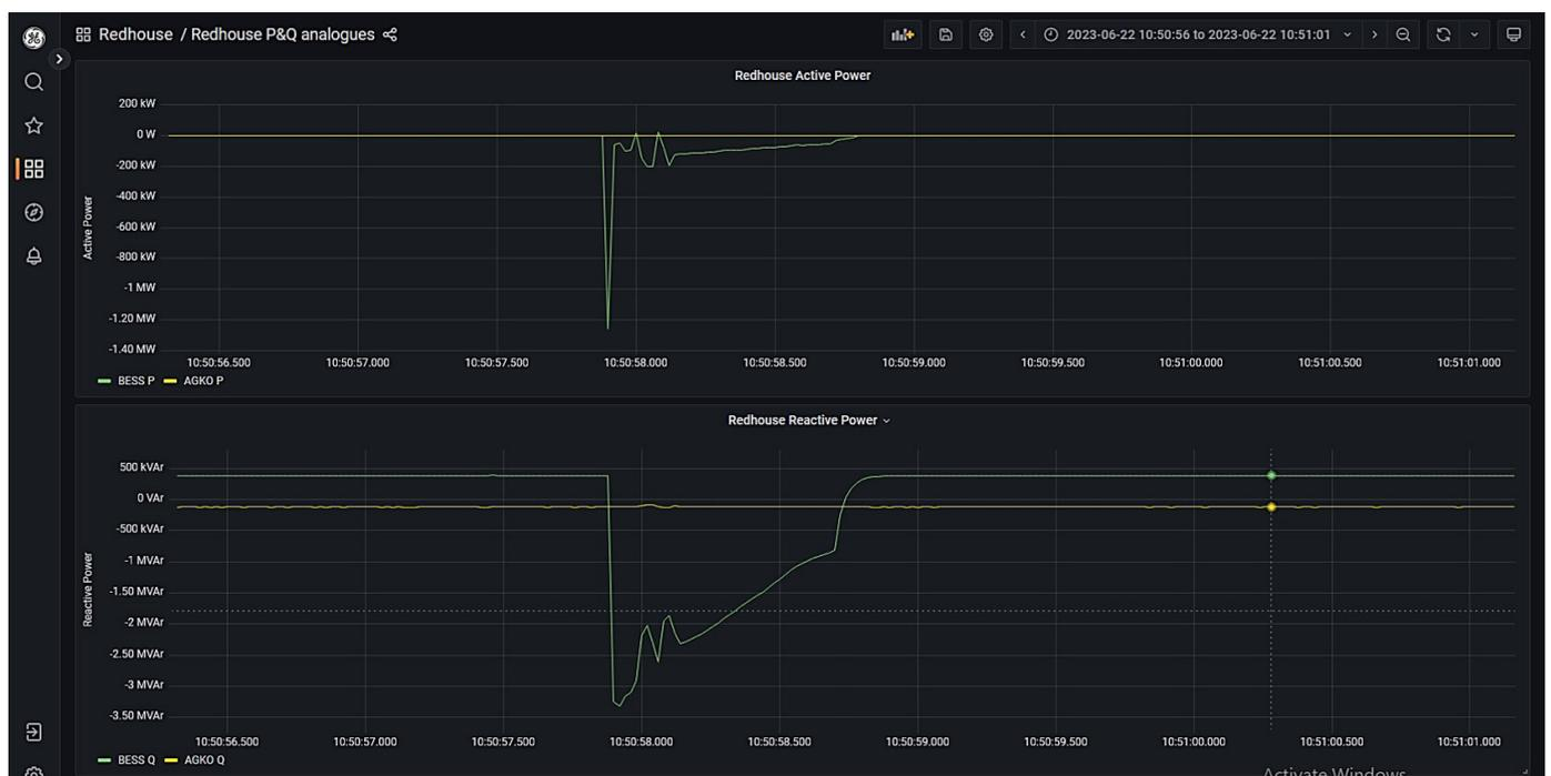
Figure 64: Energisation of Middle Balbeggie Solar transformers via BESS
