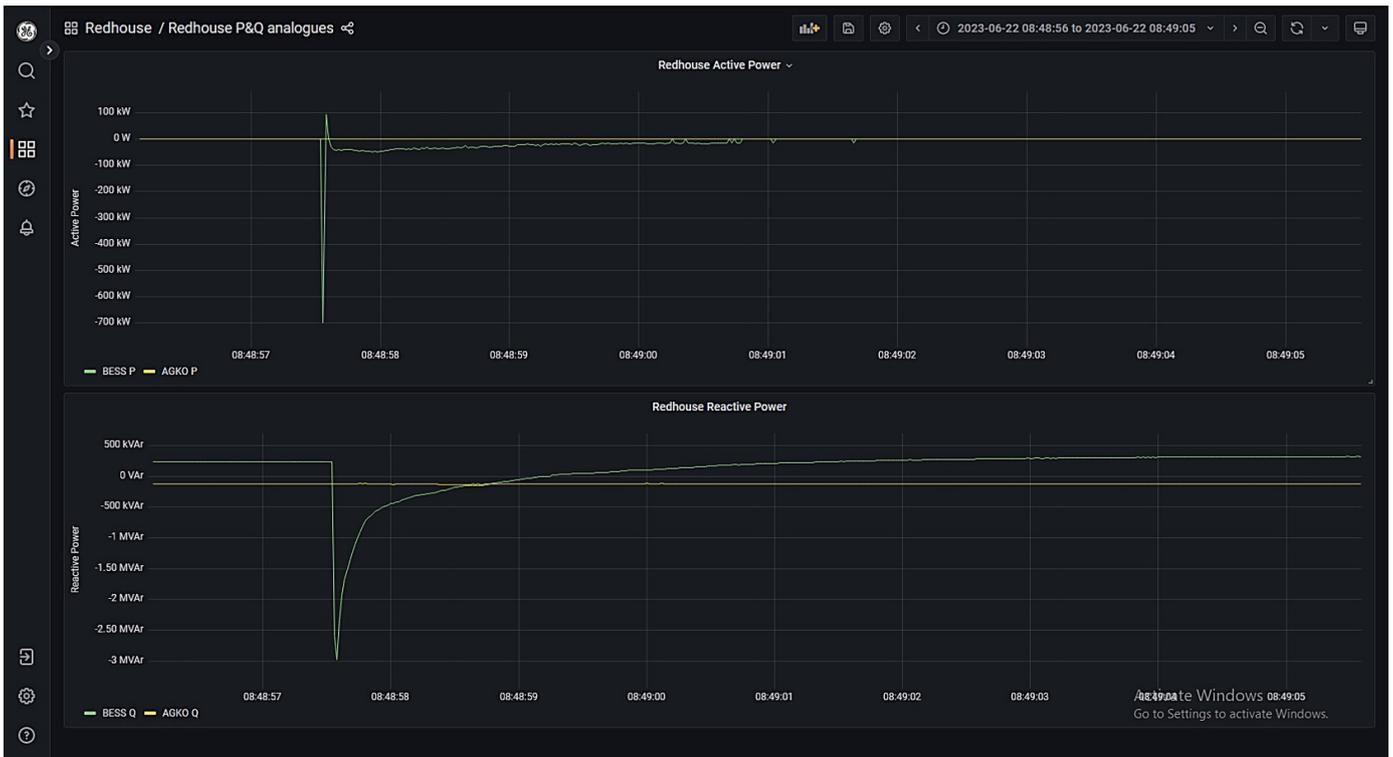
Figure 46: Chapel primary T1 energised via BESS without PoW
