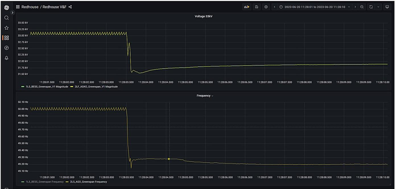
Figure 11: Grid-forming BESS and diesel generator voltage and frequency – 3.5 MW and 2.6 MVar load step (1/2)
