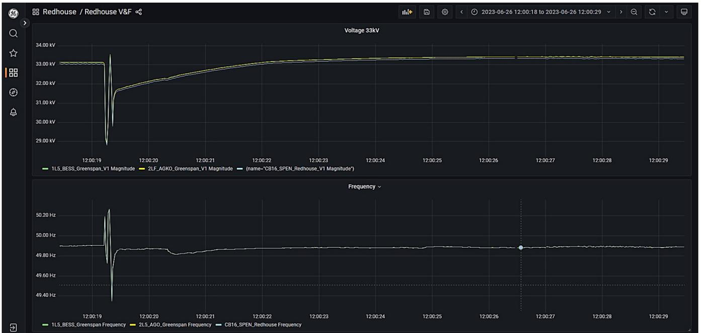
Figure 93: Redhouse GT1 and 132 kV OHL energised via the BESS and the diesel generator with PoW
