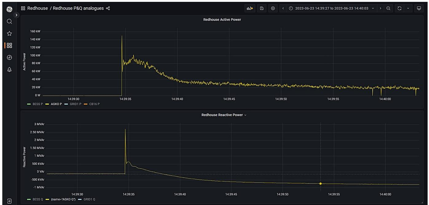
Figure 78: Redhouse GT1 and 132 kV OHL energised via the diesel generator without PoW
