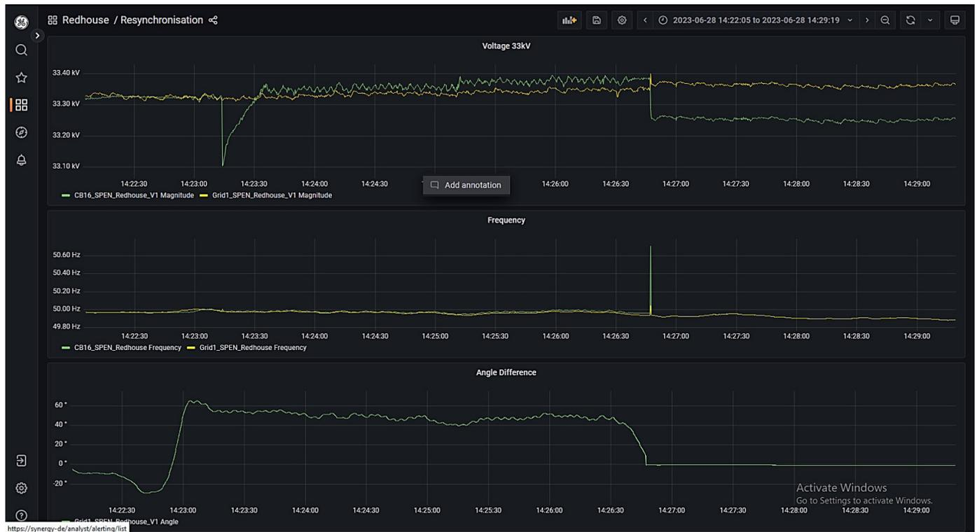
Figure 123: Resynchronisation via BESS control
