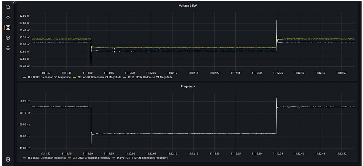
Figure 69: 4 MW load step applied to trial network with BESS and MBS connected
