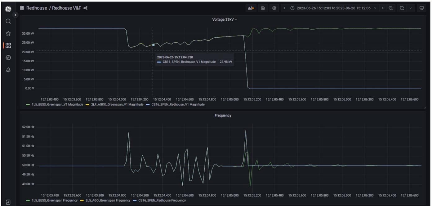
Figure 101: Redhouse GT1 and 132 kV OHL energisation attempt via the BESS without PoW – protection tripped
