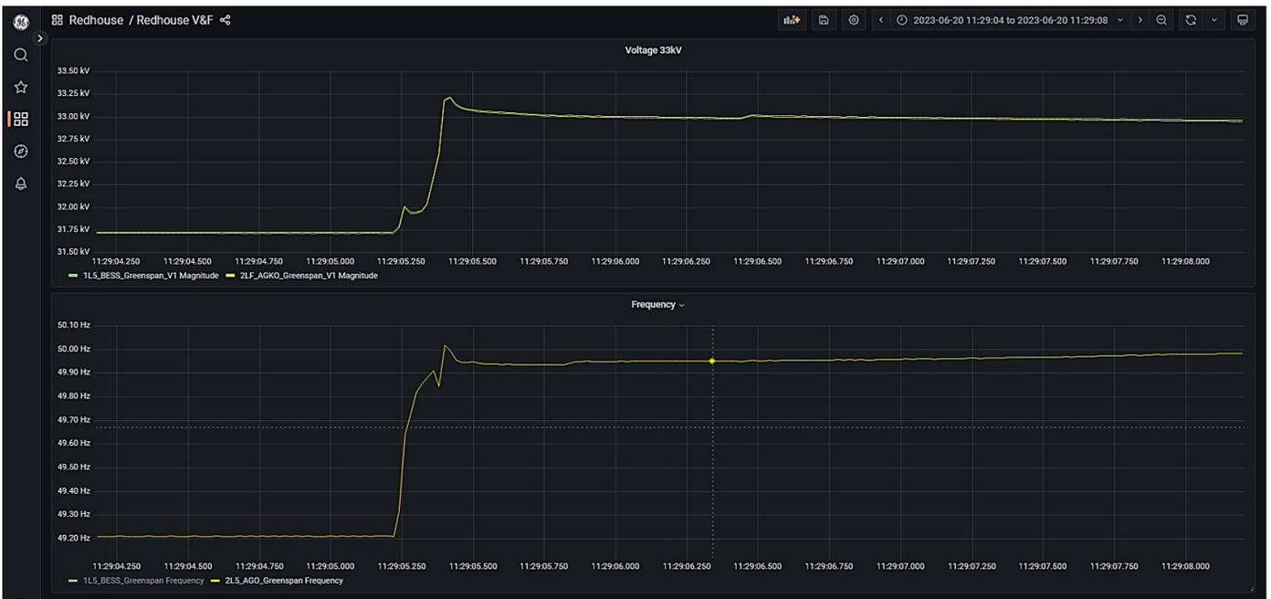
Figure 12: Grid-forming BESS and diesel generator voltage and frequency – 3.5 MW and 2.6 MVar load step (2/2)
