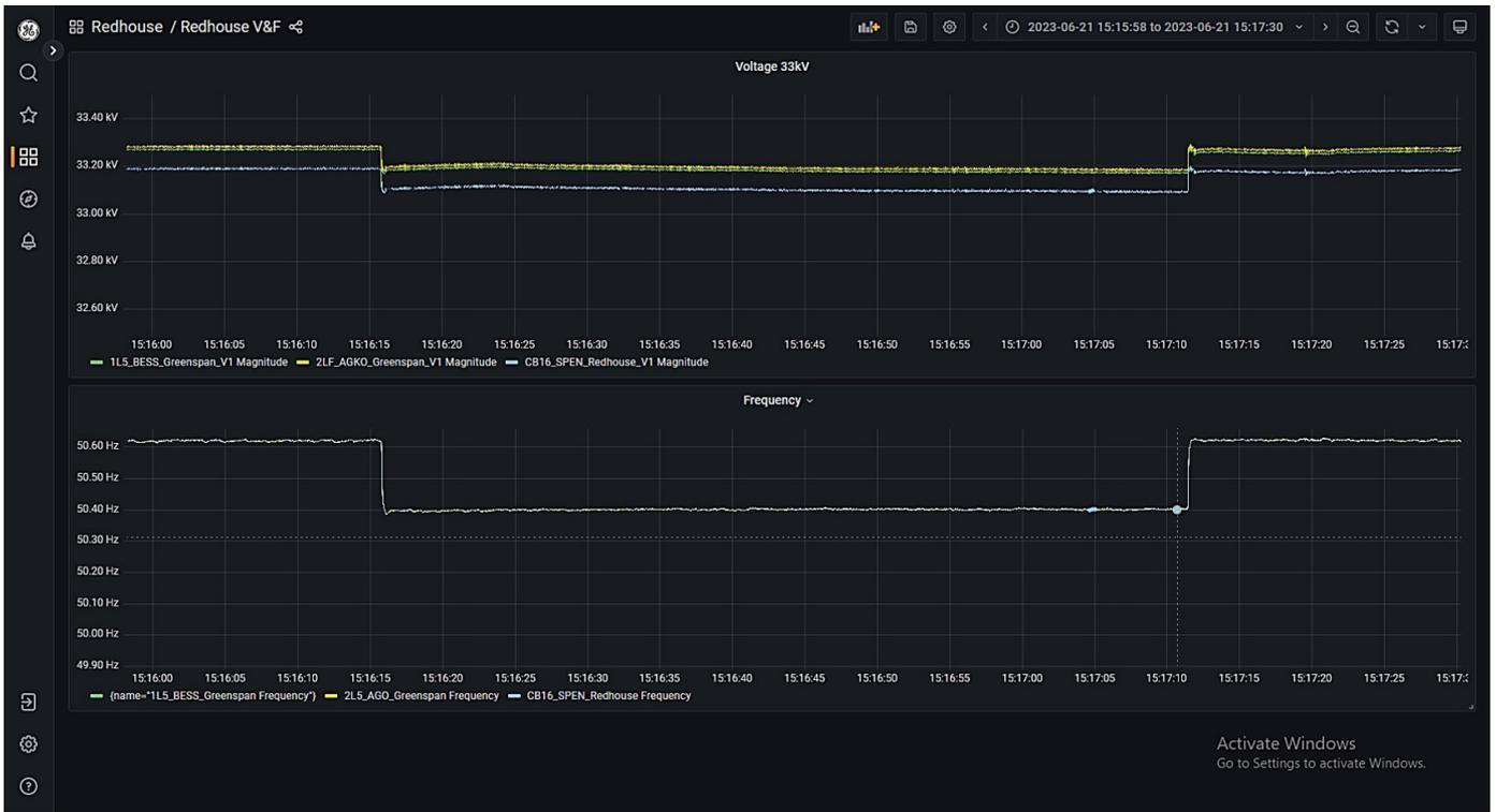
Figure 39: 1 MW load step applied to trial network with diesel generator, BESS and MBS connected
