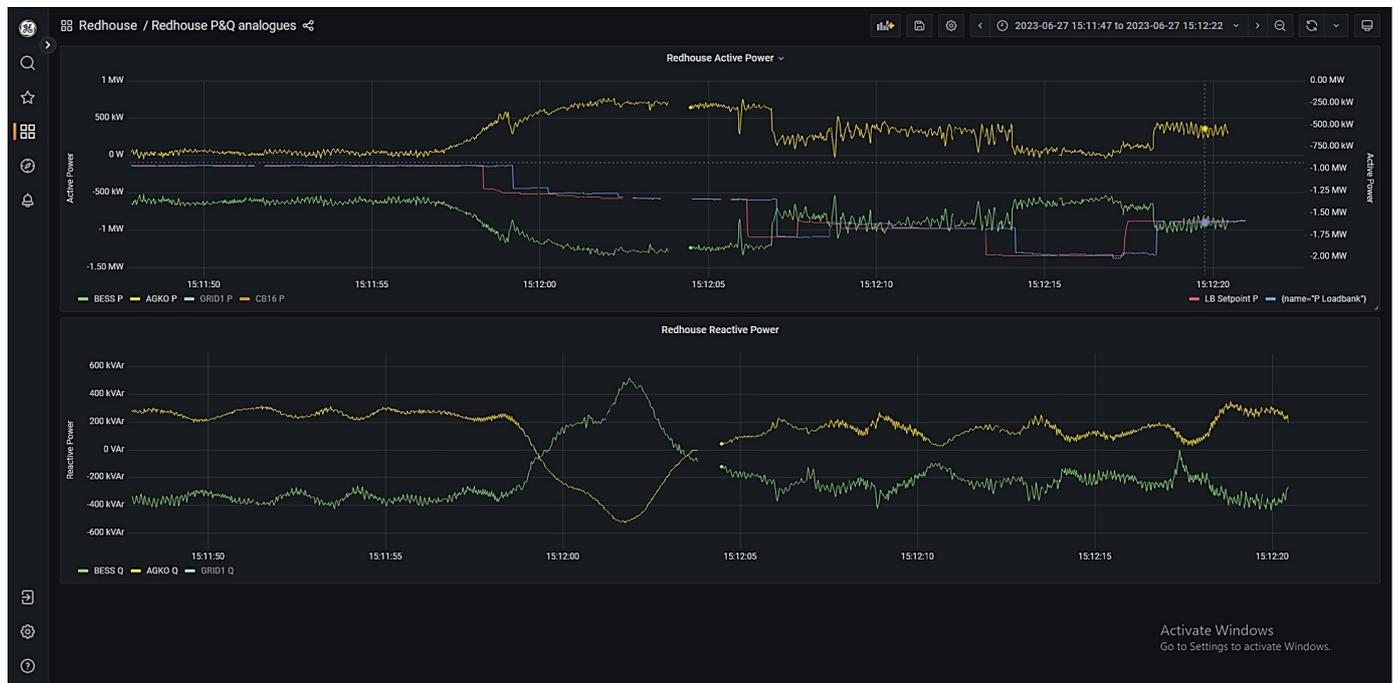
Figure 117: Diesel generator step from 1 MW to 2 MW
