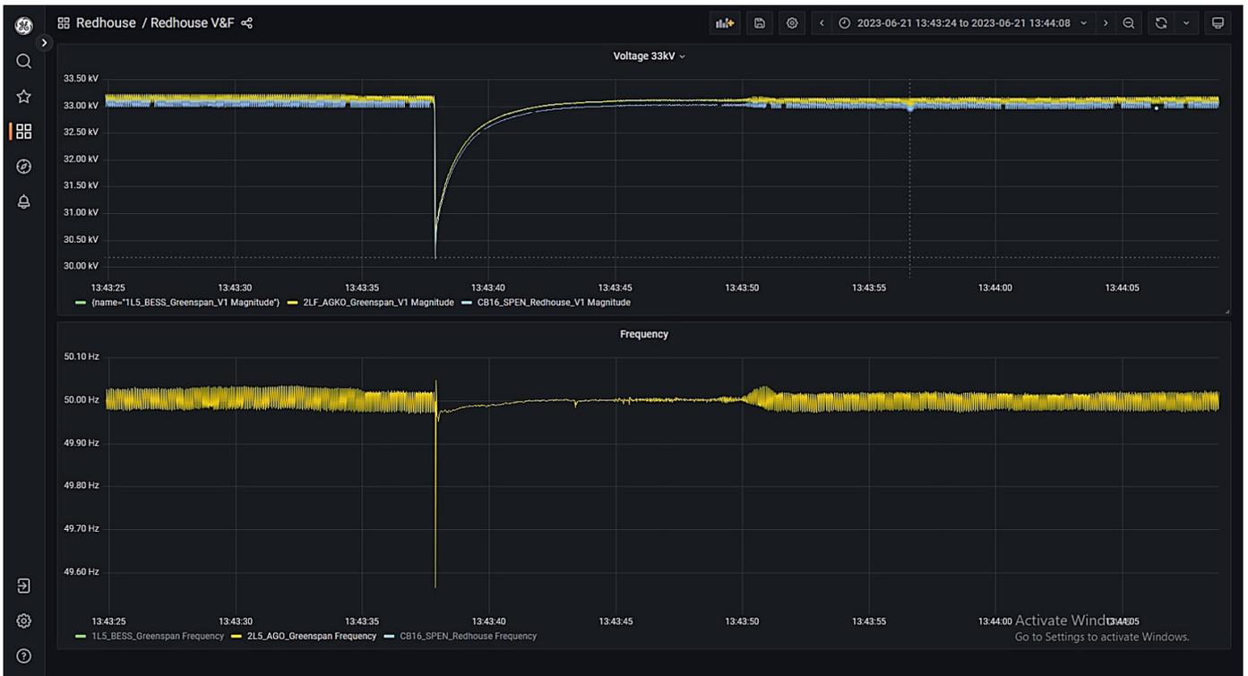
Figure 27: Redhouse primary T1 energised via the diesel generator and grid-forming BESS without PoW
