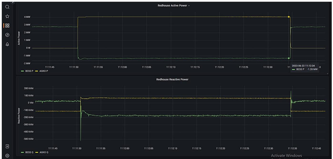
Figure 70: 4 MW load step applied to trial network with BESS and MBS connected
