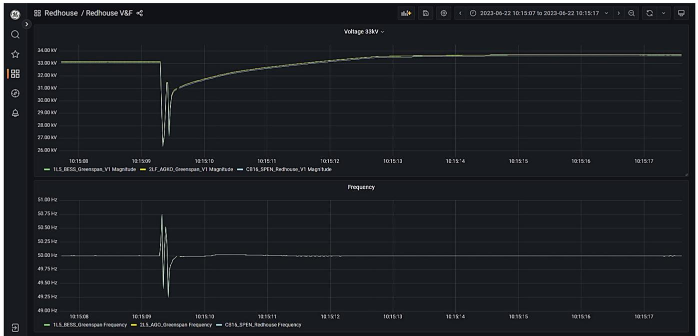
Figure 57: Chapel primary T1 and Redhouse primary T1 energised via BESS without PoW
