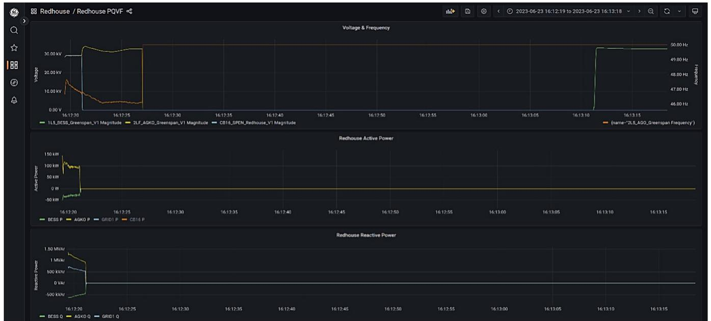
Figure 92: Diesel generator trip up to BESS automatic re-energisation (16:12:21–16:13:12)
