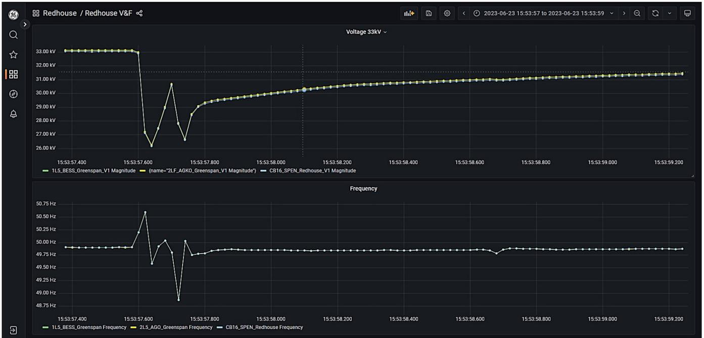
Figure 81: Redhouse GT1 energised via the BESS and diesel generator without PoW
