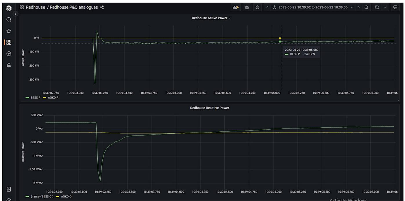
Figure 62: Chapel primary T1 and Redhouse primary T1 energised via BESS with PoW
