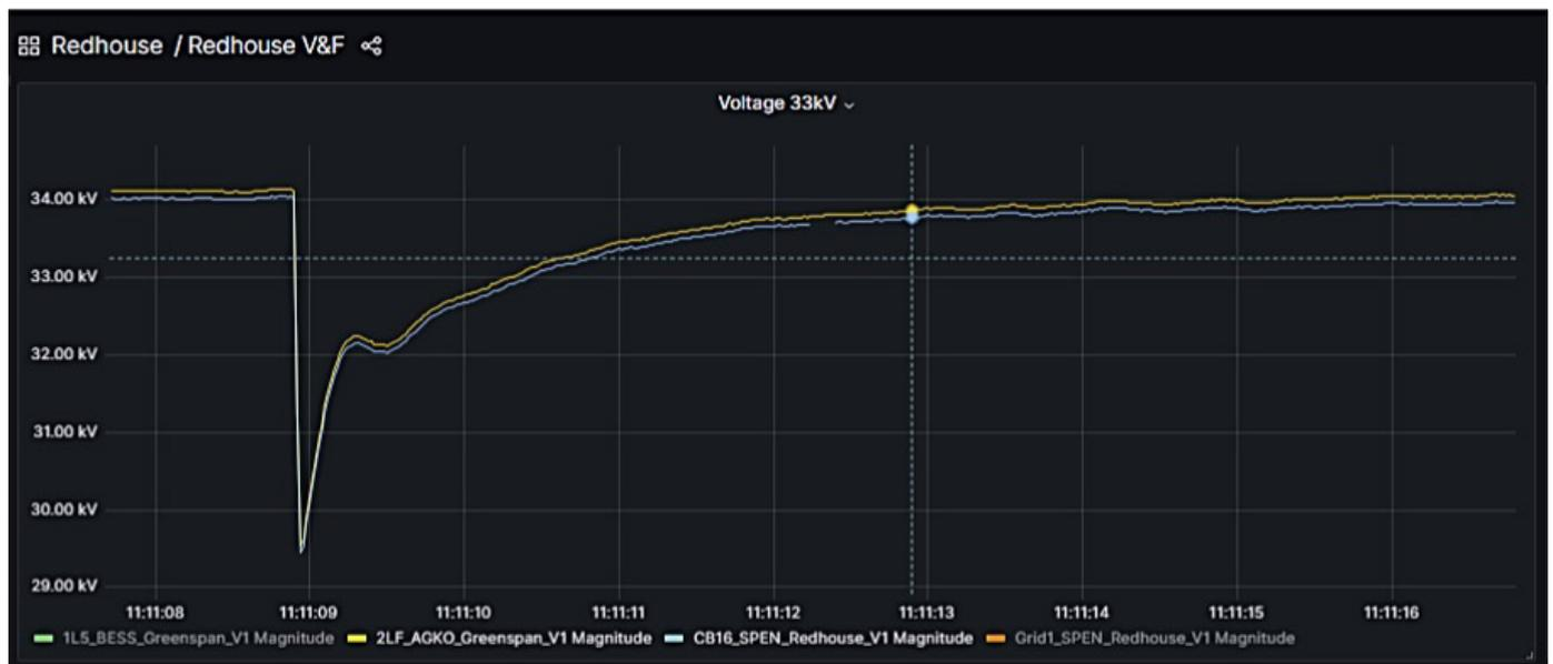
Figure 20: Chapel primary T1 energised via the diesel generator with PoW
