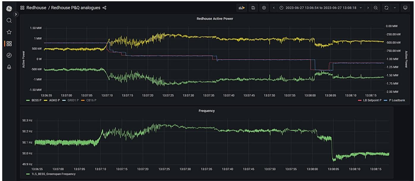
Figure 113: Diesel generator step from 1 MW to 2 MW
