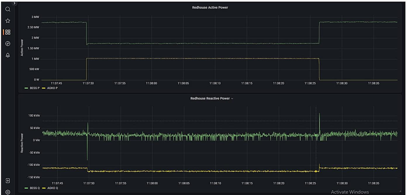
Figure 68: 1 MW load step applied to trial network with BESS and MBS connected
