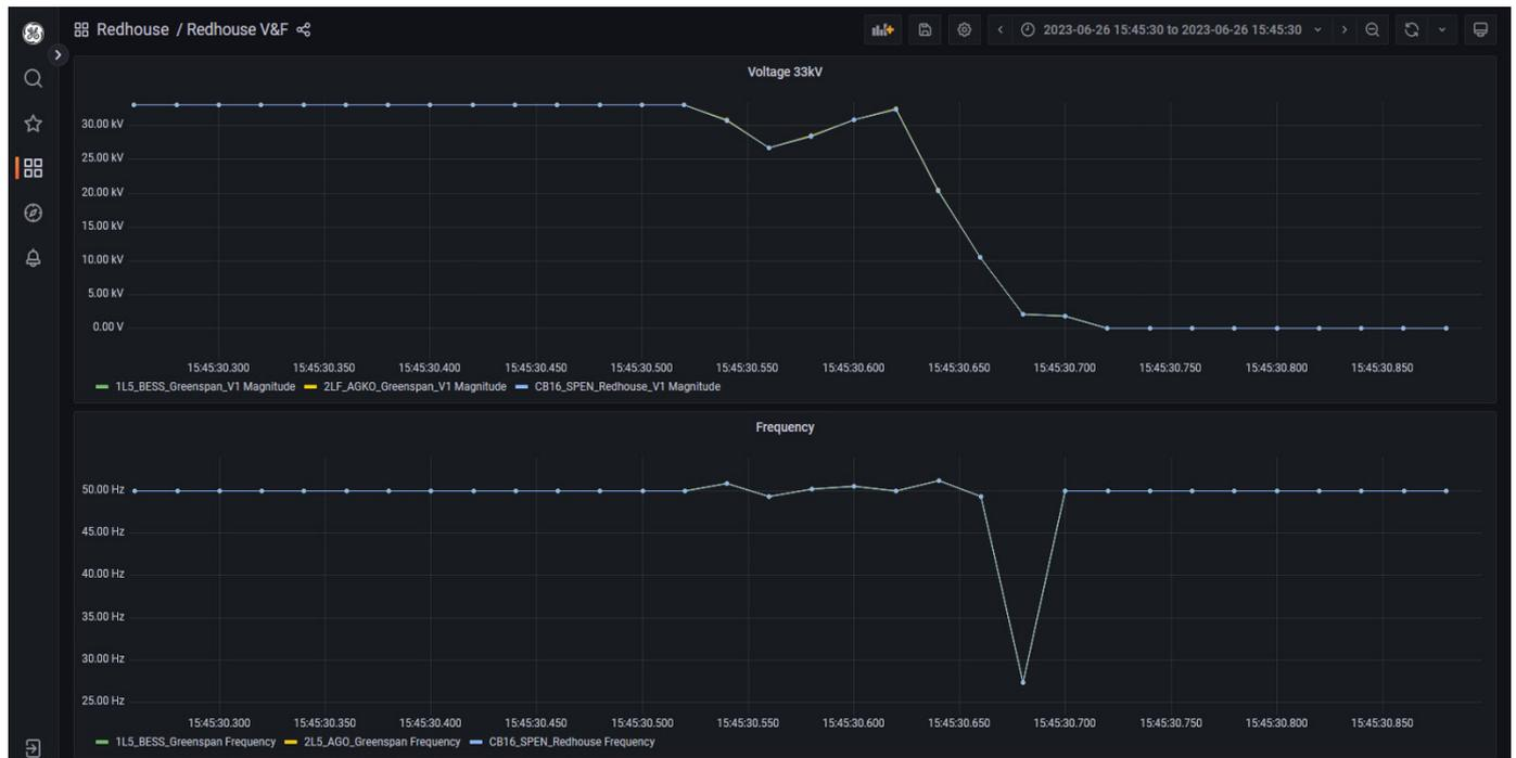
Figure 103: Redhouse GT1 and 132 kV OHL energisation attempt via the BESS without PoW – protection tripped
