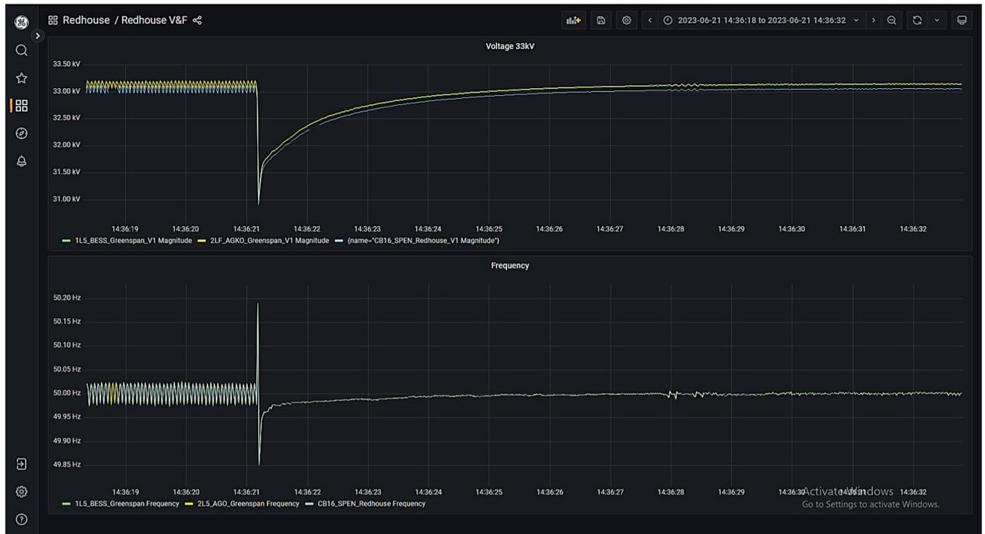
Figure 33: Chapel primary T1 and Redhouse primary T1 energised via the diesel generator and grid-forming BESS with PoW
