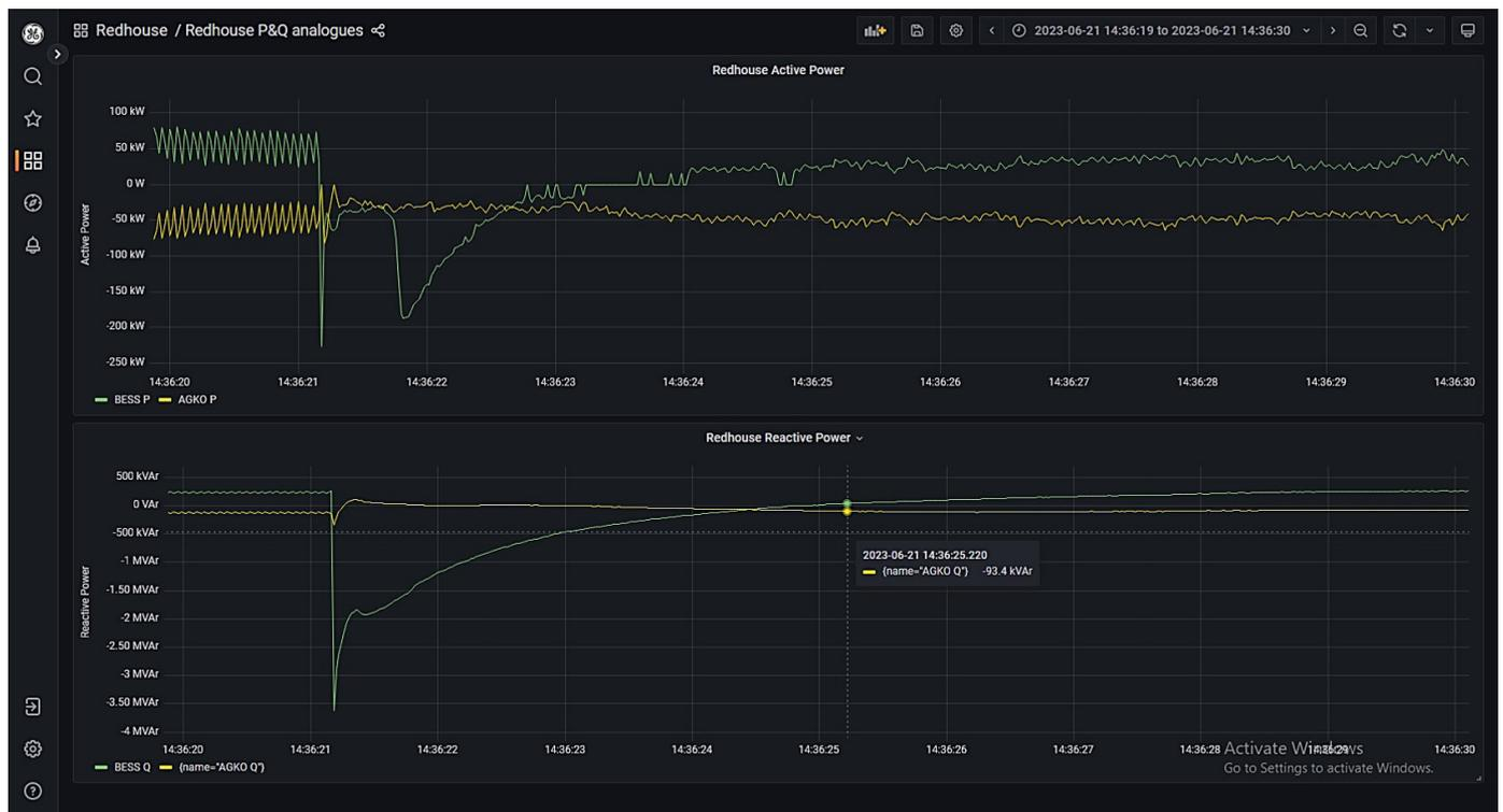
Figure 34: Chapel primary T1 and Redhouse primary T1 energised via the diesel generator and grid-forming BESS with PoW
