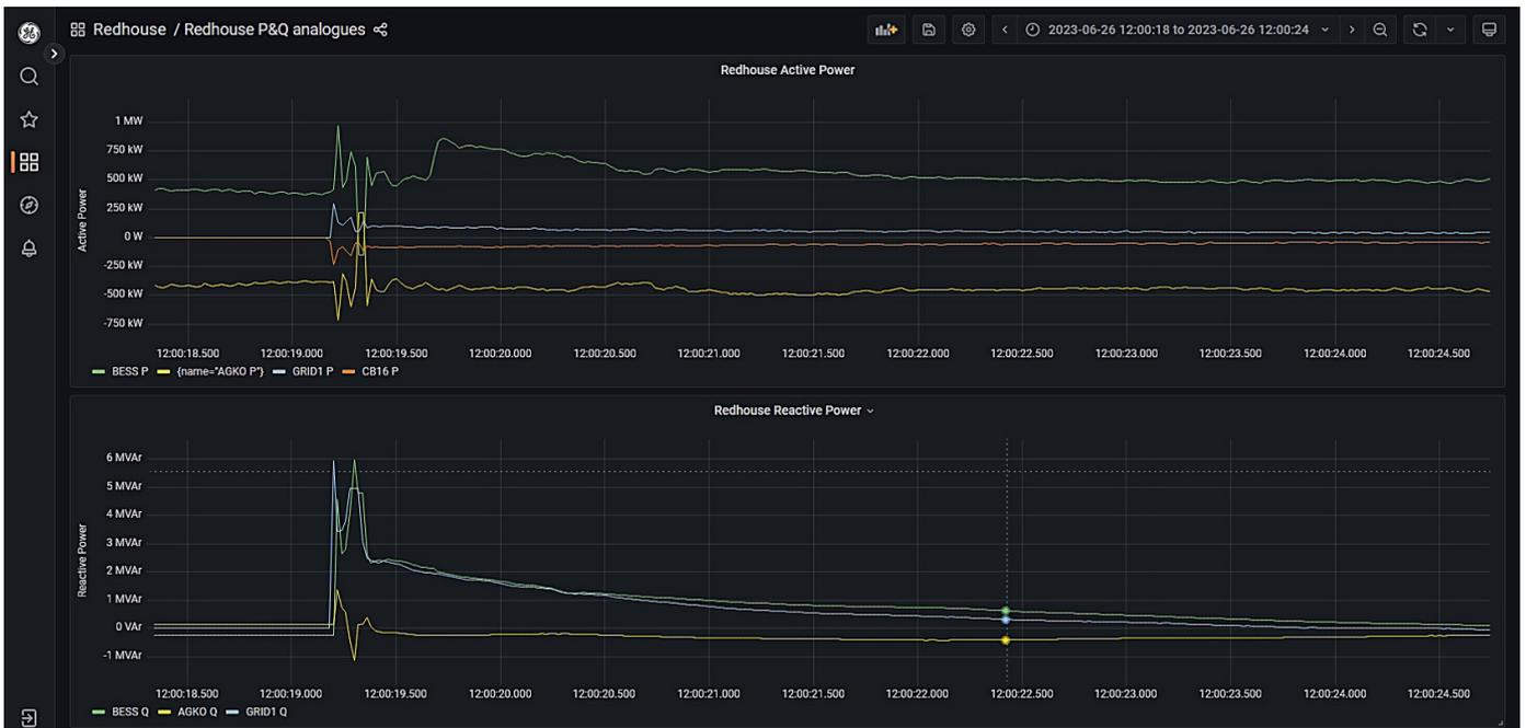
Figure 94: Redhouse GT1 and 132 kV OHL energised via the BESS and the diesel generator with PoW
