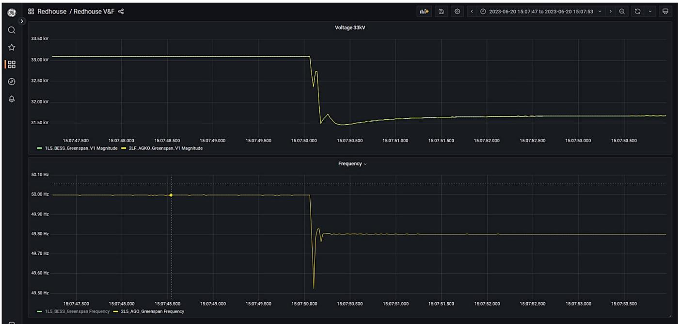
Figure 17: Grid-forming BESS voltage and frequency – 3.3 MW and 2.7 MVar load step (1/2)
