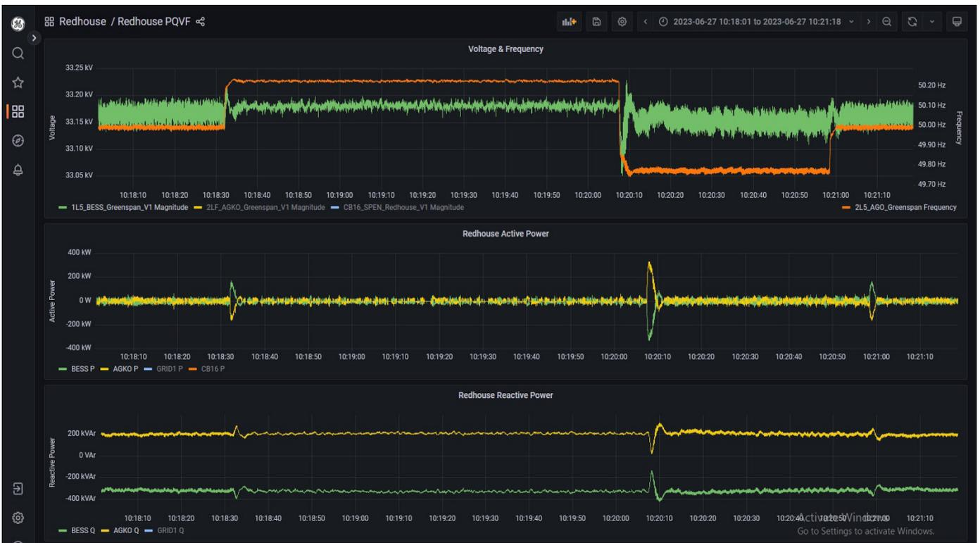
Figure 109: Testing DRZC control of BESS real power setpoints
