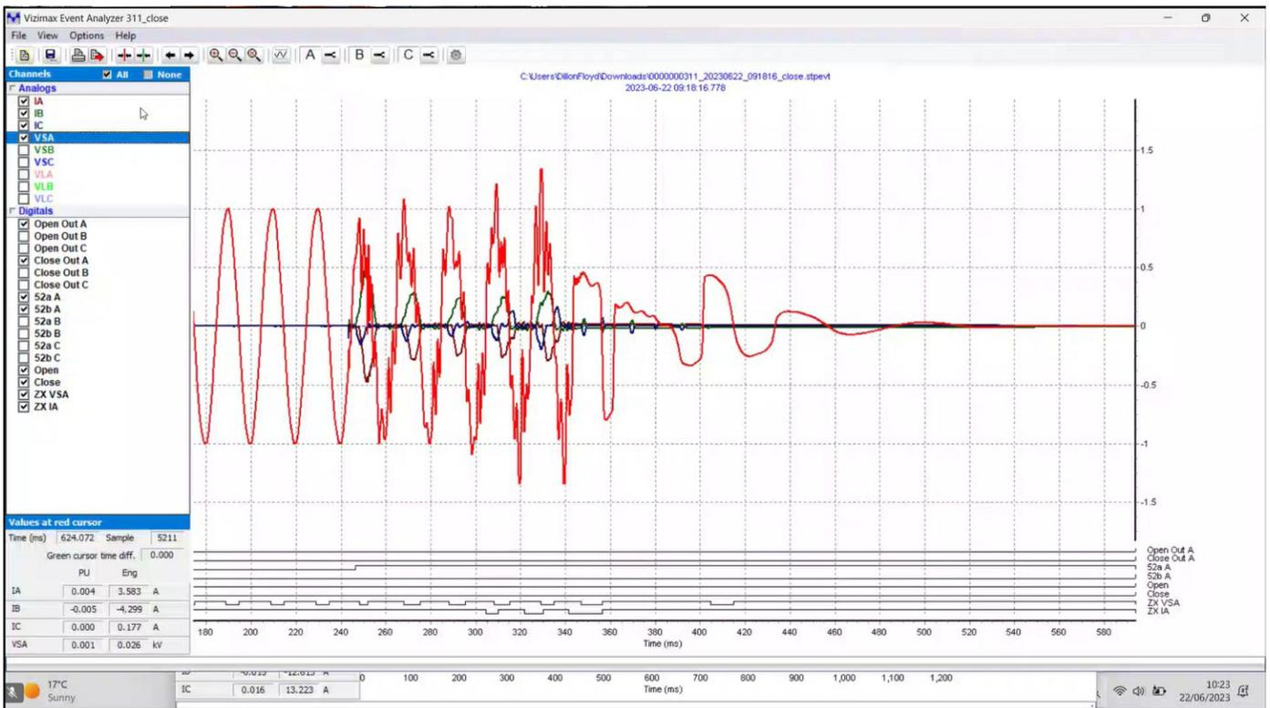
Figure 60: Voltage and current signals from PoW relay, failed Chapel and Redhouse energisation
