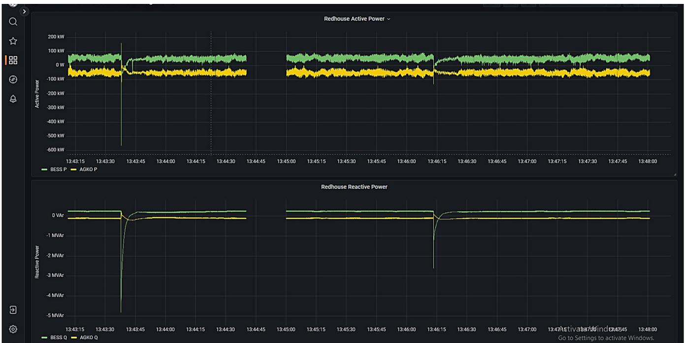
Figure 28: Redhouse primary T1 energised via the diesel generator and grid-forming BESS without PoW
