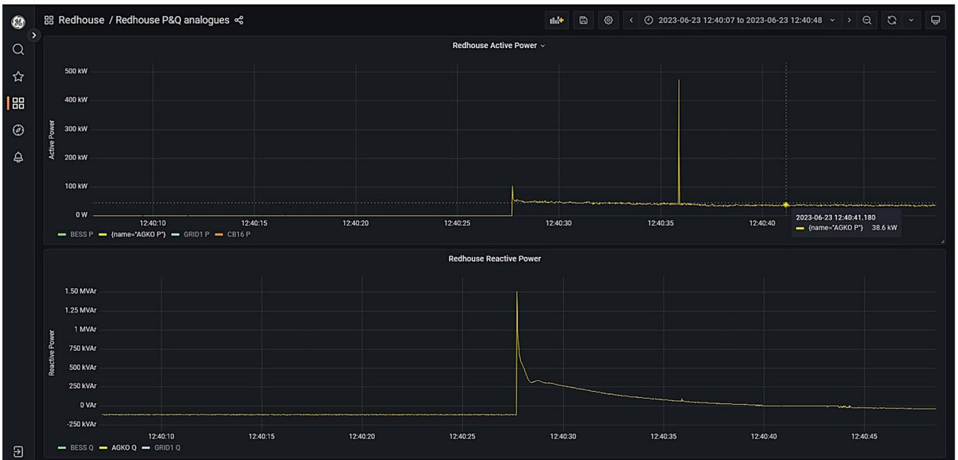
Figure 73: Redhouse GT1 energised via the diesel generator without PoW
