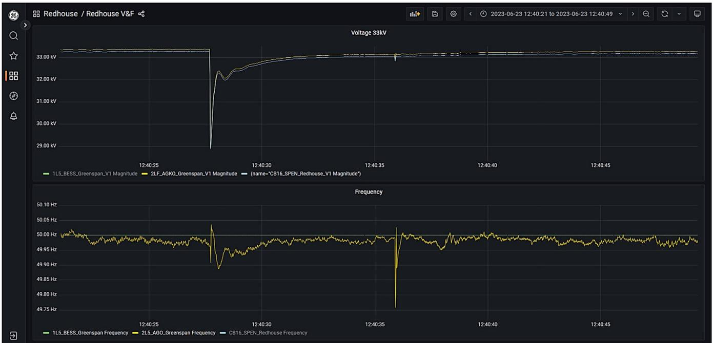
Figure 72: Redhouse GT1 energised via the diesel generator without PoW
