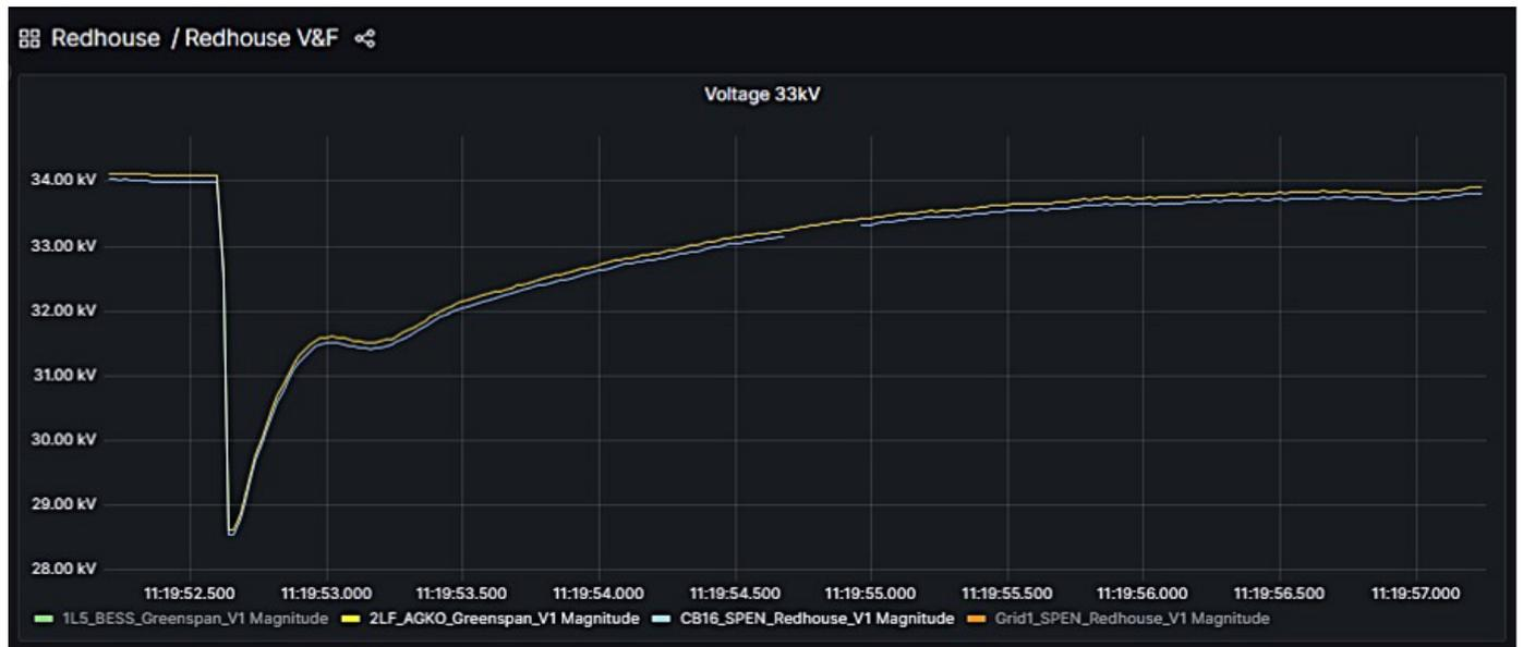
Figure 21: Chapel primary T1 energised via the diesel generator without PoW
