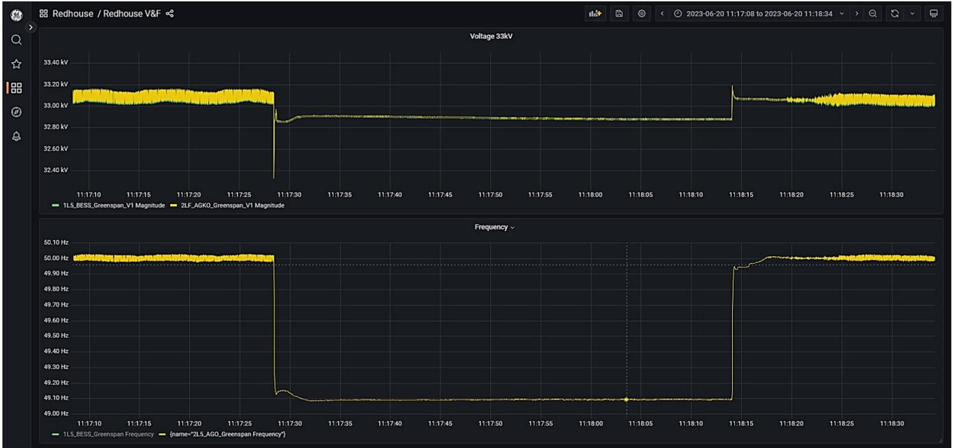
Figure 10: Grid-forming BESS and diesel generator voltage and frequency – 2.5 MW load step
