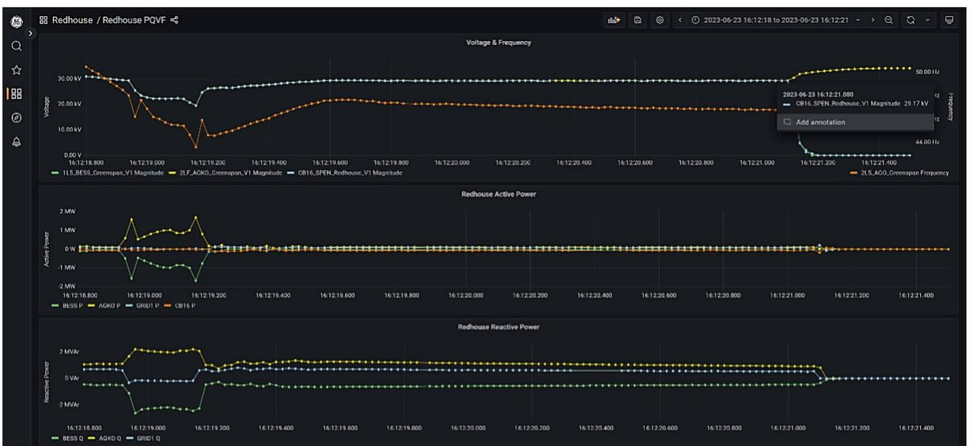
Figure 91: Stabilisation and decline of frequency up to underfrequency tripping
