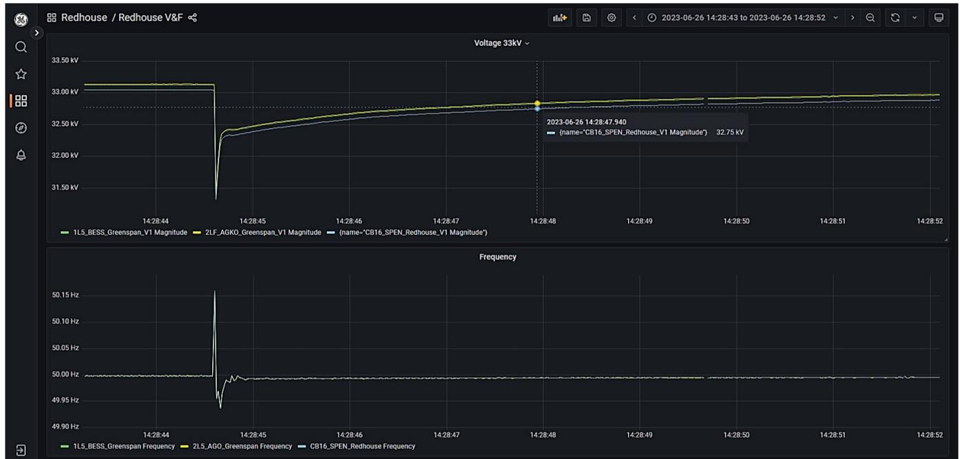
Figure 95: Redhouse GT1 energised via the BESS with PoW
