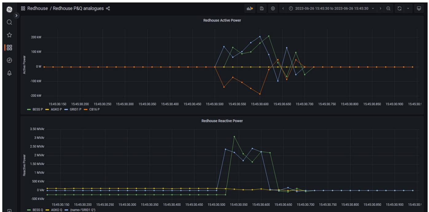
Figure 104: Redhouse GT1 and 132 kV OHL energisation attempt via the BESS without PoW – protection tripped
