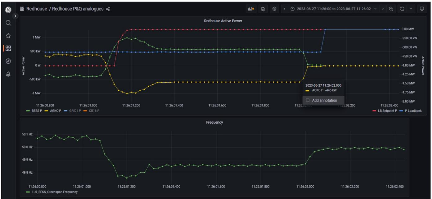
Figure 112: Initial fast balancing test via diesel generator 1 MW trip
