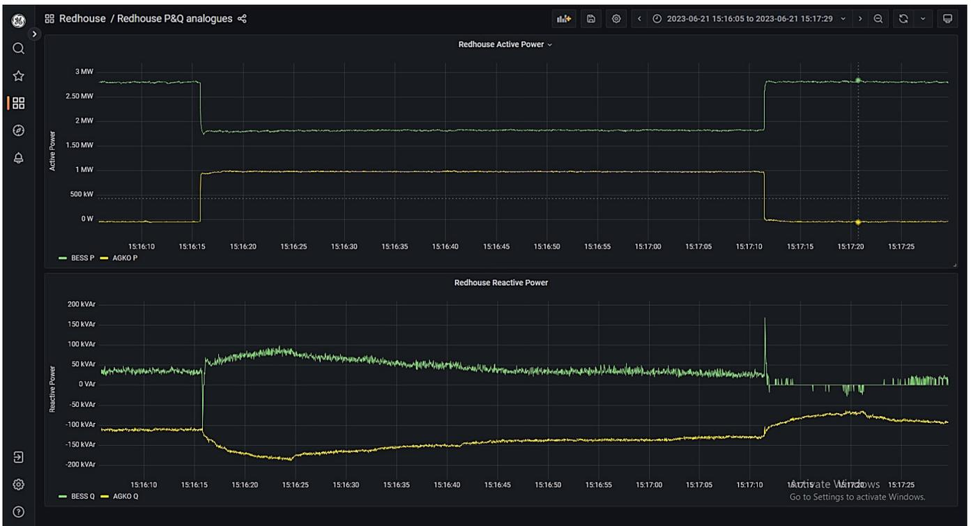
Figure 40: 1 MW load step applied to trial network with diesel generator, BESS and MBS connected
