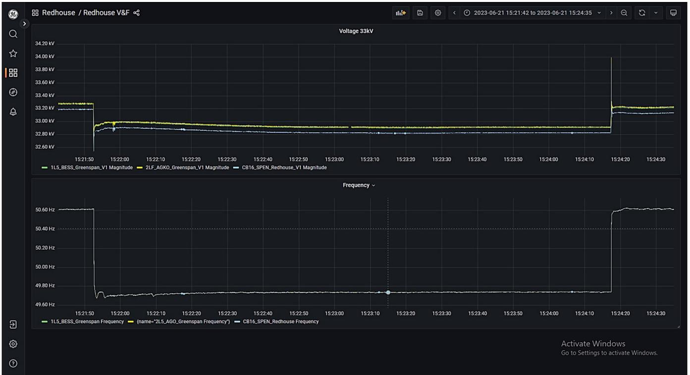
Figure 43: 4 MW load step applied to trial network with diesel generator, BESS and MBS connected
