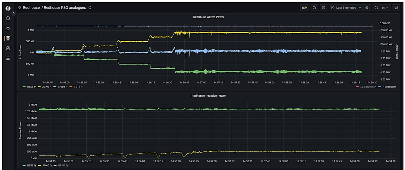
Figure 125: Diesel generator power steps while D-VPP mode is active with setpoint of 0 MW
