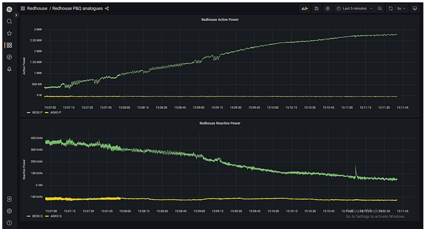
Figure 38: MBS output ramping up to ~3 MW
