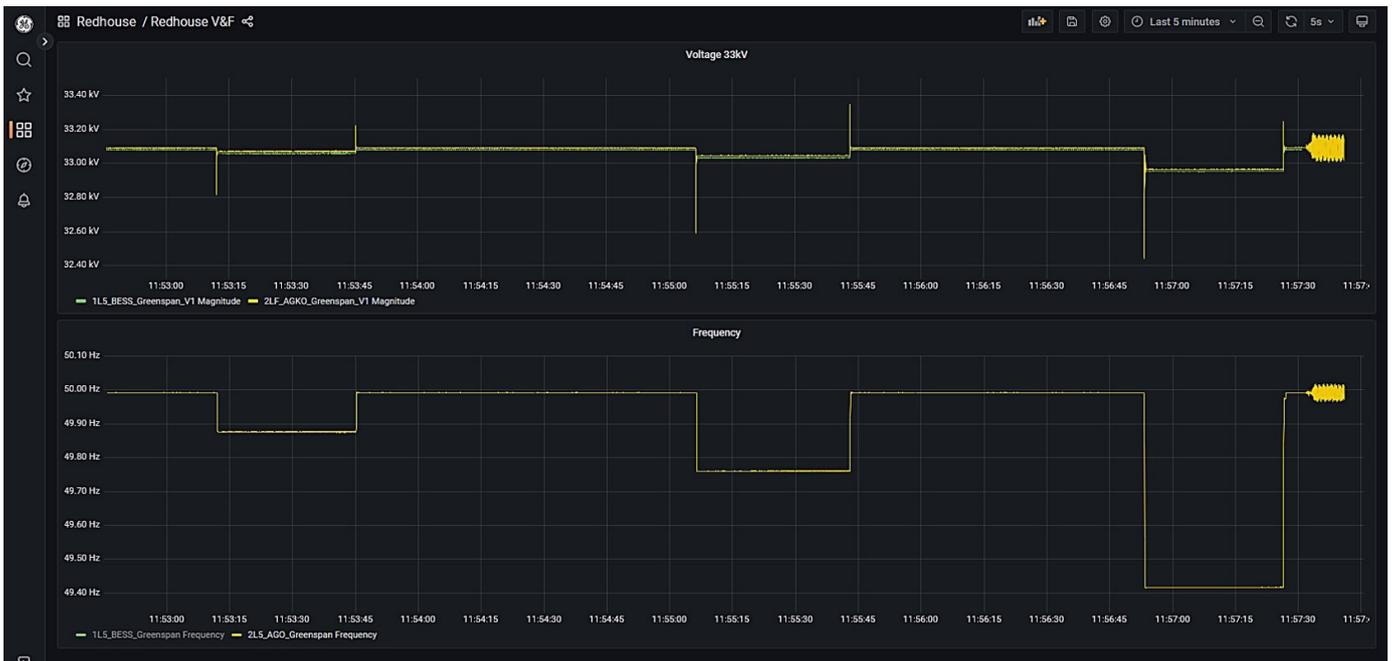
Figure 13: Grid-forming BESS voltage and frequency – 0.5 MW, 1 MW and 2 MW load steps (4% droop)
