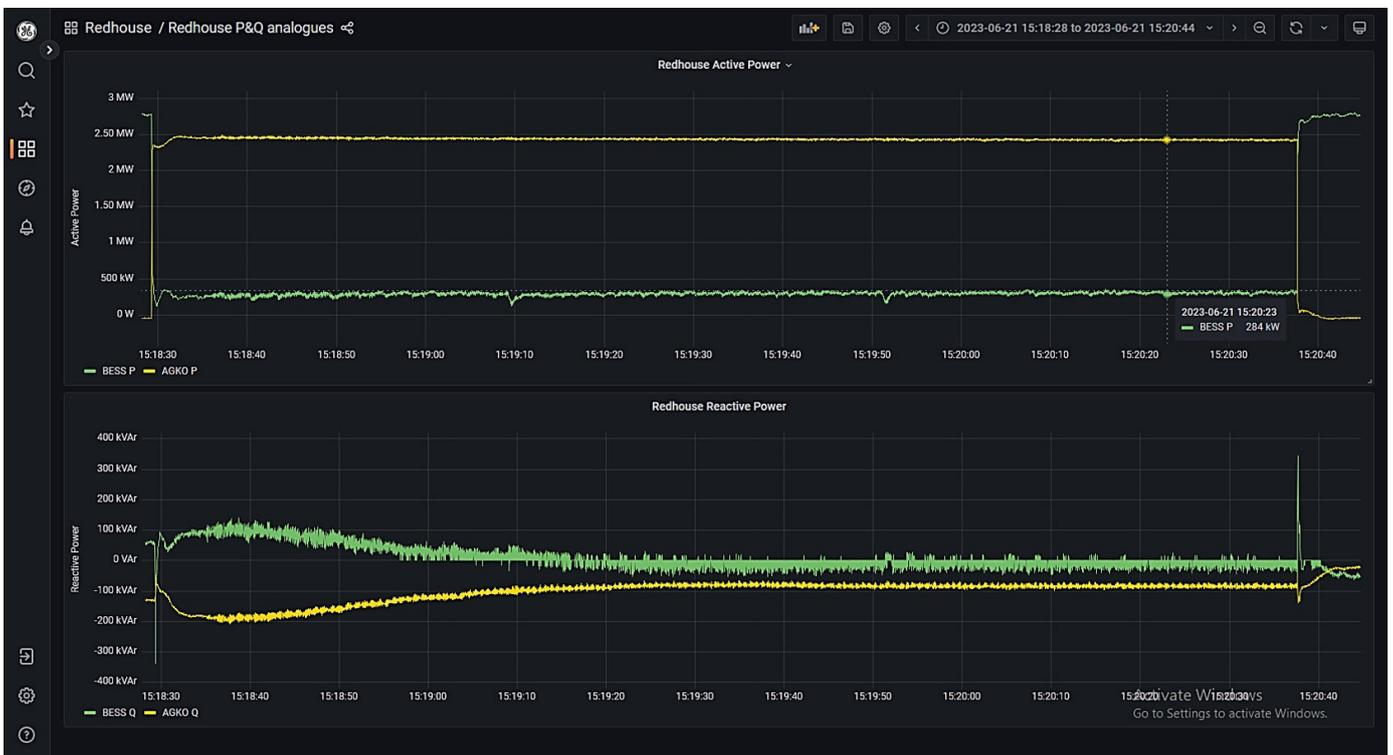
Figure 42: 2.5 MW load step applied to trial network with diesel generator, BESS and MBS connected
