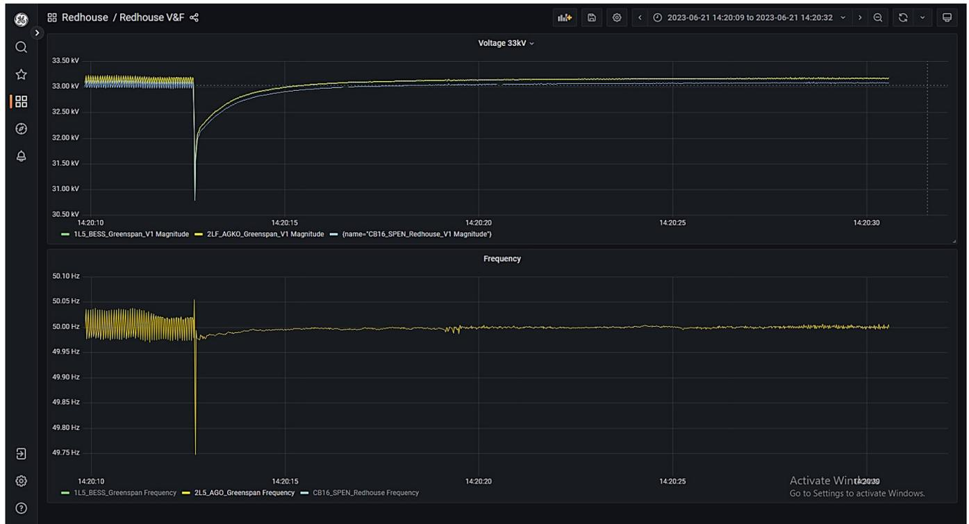
Figure 31: Chapel primary T1 and Redhouse primary T1 energised via the diesel generator and grid-forming BESS without PoW
