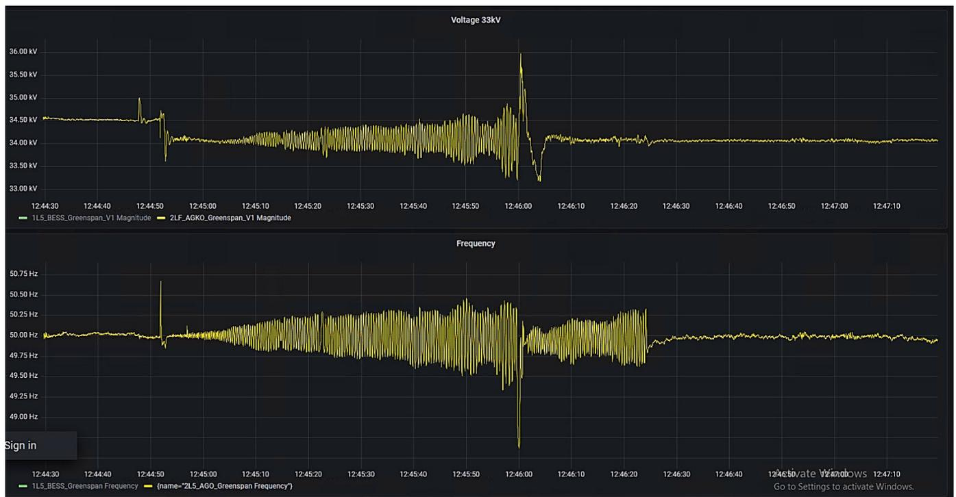
Figure 5: Grid-following BESS synchronised with diesel generator
