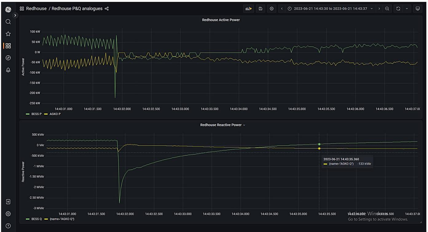
Figure 36: Chapel primary T1 and Redhouse primary T1 energised via the diesel generator and grid-forming BESS with PoW (updated operation time setting applied)
