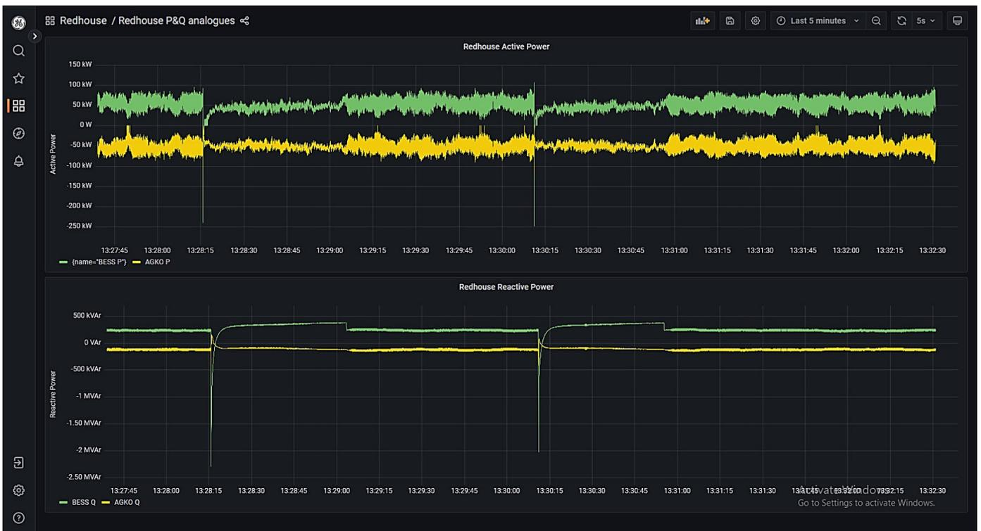
Figure 25: Chapel primary T1 energised via the diesel generator and grid-forming BESS without PoW
