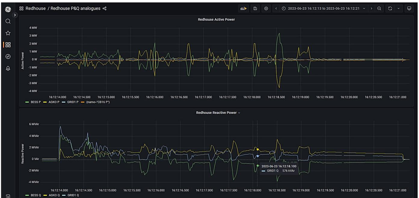
Figure 85: Redhouse GT1 and 132 kV OHL energisation attempt via the BESS and the diesel generator, instability led to trip
