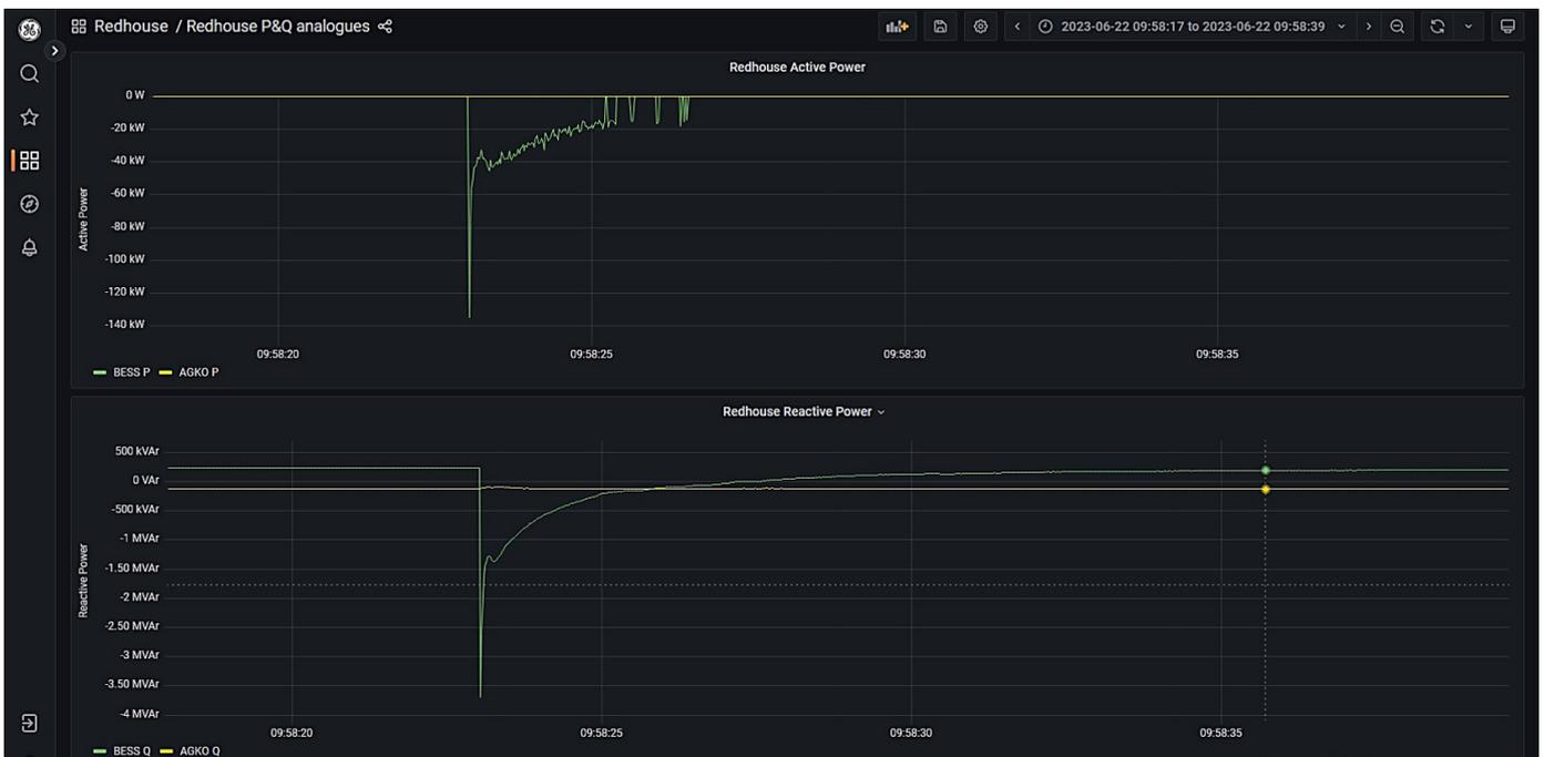
Figure 54: Redhouse primary T1 energised via BESS without PoW
