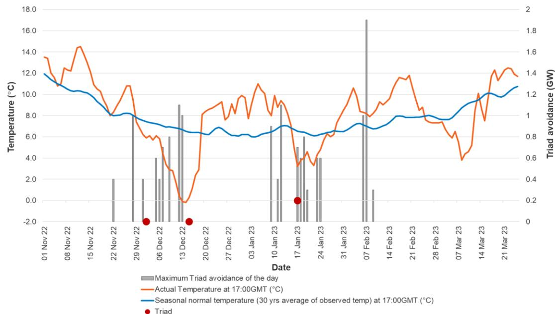
Figure 5: Daily actual temperature for winter 2022/2023 and seasonal normal temperature alongside the date of the three triads (three red dots). Note that the triad avoidance is the maximum on each day.
