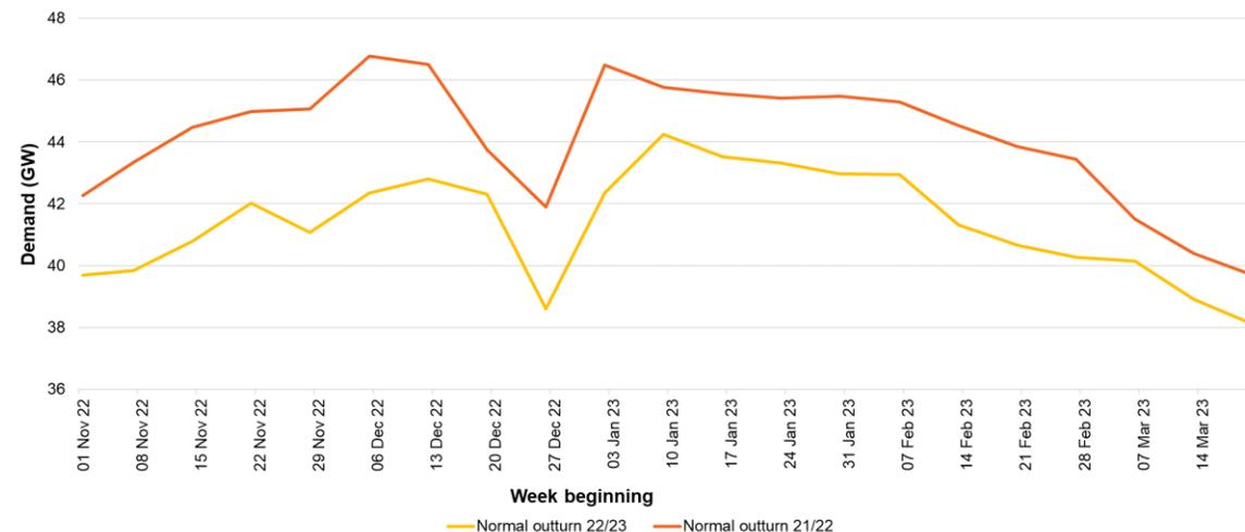
Figure 3: Peak Transmission System Demand (TSD) outturn (weather corrected) for winter 2022/23 compared to winter 2021/22.
