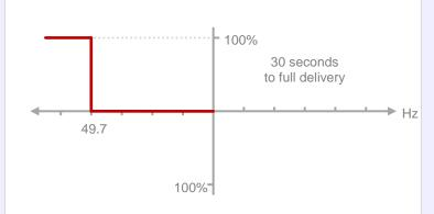
Recover frequency to 0.5Hz within 60 seconds following large losses
