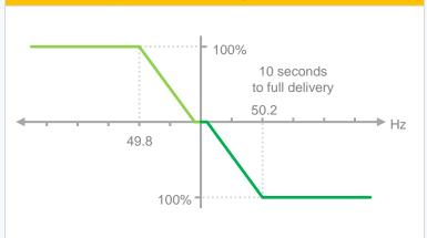
Assist in keeping frequency near to 50Hz during normal conditions
