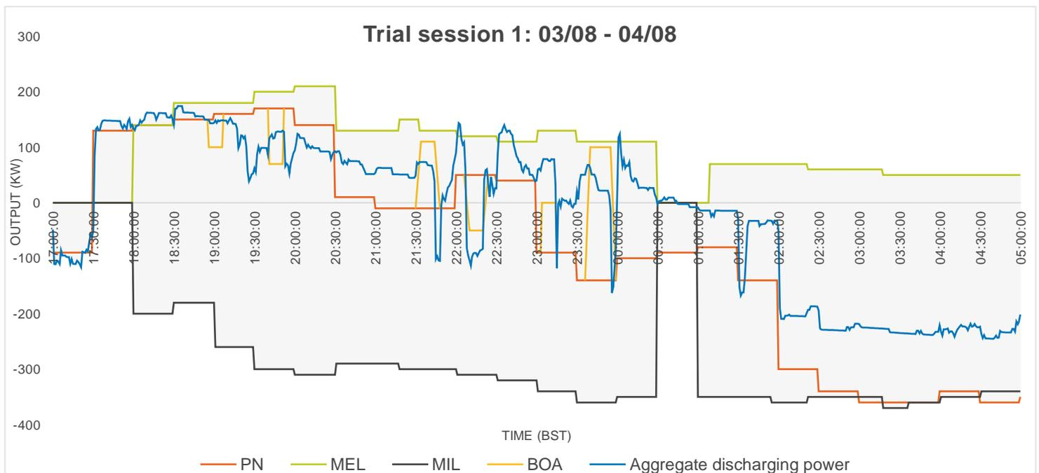
The shape is indicative of the typical activity we could expect to see from an aggregated unit made up of V2G enabled EVs. The highest aggregate discharging takes place from 17:30 to 19:00 when wholesale prices are
