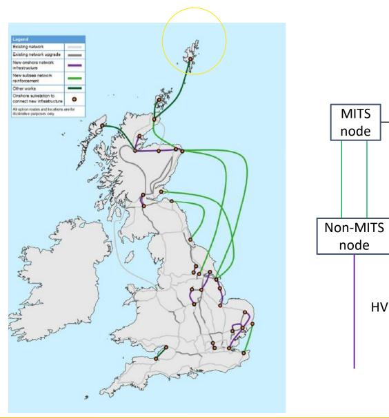
There are 132kV network on remote islands (for example, Shetland 132kV network). These 132kV assets will become part of the transmission network.
