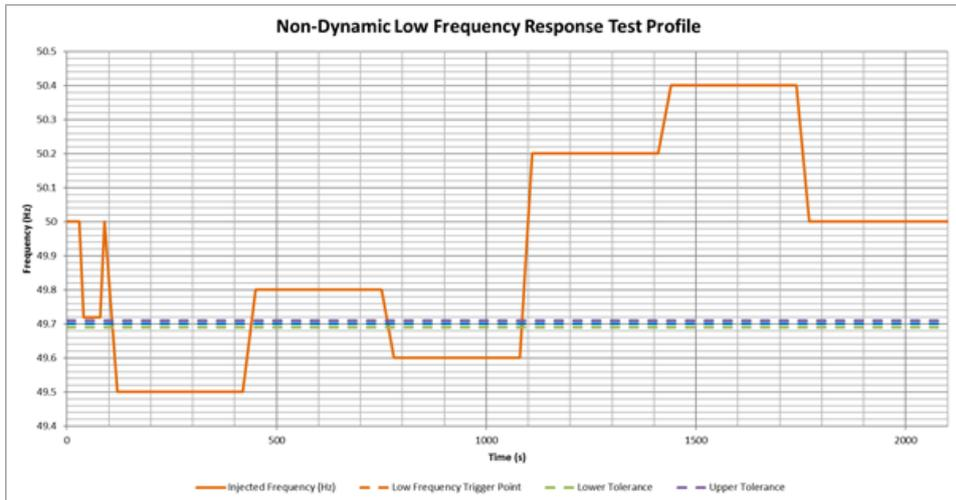
The initial frequency dip to 49.72Hz aims to prove that the relay will not activate (hence no response) if the frequency drops to just above 49.7Hz. During the sweep from 50Hz to 49.5Hz, the **Relay** should trigger at 49.7Hz ( $\pm 0.01$ Hz). Once the **Relay** has triggered, full response should be reached within 30 seconds and be sustained for a further 1770 seconds (30 minutes after relay trigger) regardless of the varying frequency injection.
