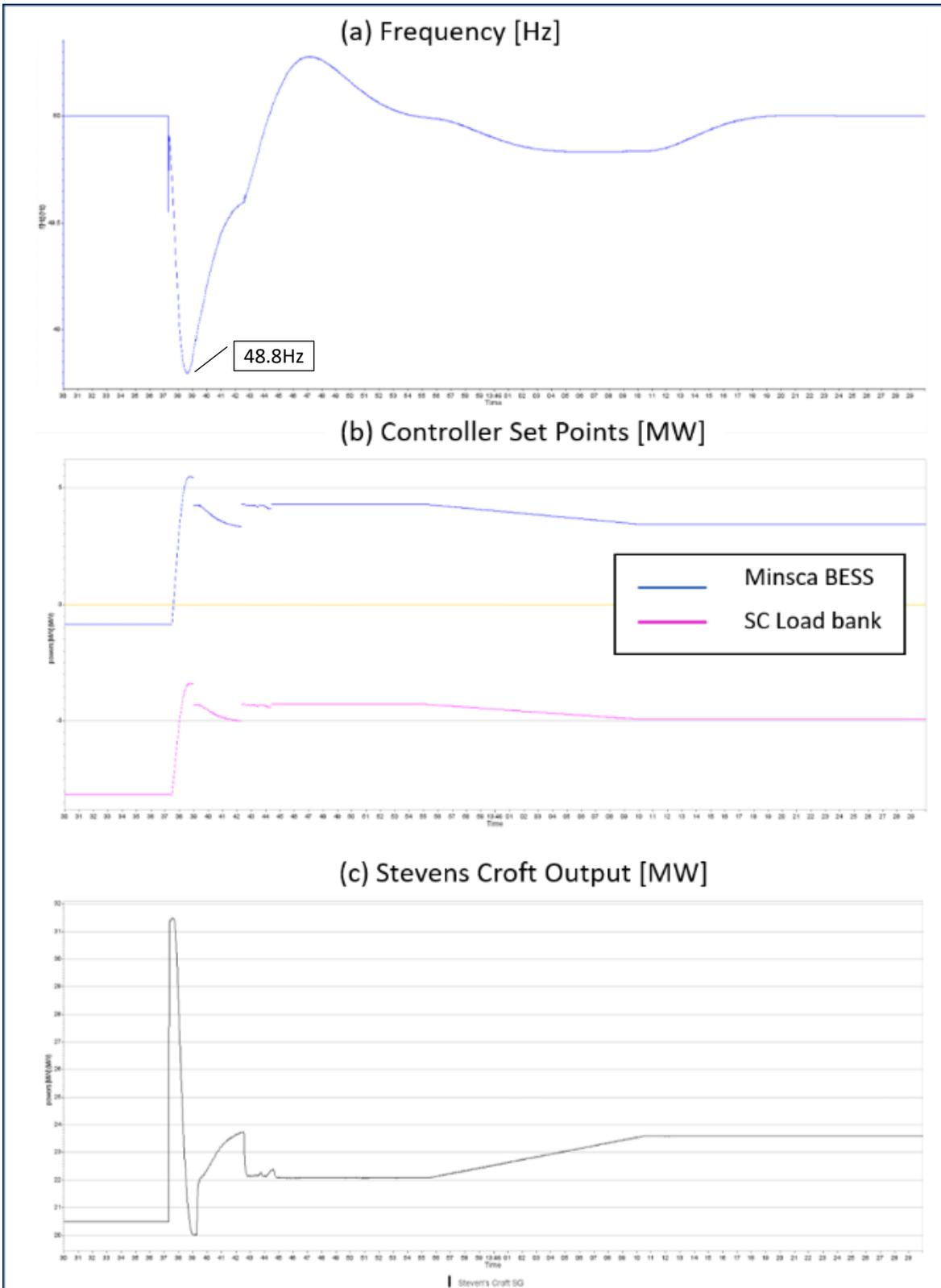
Figure 7 System response to a +10 MW load step (Delay Test Setup 2, 60 ms Delay, 1 min time axis)
