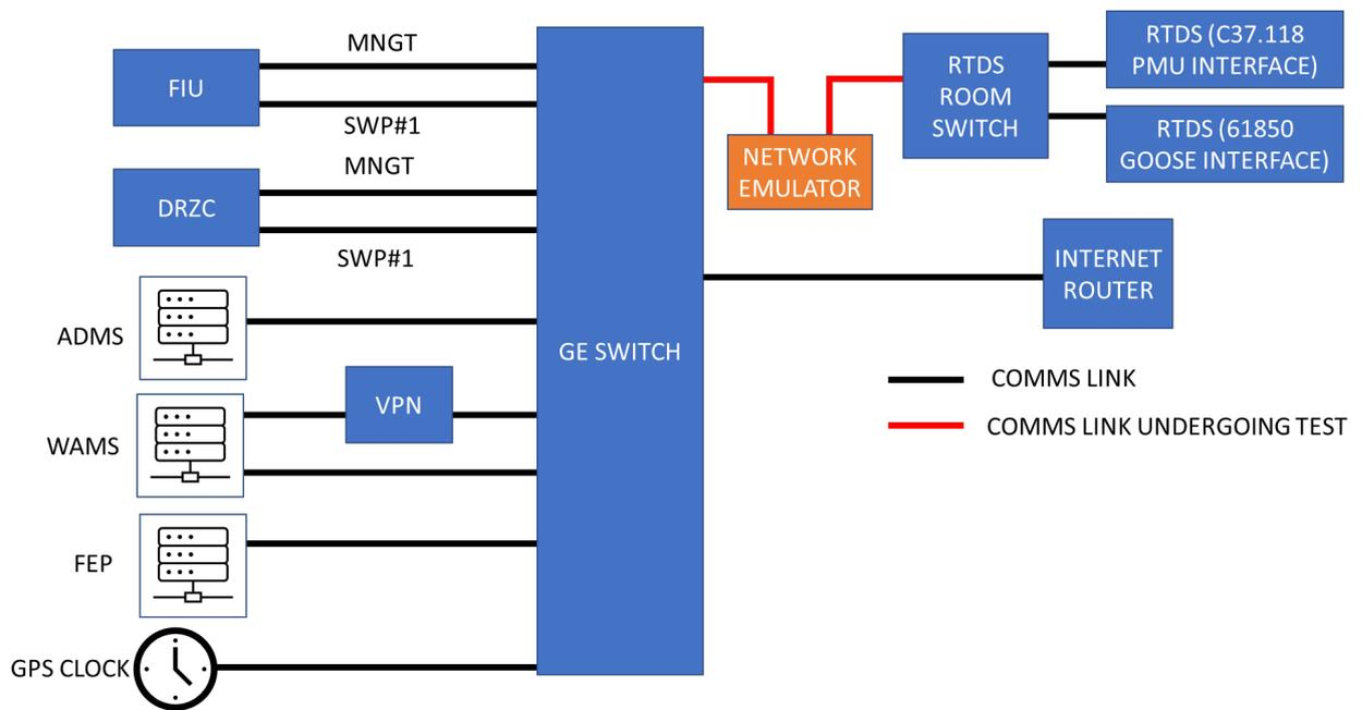
Figure 12 Network Emulator Test Position B (for Test 3)
