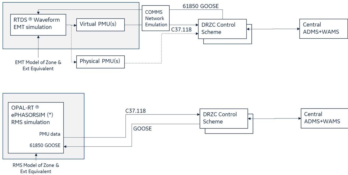
Figure 1 Examples of structure of Hardware-in-the-Loop test environments (Upper: RTDS; Lower: Opal-RT)
