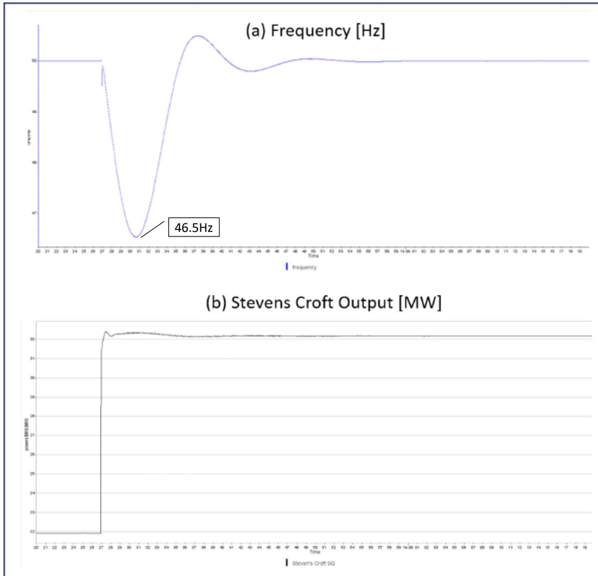
Figure 8 System response to a +10 MW load step (Delay Test Setup 2, 90 ms Delay, 1 min time axis)
