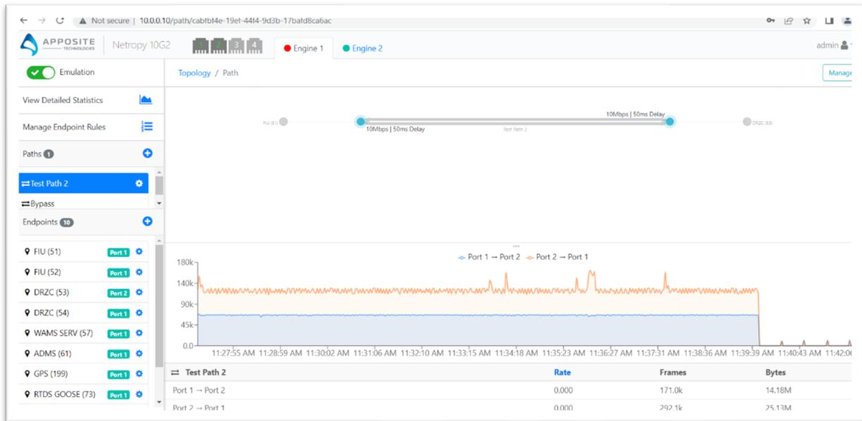
Figure 5 Network Emulator user interface screen, showing network traffic between FIU (Port 1) and DRZC (Port 2)
