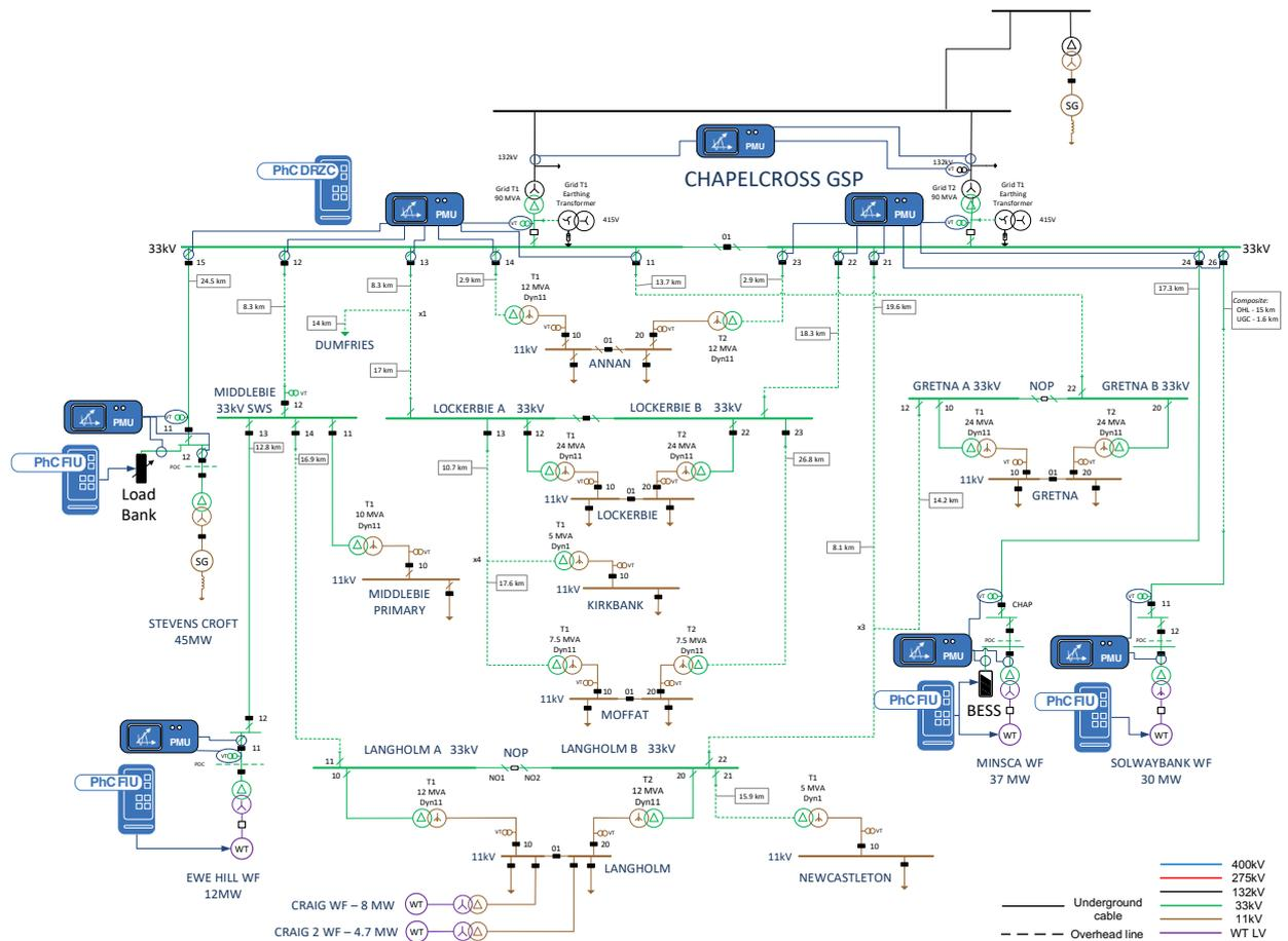
Figure 3 Chapelcross Distribution Network modelled for Distribution Restoration Zone Testing
