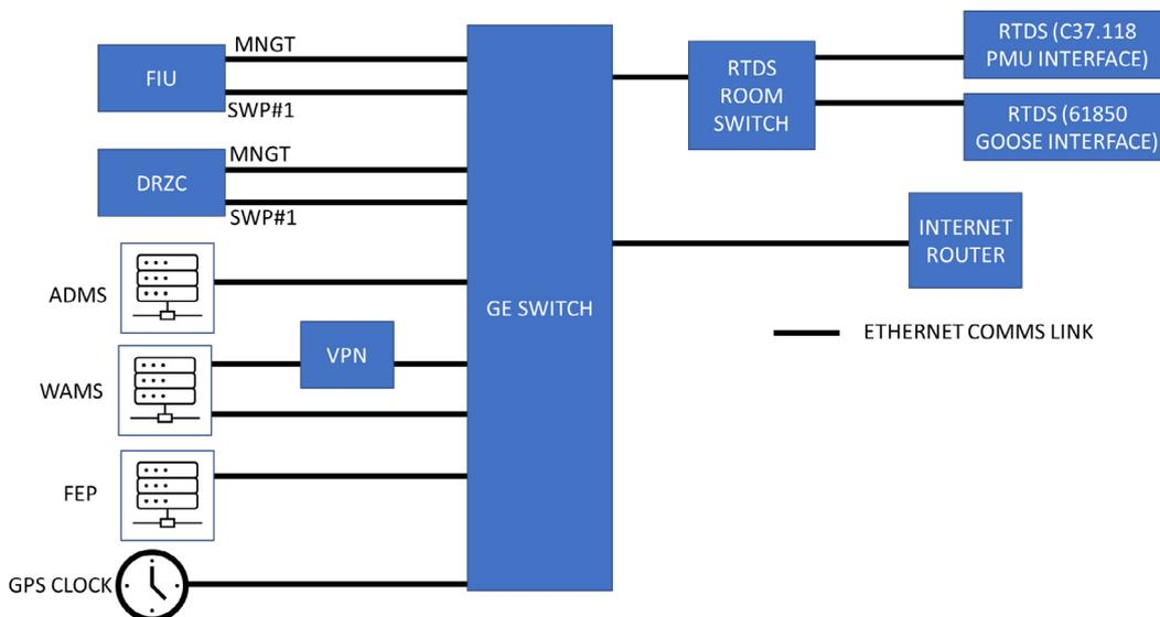
Figure 10 Communications Setup at the HVDC Centre
