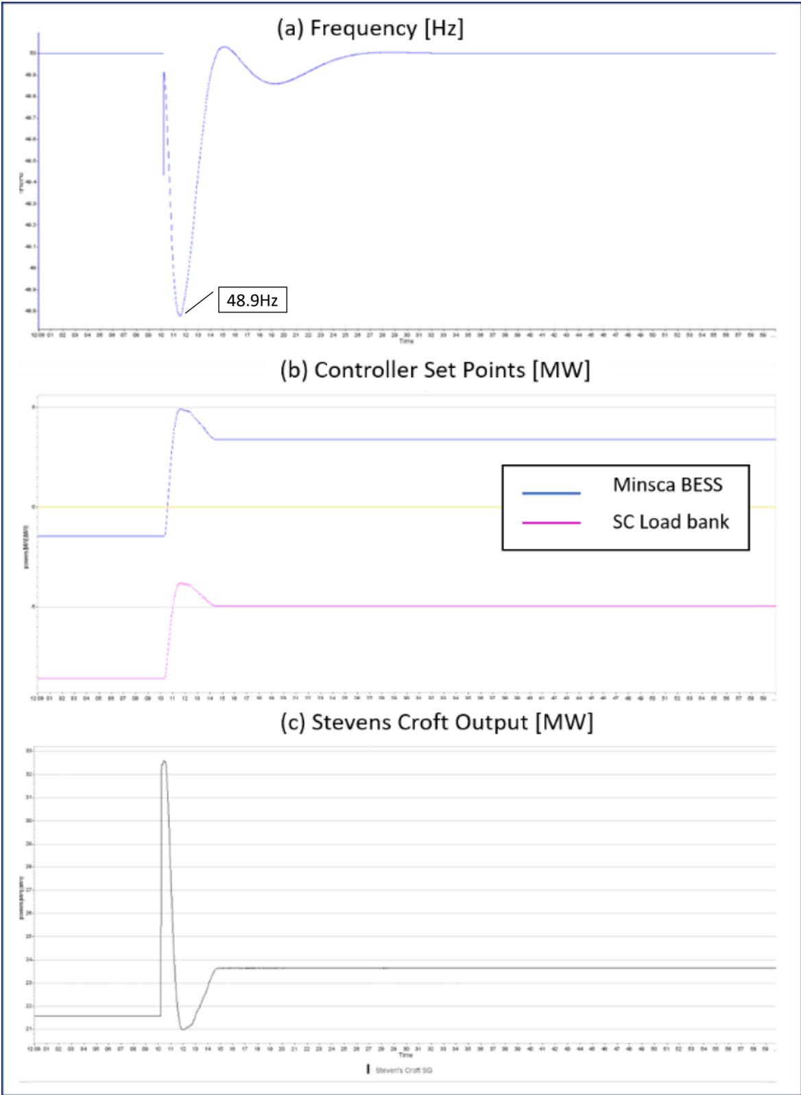
Figure 6 System response to a +10 MW load step (Delay Test Setup 2, 0 ms Delay, 1 min time axis)
