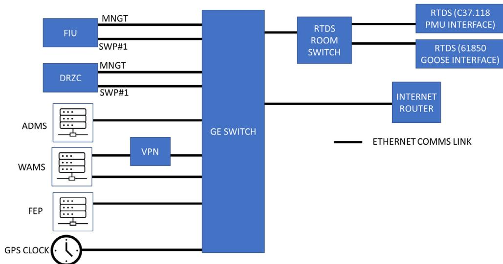
Figure 4 Communications/Network Setup at the HVDC Centre
