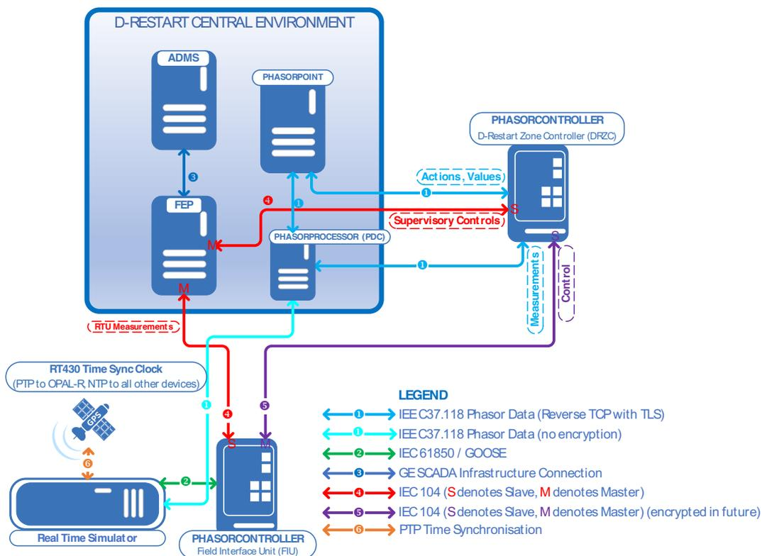
Figure 2 Test configuration for Hardware-in-the-Loop Testing
