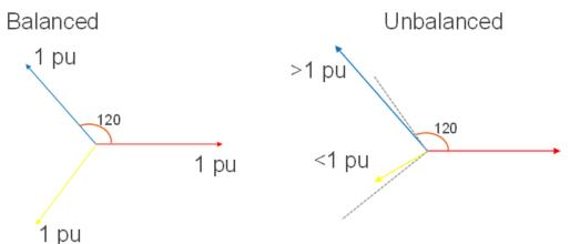
The main impact of NPS on system operation can be seen on the rotating electrical machines experiencing negative sequence torques. The predominant consequence is machine overheating and pulsating torque which reduces life expectancy of the machine. The Grid Code limits and Engineering Recommendation planning levels take into account the long term impact on the machines while allowing for suitable protection settings for the machines.
