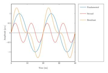
(a) Basic illustration example with one harmonic frequency imposed
