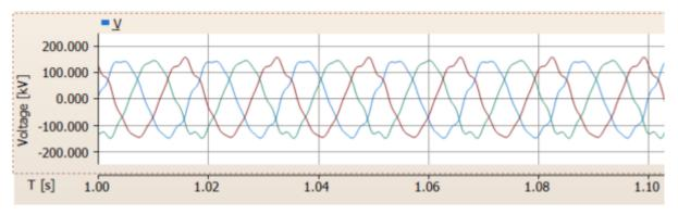
(b) Realistic example of 3 phase voltages with harmonic distortion
