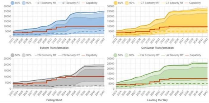
With increasing generation and potential interconnectors in the SSEN Transmission area for all scenarios, the required transfer across boundary B4 is expected to increase significantly over the ETYS period. The prospective generation behind boundary B4 includes around 2.7GW from Rounds 1-3 and Scottish territorial waters offshore wind located off the coast of Scotland.
