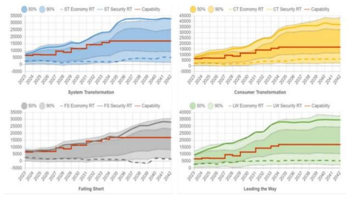
Across all FES, there is an increase in the power transfer requirements from Scotland to England due to the connection of additional generation in Scotland, primarily onshore and offshore wind.
