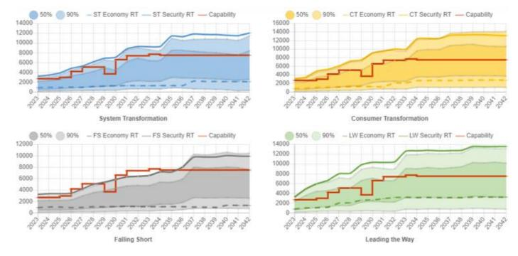
New renewable generation connections north of the boundary are expected to result in a significant increase in export requirements across the boundary, especially along the Beauly - Denny circuit. All generation north of boundary B0 also lies behind boundary B1a.
