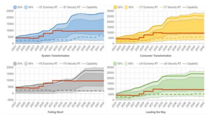
The capability line (in red) is based on the recommendations from the NOA 2021/22 optimal path which uses the 2021 FES and ETYS data as inputs. The 50%, 90% Economy RT and Security RT lines are based on FES 2022. The ETYS and NOA methodologies for this boundary are different and can result in different transfer capabilities.
