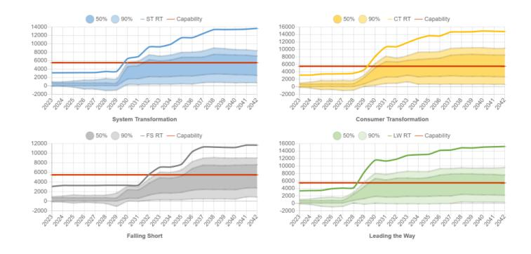
The capability line (in red) is based on the ETYS transfer capability using FES 2022 data, described below. The 50%, 90% Economy RT and Security RT lines are based on FES 2022.
