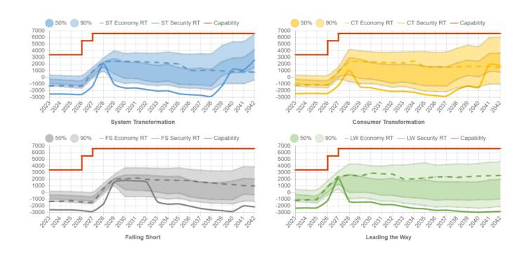
It can be seen that until new generation or interconnectors connect there is very little variation in boundary requirements, and that the current importing boundary capability is sufficient to meet the short-term needs.
