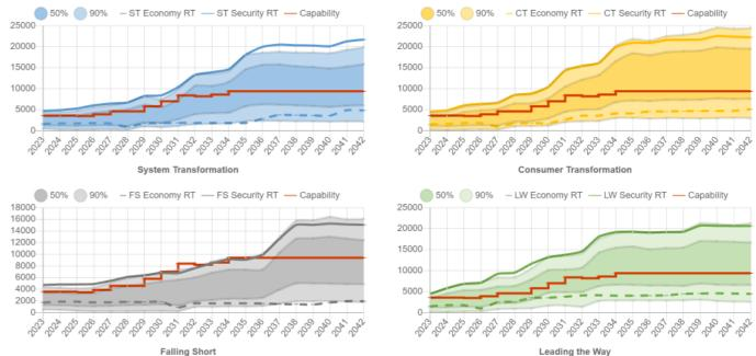
The potential future boundary transfers for boundary B2 are increasing at a significant rate because of the high volume of renewable generation to be connected to the north of the boundary. This increased generation capacity will drive increasing power flows down the east coast 275kV circuits.
