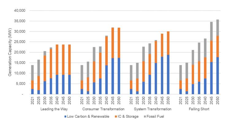
In a highly decentralised scenario like Leading the Way, local generation capacity connected at the distribution level in this region could reach over 15GW by 2030. Of that capacity, a typical embedded generation output on average might be around 4GW. The South is expected to fulfil a smaller portion of its demand from local embedded generation than other regions are.
