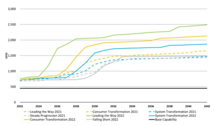
The percentile power flows are not determined for the B3b boundary. The capability line (in black) is based on the ETYS transfer capability using FES 2022 data, shown below.
