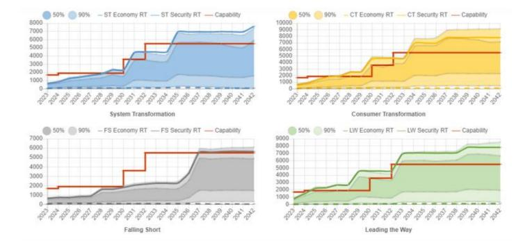
The power transfer through B0 is increasing due to the substantial growth of renewable generation north of the boundary. This generation is primarily centred around both onshore and offshore wind. There is also the prospect of new marine generation resource in the Pentland Firth and Orkney waters in the longer term.
