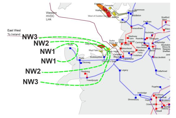
Currently, there is not a significant amount of generation behind NW2, mainly Dinorwig pumped storage and offshore wind projects connecting to Bodelwyddan. The expected transfers only see significant changes from around 2029 onward when they increase very sharply as large new offshore wind projects come online and an intra GB DC link connecting to Scotland lands at Pentir. This will mean that in future transfers across the NW2 boundary will be heavily dependent on wind conditions.
