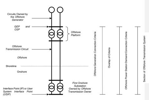
Figure 1.2 An offshore transmission system with a directly connected power station and first onshore substation owned by the offshore transmission owner
