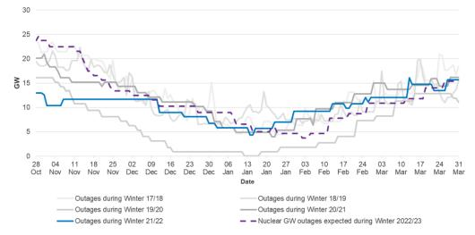
Figure 14. The impact on French nuclear capacity from planned outages in 2022/23 and actual outages in recent years<sup>3</sup>
