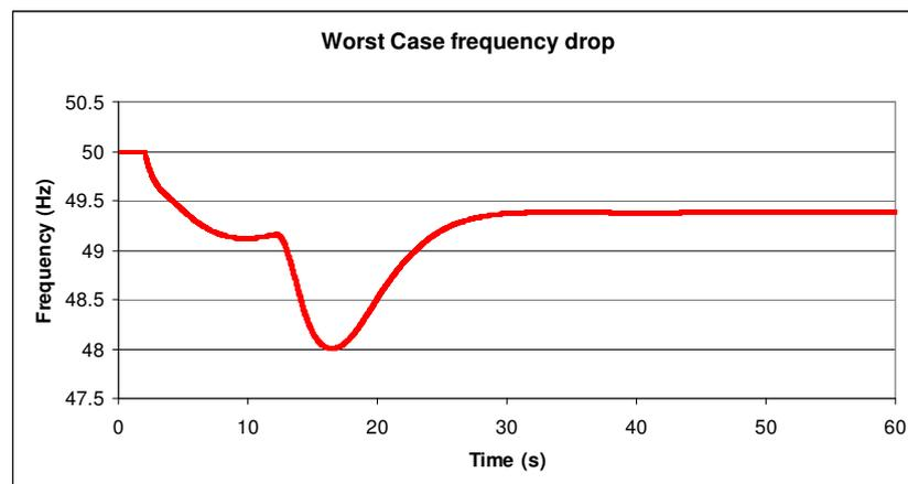
Figure 6.0A – Effect on System Frequency as a result of the Recovery Period at Critical Wind Speeds
