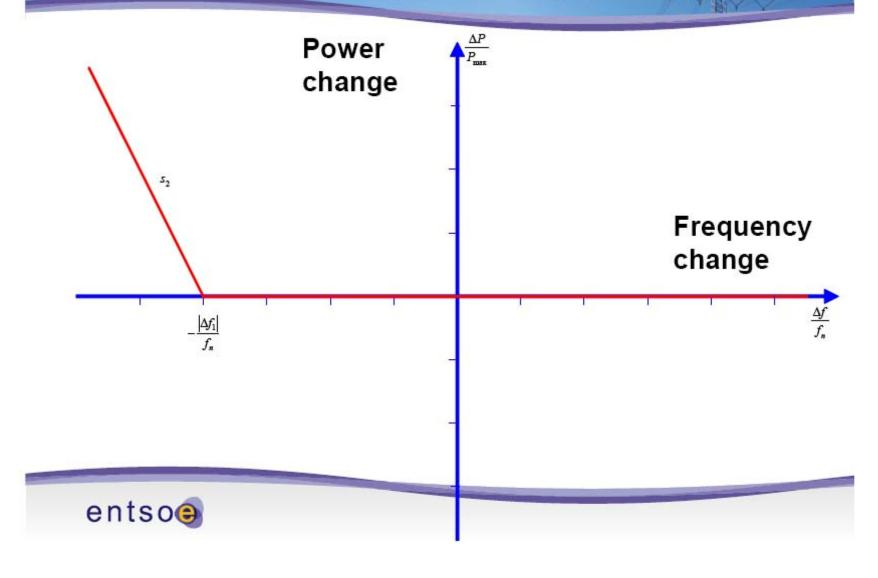
FSM The relationship between the relative change in frequency ( $\Delta$  f/fn) and the required response in terms of relative power change ( $\Delta$ P/Pmax)
