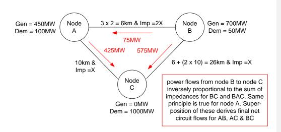
Nodes A and B export, whilst Node C imports. Hence the DCLF algorithm derives flows to deliver export power from Nodes A and B to meet import needs at Node C.
