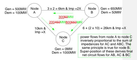
Node B exports, whilst Nodes A and C import. Hence the DCLF algorithm derives flows to deliver export power from Node B to meet import needs at Nodes A and C.
