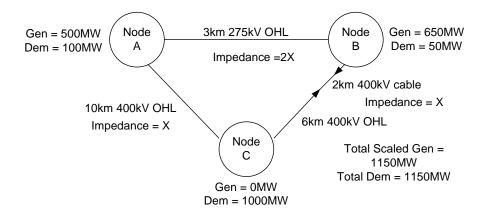
Assuming Node A is the reference node , each 400kV circuit has impedance X, the 275kV circuit has impedance 2X, the 400kV cable circuit expansion factor is 10 and the 275kV overhead line circuit expansion factor is 2, the DCLF transport algorithm calculates the base case power flows for Peak Security background as follows:
