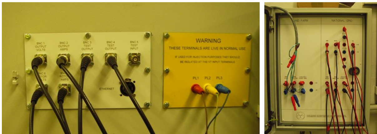
Figure 1: Example of Compliance Test Signal Connections
