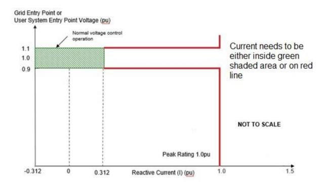
Figure 6 showing an interpretation of the existing legal text requiring the current to either be in the green box or on the red line
