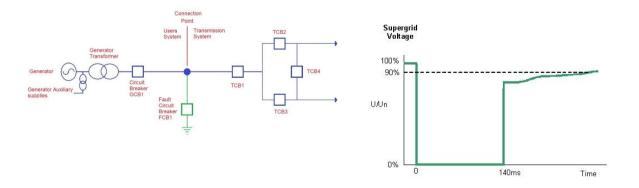
Figure showing theoretical worse case fault which plant has to be capable of riding though
