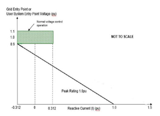
Figure 7 showing the proposed reactive current injection requirements, requiring the current to always remain above the black line
