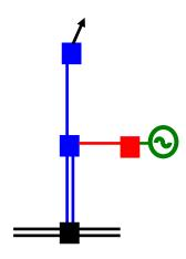
This example shows a radial circuit that facilitates both generation and demand. The separate demand and generation substations connect via to a substation via a single circuit which in turn connects to a single MITS substation via a double circuit. In this scenario the generation substation and the single circuit connecting to the intermediatary substation form a radial spur used only for connecting generation to the MITS.
