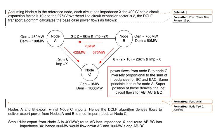
Step 2:Net export from Node B is 600MW; route BC has impedance X and route BA-AC has impedance 3X; hence 450MW would flow down BC and 150MW along BA-AC
