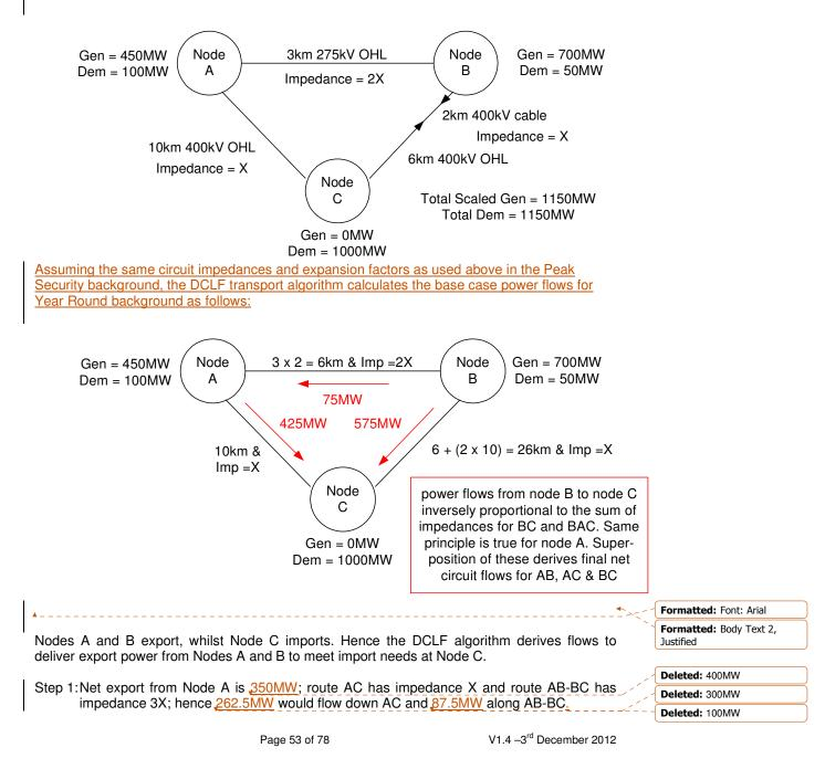
Step 2:Net export from Node B is <u>650MW</u>; route BC has impedance X and route BA-AC has impedance 3X; hence <u>487.5MW</u> would flow down BC and <u>162.5MW</u> along BA-AC
