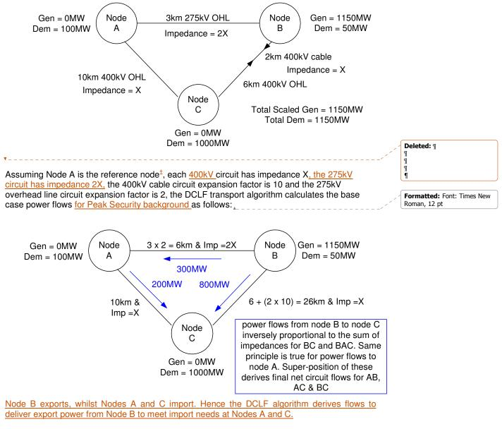
Step 1:Net export from Node B to Node A is 100MW; both routes BA and BC-CA have impedance 2X; hence 50MW would flow down both routes.
