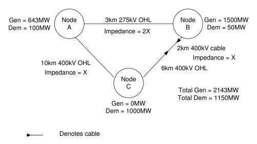
The first step is to match total demand and total generation by scaling uniformly the nodal generation down such that total system generation equals total system demand.
