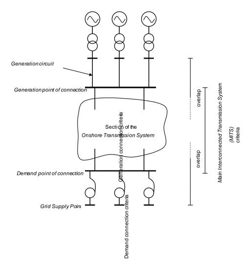
Figure 1.1 The *onshore transmission system* with a directly connected *power* station
