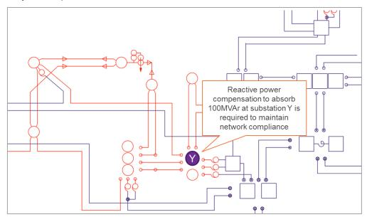
Next, the ESO calculates the effectiveness for options connecting at substation Z with substation Y as the reference point. The ESO models reactive power compensation to absorb 100MVAr at substation Z and tests it under selected backgrounds and conditions. In this example, analysis results show that (on average) implementing reactive power compensation to absorb 100MVAr at substation Z reduces the compensation required at substation Y from 100MVAr to 25MVAr.
