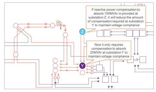
The ESO can then approximate the effectiveness for any options connecting at substation Z as (100-25)/100 = 0.75 with respect to the reference point.
