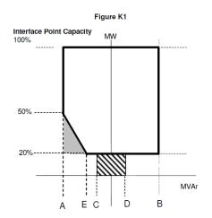
**Point A** is equivalent (in MVAr) to 0.95 leading Power Factor at active power transfer equal to the Interface Point Capacity.
