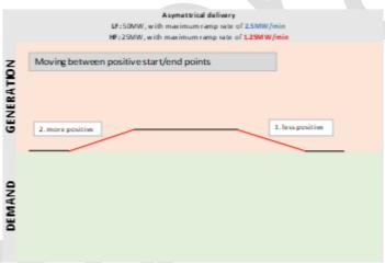
In the **second** example the ramp rates are calculated from the quantity of LF. The specific baseline change illustrated is typical of a unit managing its SoE due to delivery of LF (i.e. it needs to charge/demand to increase its stored energy after responding to low frequency).
