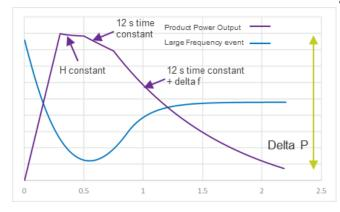
Swing equation relationship to determine additional active power to allow df/dt of upto 1 Hz/s
