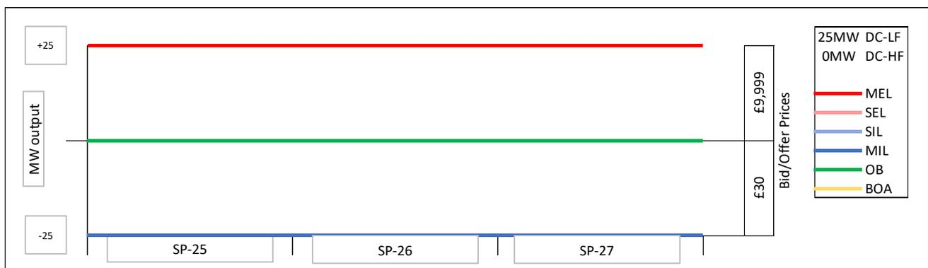
The ESO issues a short (<15 min) BOA bid from (PN to MIL) to the unit which is accepted. Following BOA acceptance, the BMU re-declares its MIL in-line with the principles described in the section above. The MIL is re-declared at a point at least 15+2 minutes after the point of instruction.
