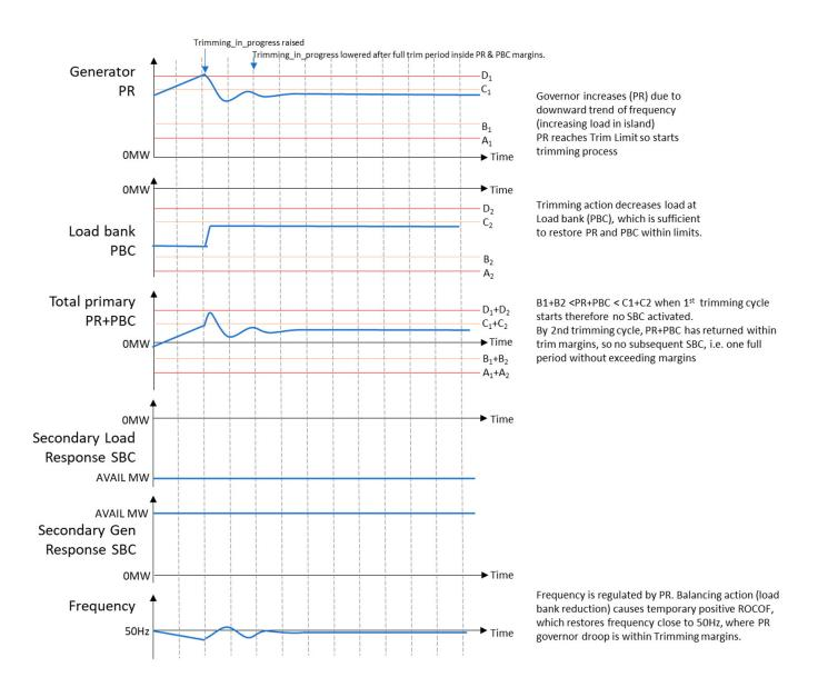
Figure 8: Generator PR at D<sub>1</sub> trim limit +  $\rightarrow$  PBC response
