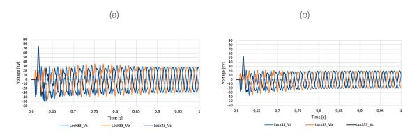
Figure 46: Instantaneous phase voltages at Lockerbie 33kV busbar for (a) 1pu and (b) 0.7pu energisation voltage
