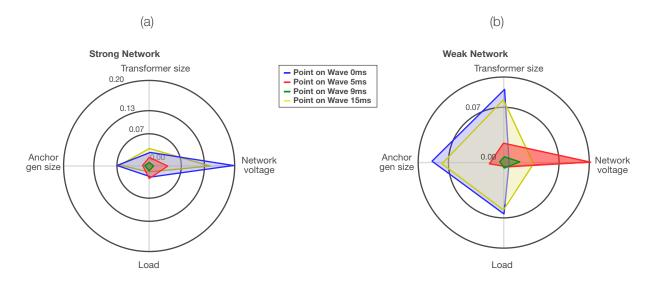
Figure 37: Quantitative influence of parameters on system voltage dip
