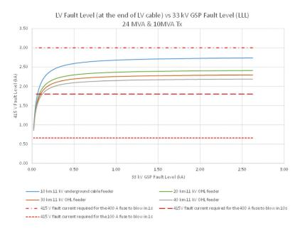
Figure 34: LV Fault level (at end of 400m LV cable) for four feeder options vs 33kV GSP fault level (LLL) for a 24MVA primary transformer; the 415V fault current for a 400A and 100A fuse to blow in 1s are shown
