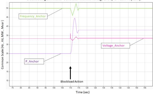
Blockloading on Anchor Generator without Voltage Droop or Fast Frequency.
