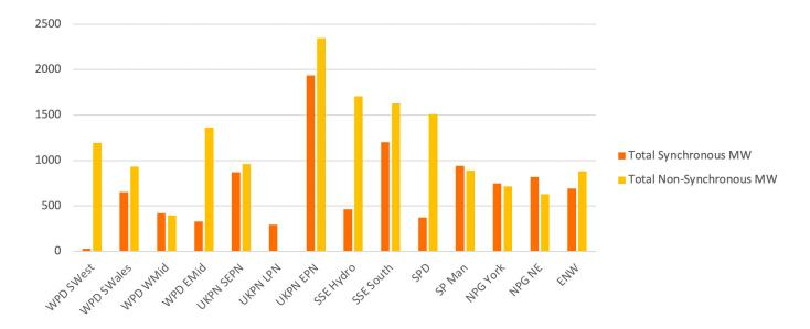
Figure 25: Amount of presently connected synchronous generation (orange), and non-synchronous generation (yellow) per DNO area
