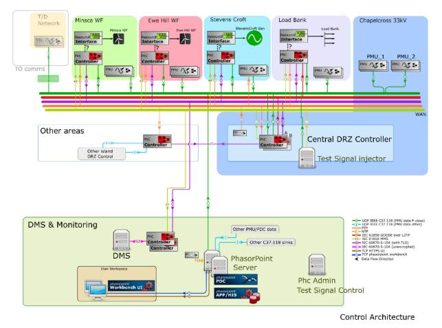
Figure 17: High level DRZ-C solution design including key components, links and communications protocols
