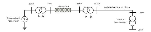
Figure 38: Schematic of the network used for the Ecclefechan energisation study
