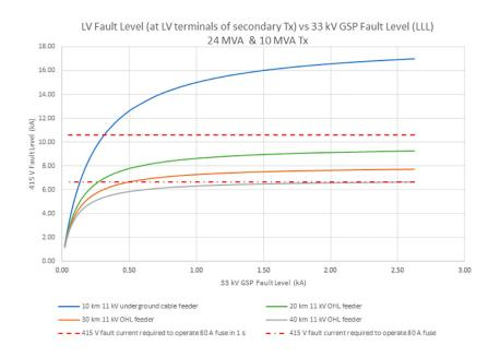
Figure 33: Fault level (at LV terminals of secondary Tx) for four 11kV feeder options vs 33kV GSP fault level (LLL) for a 24MVA primary transformer
