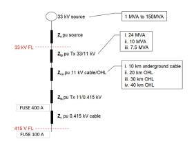
Figure 30: Simplified single line diagram of the network under consideration
