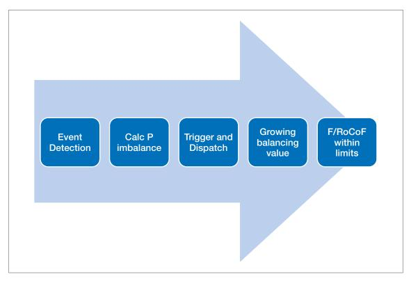
Figure 2: Fast balancing process
