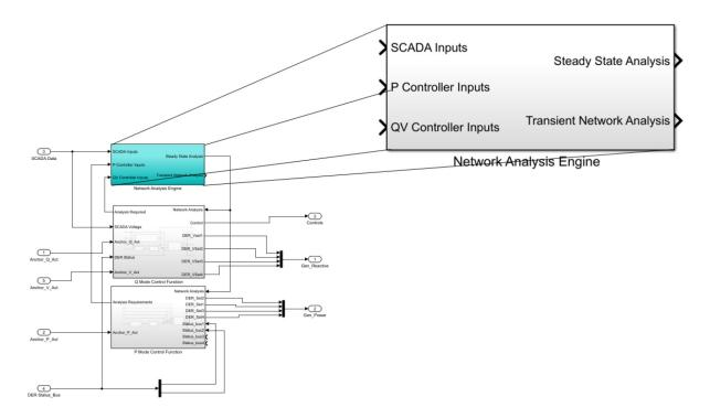
Figure 21: Block diagram showing inputs and outputs to network analysis engine
