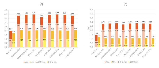
Figure 40: Impact of energisation voltage on the TOV, (a) energisation at 1pu, (b) energisation at 0.7pu
