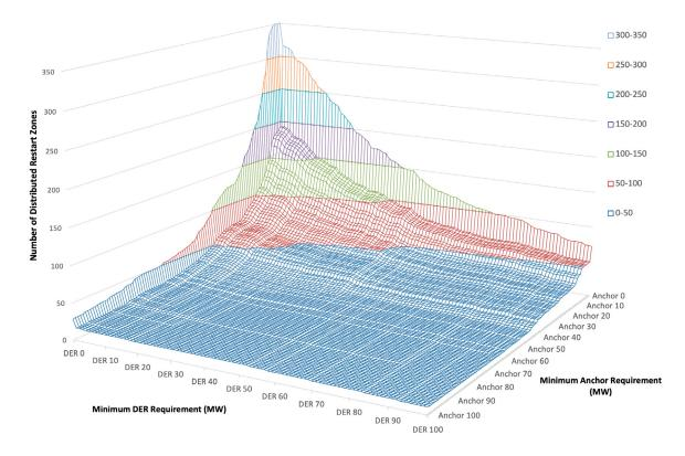
Figure 28: Number of DRZs as related into increasing anchor and DER requirements (does not Include network in and around London)
