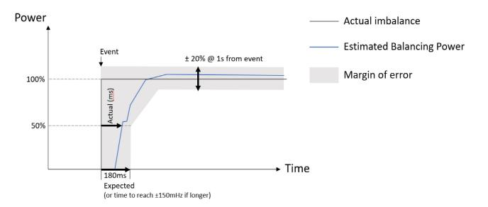
Figure 4: Load bank power response based on measured RoCoF during an event (continuous response provided up to maximum RoCoF). Response should settle within some defined margin of actual imbalance
