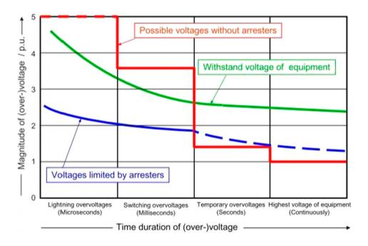
Figure 35: Temporary overvoltage vs withstand voltage of equipment<sup>14</sup>
