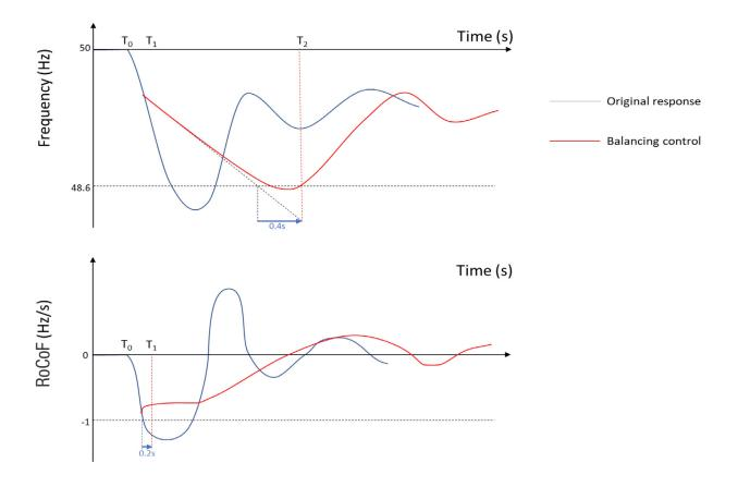
Figure 3: Qualitative illustration of the effect of fast balancing on frequency and RoCoF
