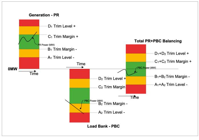
Figure 7: Trim levels and margins for slow island balancing process
