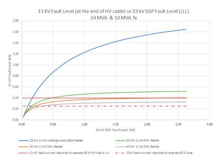
Figure 32: 11kVFault level (at end of feeder circuit) vs 33kV source fault level (LLL) for a 24MVA primary transformer
