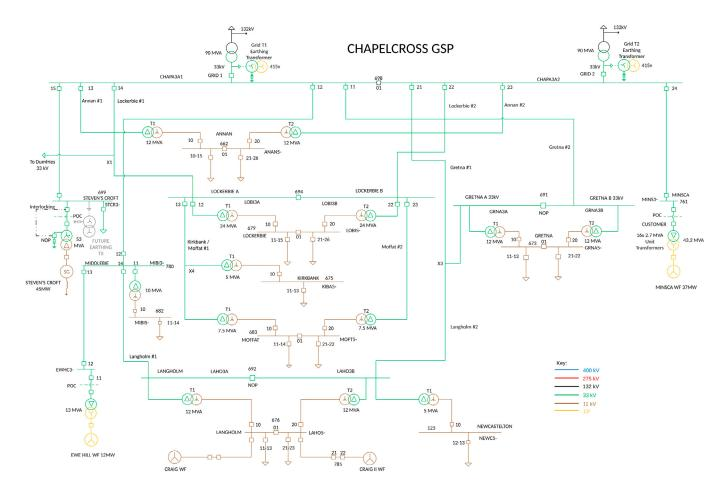
Figure 45: Chapelcross GSP case study network single line diagram
