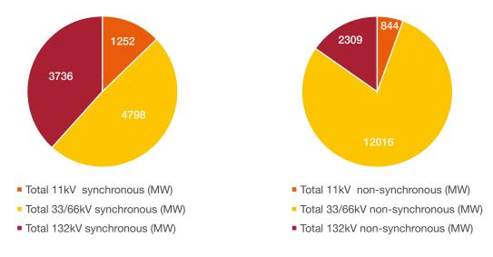
Figure 26: Synchronous DER and non-synchronous DER MW split by connected voltage
