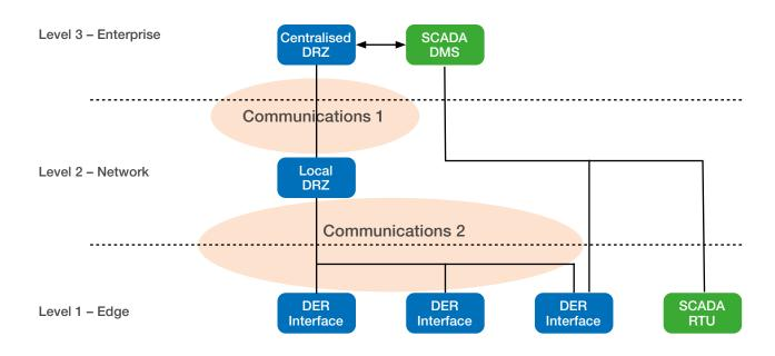
Figure 20: DRZ-C hybrid deployment
