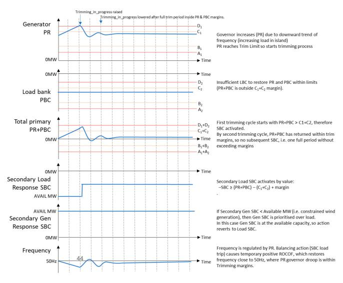
Figure 9: Generator PR at D1 trim limit+ → SBC response
