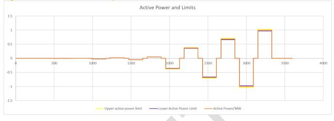
Figure 2 – Test 1 Active Power Response
