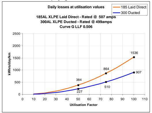
This graph shows the effect of using a larger cable in a duct to obtain a similar circuit rating.
