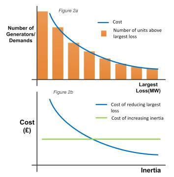
When the system sees an imbalance in generation and demand, the system frequency changes. System inertia directly links with the Rate of Change of Frequency (RoCoF) for any sudden change in generation and demand.
